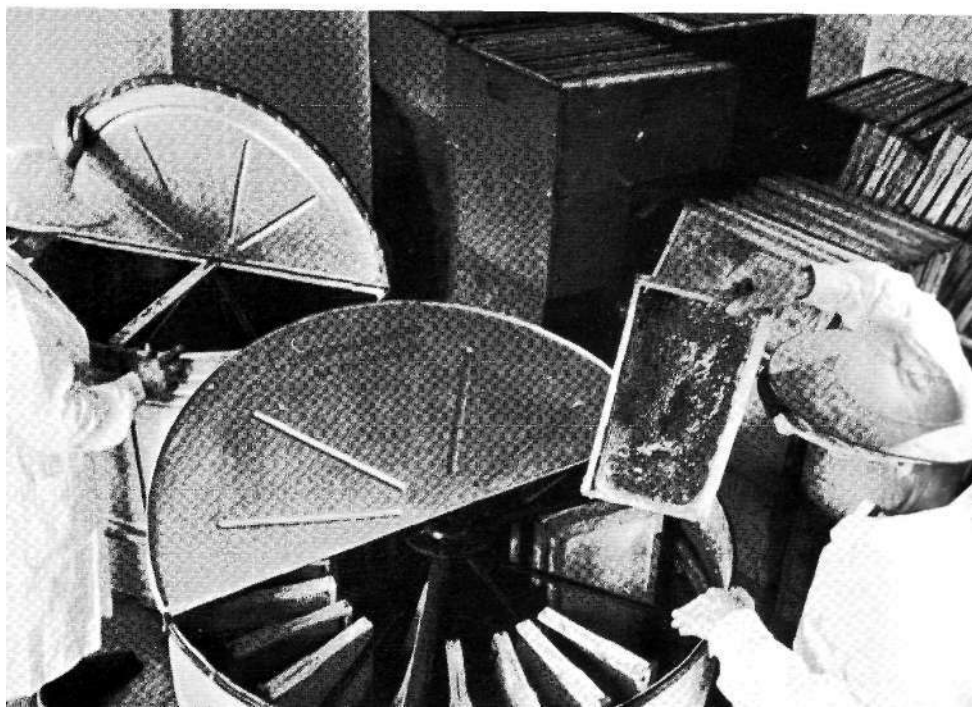
Left A small tangential extractor suitable for a beekeeper with two or three hives. Below A motorized radial extractor being filled with frames.
