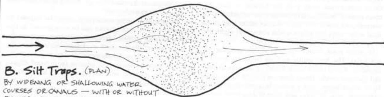
**B. Silt Traps.** (PLAN)
