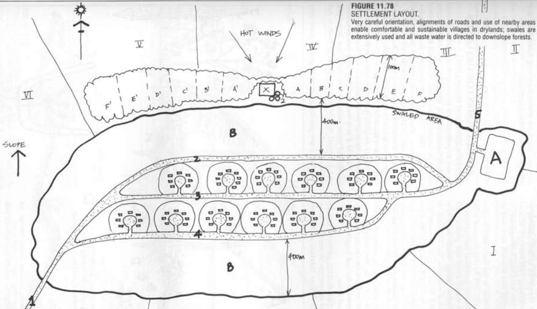
**A-F and A'-F:** Sewage or swale-fed fuel forests on 6-year rotations, surrounded by belts of perpetual forests. Gravity flow of sewage or swale/diversion water to this site.
