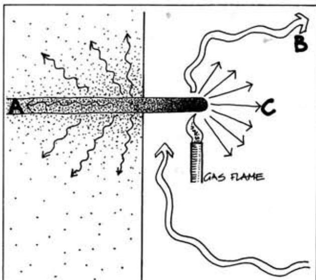
**A HEATED BAR EMBEDDED IN CONCRETE DEMONSTRATES HOW HEAT DIFFUSES TO COLDER AREAS.**
