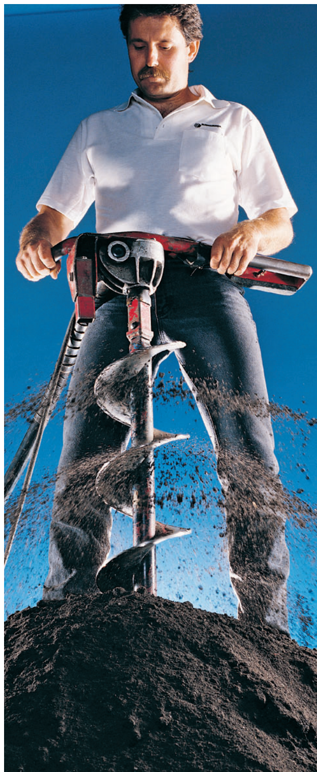
Power augers quickly dig holes for post footings. They are available at rental centers. Some models can be operated by one person, while others require two people.
