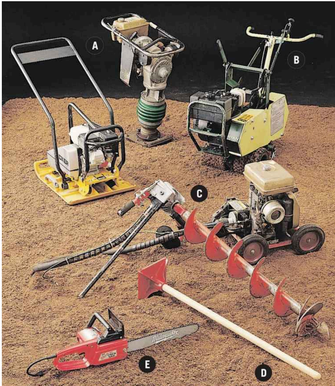
Specialty tools include: tamping machines (A), sod cutter (B), power auger (C), hand tamper (D), chainsaw (E).
