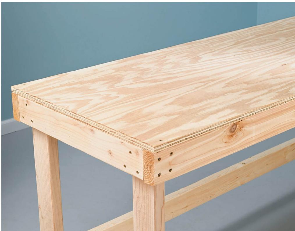
**Exterior plywood** offers a smooth, continuous surface for a bench top or shelf. One full 4 × 8' sheet of  $\frac{3}{4}$ "-thick plywood will cover a full-size bench top and shelf. Fasten plywood to the frame parts with  $1\frac{1}{2}$ " deck screws. Keep in mind that a plywood surface won't drain like a permeable material; you may want to pitch the bench slightly to one side for drainage. Coat it with deck stain or paint to make it easier to clean and more stain resistant.
