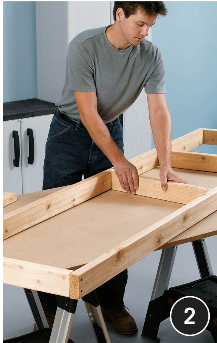
**Install the top supports** between the side pieces, spacing them 24" apart on center. First, mark layout lines onto both side pieces, then square the frame by measuring diagonally between opposing corners; the frame is square when the measurements are equal. Fasten the supports with pairs of 3½" deck screws.
