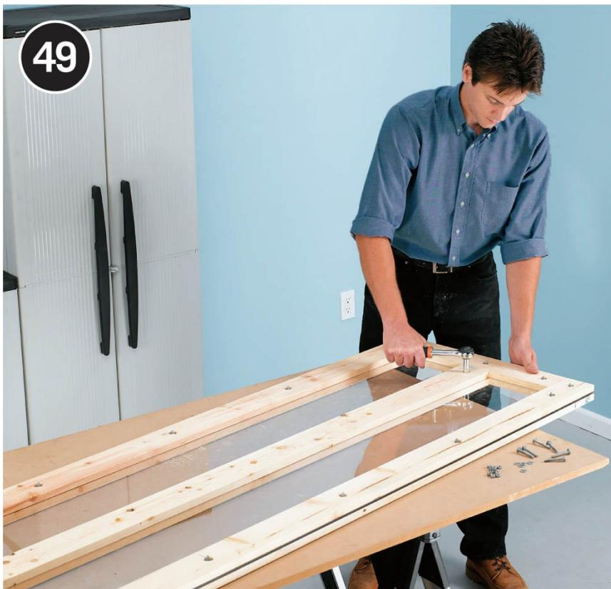
**Bolt the door together** in the same manner as the window, drilling over-sized guide holes and counterboring slightly for the nuts. Install two or three bolts in the center stile area to keep the frame and glazing from separating.
