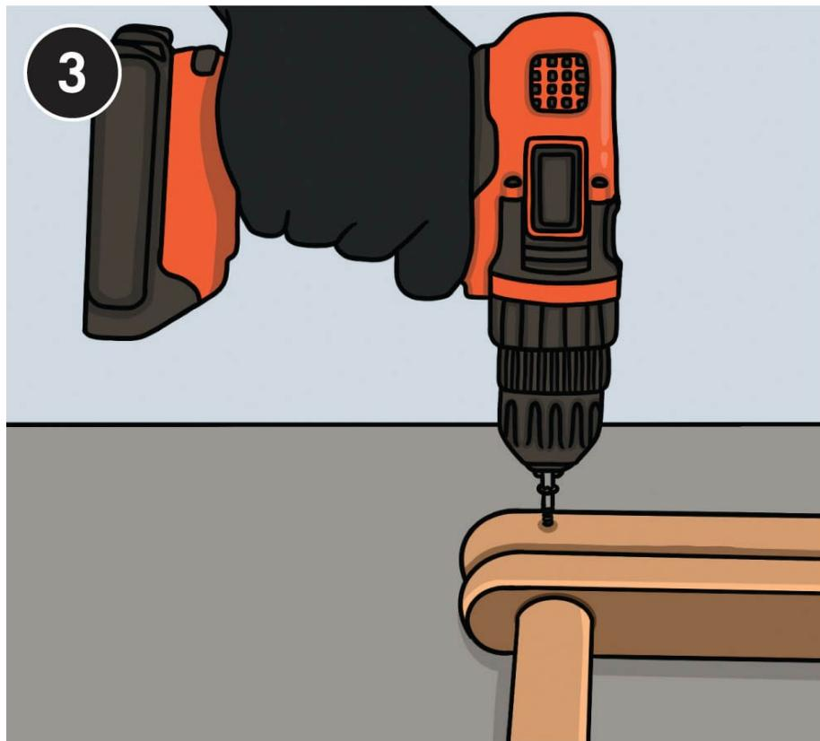
**Measure and mark** 1" from the end of the outside board of the leg pair. Drill a pilot hole, and then screw the outer leg to the dowel with a #4 x 2" screw. Repeat with the opposite leg pair.
