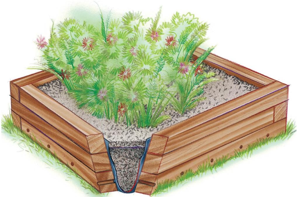
**This basic but very sturdy raised bed** is made with  $4 \times 4$  landscape timbers stacked with their ends staggered in classic log-cabin style. The corners are pinned together with 6" galvanized spikes (or you can use timber screws). It is lined with landscape fabric and includes several weep holes in the bottom course for drainage. Consider adding a  $2 \times 8$  ledge on the top row. Corner finials improve the appearance and provide hose guides to protect the plants in the bed.
