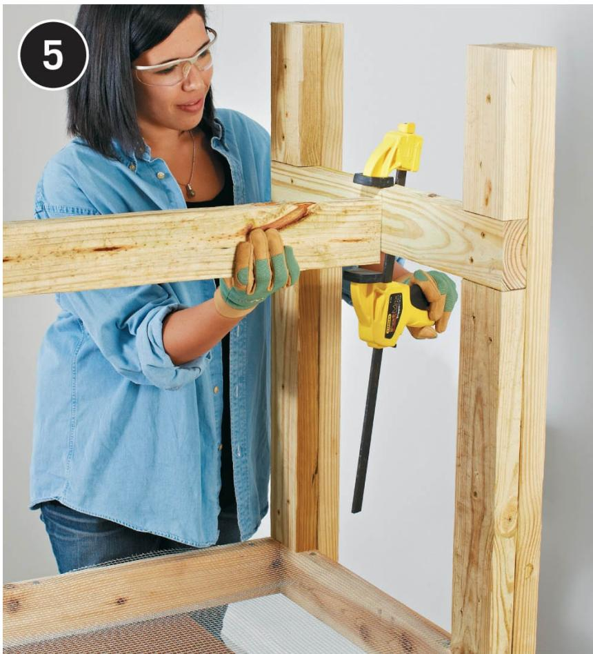
**Attach the stretcher with  $2\frac{1}{2}$ " screws.** Use clamps to hold the wood in place while you predrill and fasten. Also measure and cut the bottoms of the legs, and fasten with adhesive and screws.
