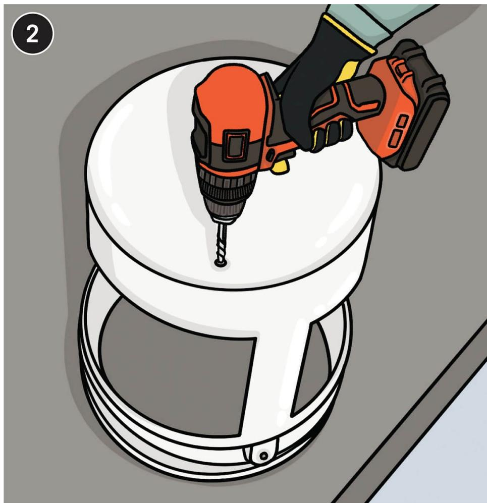
**Drill an access hole** and use a jigsaw to cut out the two windows, leaving the spines and bottom section. Drill a random pattern of  $5/64$ " drainage holes in the bottom of the bucket.
