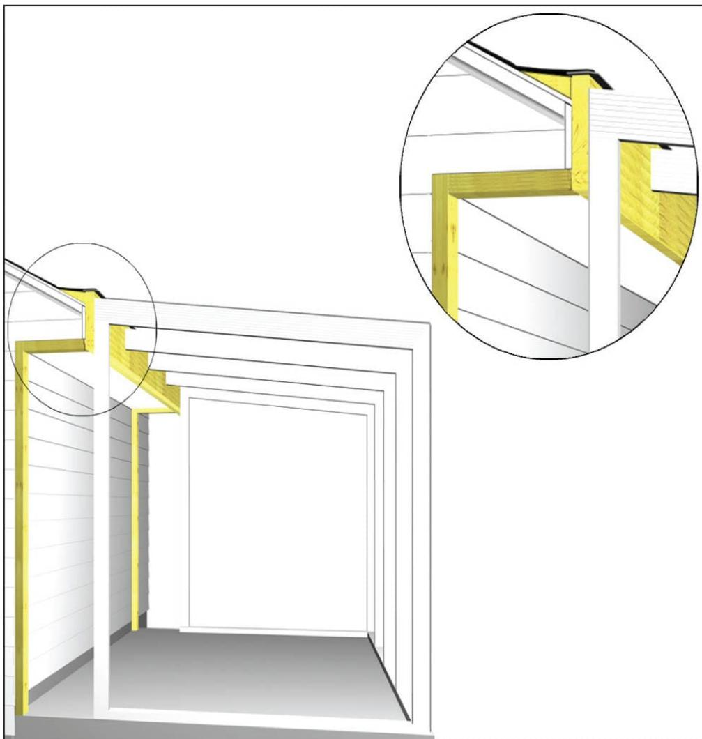
**If the sunroom is slightly taller than the roof eaves,** you can add a ledger that's taller than the fascia, but it cannot extend more than a couple of inches higher. Fill in the open area beneath the roof covering created at the side using a full-width wood wedge and caulk. The roof covering must retain a slight slope with no swales.
