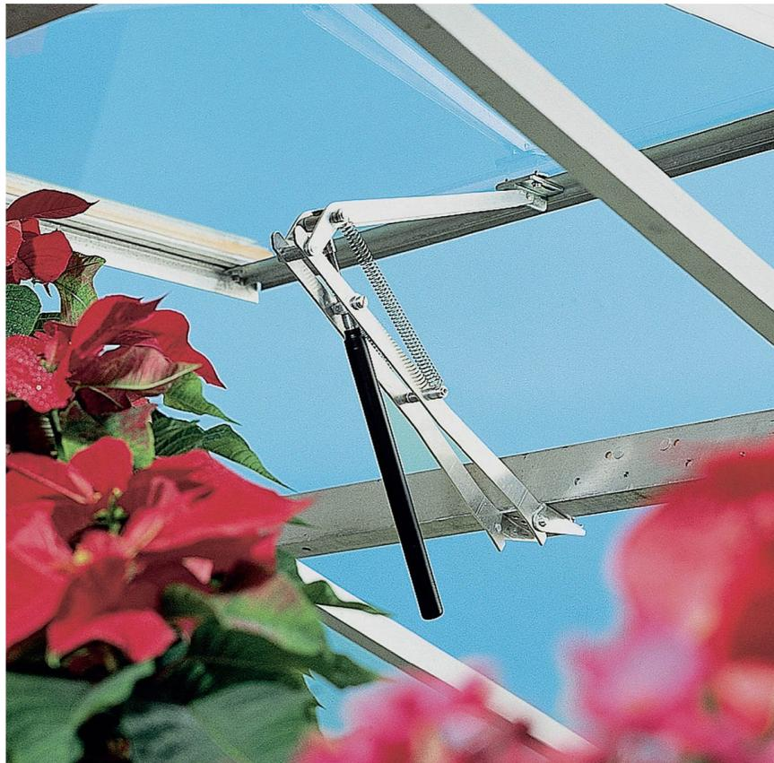
**Pick accessories** to make greenhouse gardening easy on yourself. The solar-powered automatic openers shown here make opening and closing vents and louvers one less thing you need to worry about. As the black probes are heated by increasing sunshine, they slowly trigger the opening devices, working in reverse when the sun goes down.
