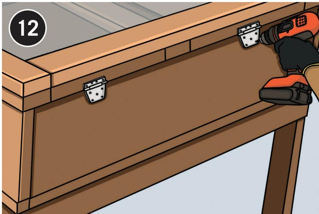
**Place the lid on top** of the box as it will rest when closed. Measure, position, and mark the hinge screw holes. Screw the hinges to the box and the lid edge.
