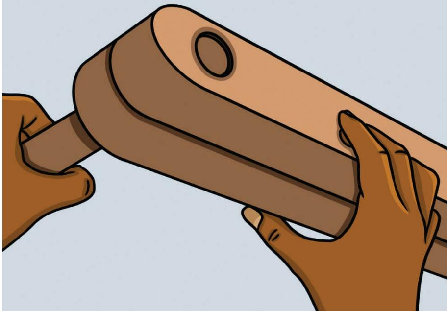
**Set two of the legs on edge**, flush to one another, side by side on a flat, level work surface. Align the holes in the ends of each leg. Slide the end of the dowel into the holes, until the end of the dowel is flush with the outside face of the leg pair. If the fit is tight, tap the opposite end of the dowel until it is through the holes. Repeat to fasten the second leg pair onto the opposite end of the dowel.
