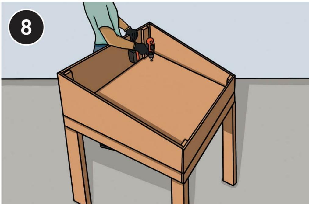
**Stand the base upright** on a flat, level surface. Set the box frame in place on the top of the base. Check that it is properly oriented; the box should be flush with the skirt boards all around. When you're sure the position is correct, screw the floor of the box to the top of each leg with at least two 2" deck screws.
