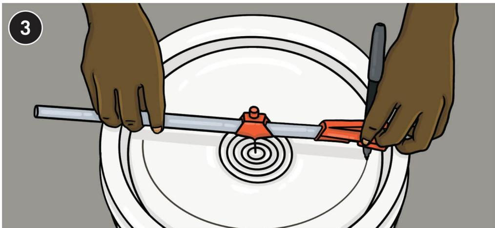
**Use a compass or trammel** on the bottom and lid of the bucket to mark a centered circle on each. The circle should be about  $9\frac{1}{2}$ " in diameter on the lid and about  $8\frac{1}{2}$ " in diameter on the bottom. Use a handsaw to cut the bucket in half.
