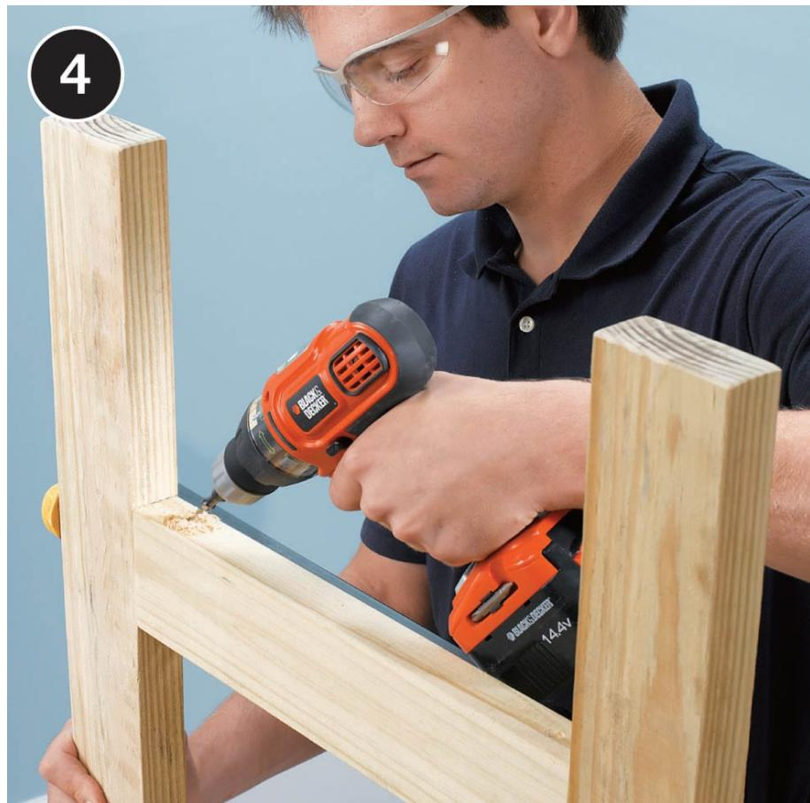
**Mark the inside edge of each leg,** 10" up from its bottom end. Measure the distance between each leg pair and cut a leg support to fit snugly between the legs, using the 10' 2 x 4. Install the leg supports with their bottom edges on the marks; drive 3½" screws toenail style through the top and bottom edges of the supports and into the legs.
