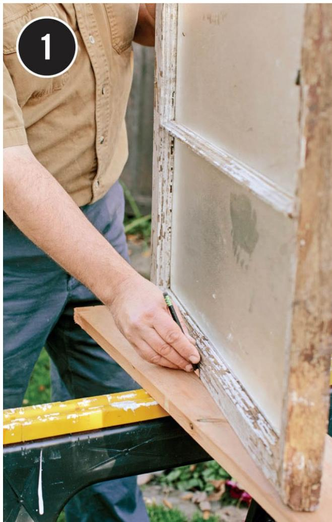
**Inspect a 1 x 6 fence board**, at least 24" long, to ensure that it is straight and free of defects. Measure from one corner, down 24" to the bottom edge of the board, creating a right-angle triangle. Use a speed square, or the edge of the window, to mark a straight line up from the bottom point of the triangle (the lower tip of the hypotenuse).
