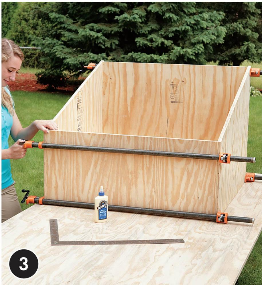
**Assemble the front, back and side panels** into a square box. Glue the joints and clamp them together with pipe or bar clamps. Adjust until the corners are square.
