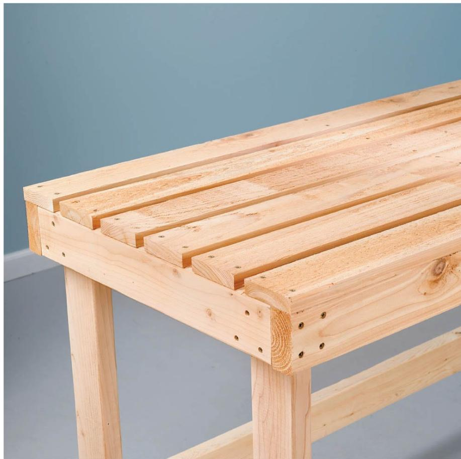
**1 x 4 or 1 x 6 cedar boards or decking boards** make an attractive top surface and offer some runoff, depending on how widely the boards are gapped. For the bench top, run boards parallel to the length of the top frame; for the shelf, run them perpendicular to the length of the shelf frame.
