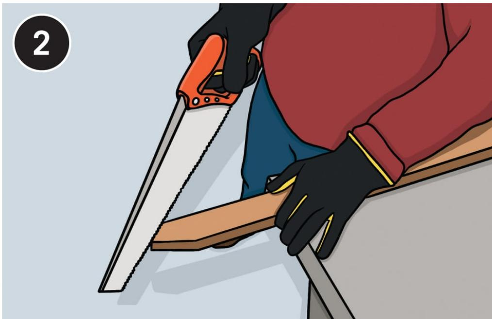
**Saw two  $13\frac{1}{2}$ "-long corner post stakes** from pallet stringers. Cut two corner posts 12" long. Saw the ends of all the posts in 3" points. The points don't need to be precise; cut them with a table saw if you have access to one, or with a circular saw or hand saw.
