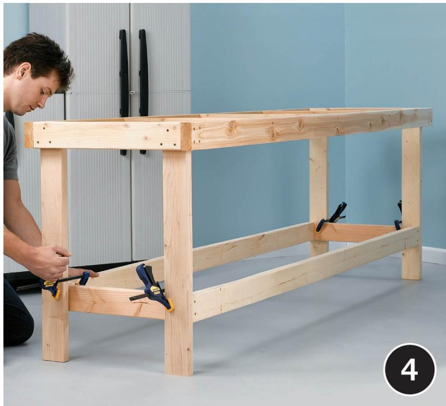
**Assemble the shelf frame** in the same manner as the top frame. Mark the inside face of each leg 10" up from the bottom end. Position the shelf frame with its top edges on the marks, and fasten it to the legs with 2½" deck screws driven through the frame ends. The side frame pieces should be flush with the outside edges of the legs.
