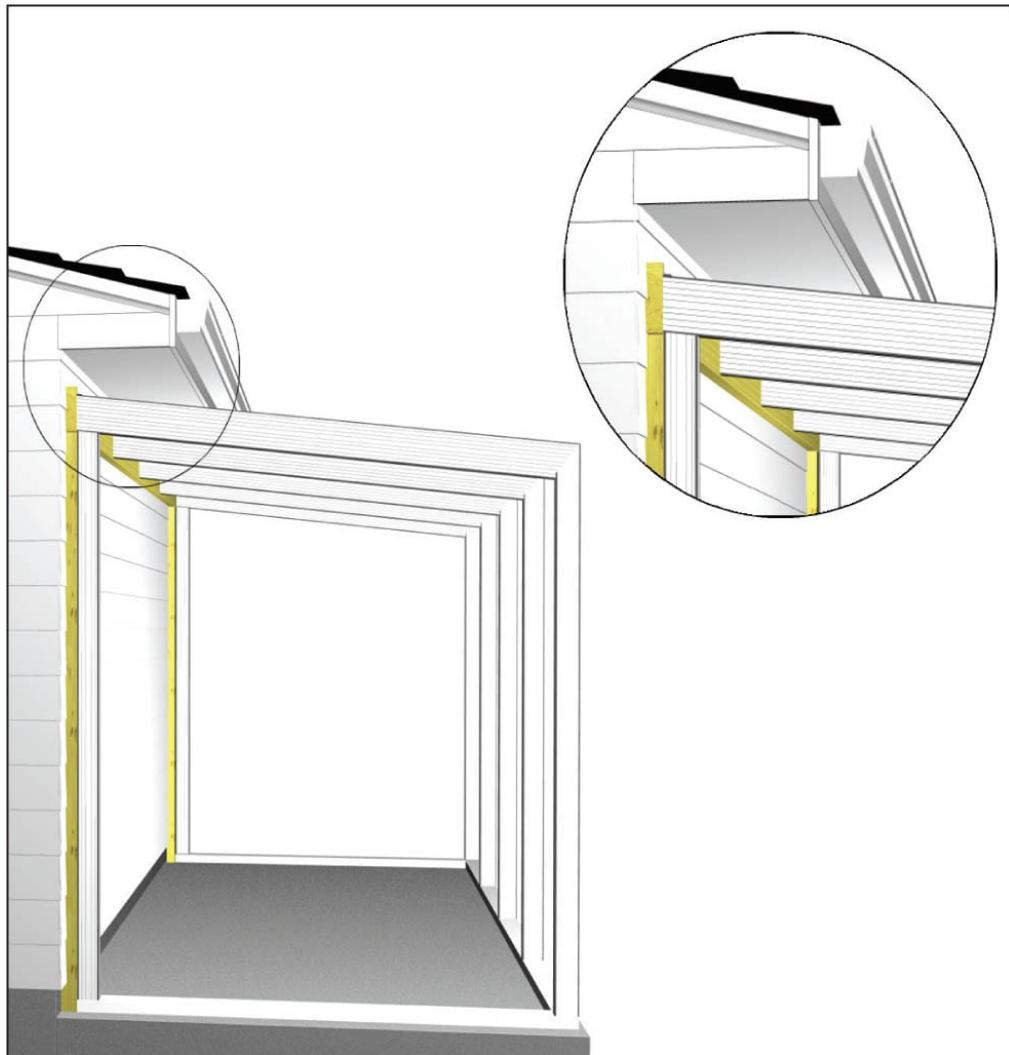
**Attach the ledger directly to the wall** if there is no eave overhang or if there is at least 6" of clear working space between the top of the ledger and the bottom of the eaves.
