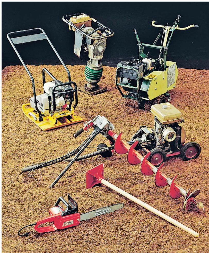
**Rent outdoor power equipment** if you need to do significant regrading to create a flat, level building base. Be sure to have your local utility company inspect for any buried utility lines first. (You may prefer to hire a landscaping company to do regrading work for you.)
