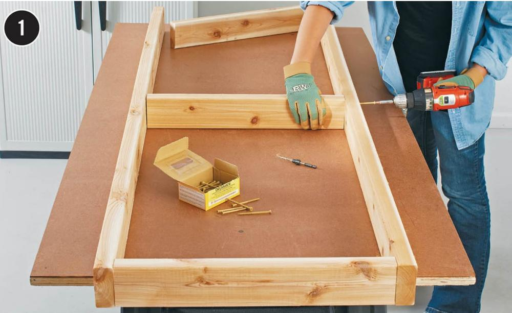
**Cut the parts** for the table frame to length and assemble the cedar top tray with the center divider. Predrill all screw holes to avoid splits, and use two screws at each corner. Use 2½" (or 3") deck screws. This design is for a 2 × 6 ft. tray, but you can make it larger or smaller.
