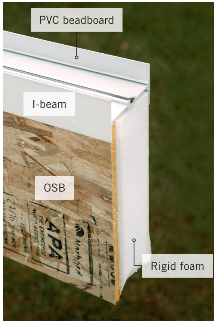
**Roof panels** come in varying thicknesses depending on the thickness of the rigid foam insulation board that is used (here, 4"). The narrow filler panel seen here features washable PVC beadboard on the interior side to create a ready-to-go ceiling once it is installed. The exterior side of the panel is 5/8" oriented strand board (OSB) to create a surface for installing building paper and asphalt shingles.
