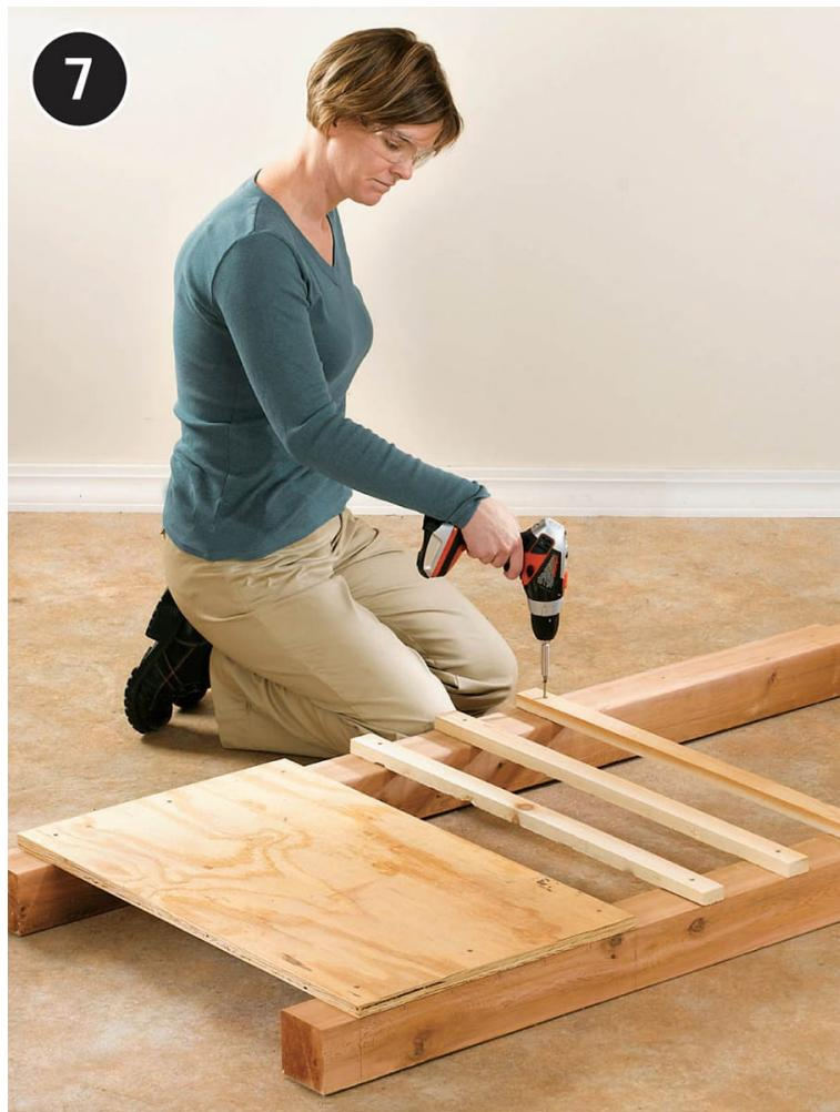
8. Attach the siding with 2-inch screws. Flip the project over and repeat the process to attach siding to the other side.
