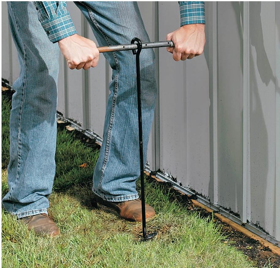
**Earth anchors, or anchor stakes,** are often used to tie down very lightweight greenhouses and crop covers to prevent them from blowing away. A typical anchor is a long metal rod with a screw-like auger end that is driven into the ground. An eye at the top end is used for securing a cable or other type of tether attached to the greenhouse.
