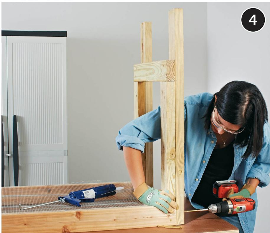
**With the tray turned upside down**, fit the legs onto the ends. Check that they're square to the frame and sitting flat underneath it—if you see daylight between the inner leg and the tray, trim the outer leg a little so the gap disappears. Screw each leg to both parts of the cedar frame.
