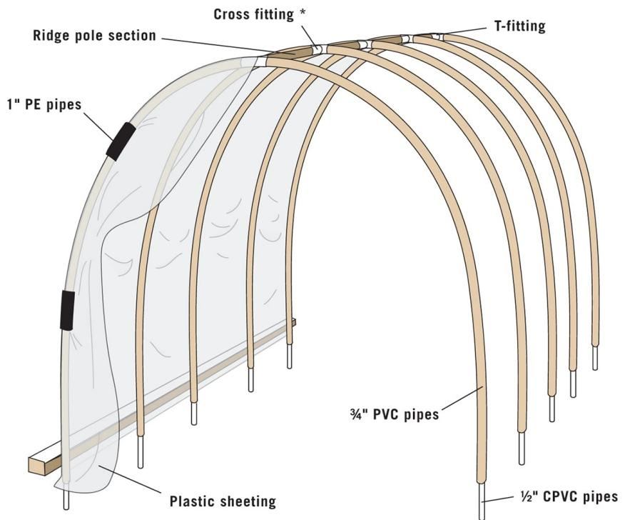
**\* If you can't find cross fittings, use a T fitting placed off center in each direction for the center hoops, and a filler piece of pipe between them**
