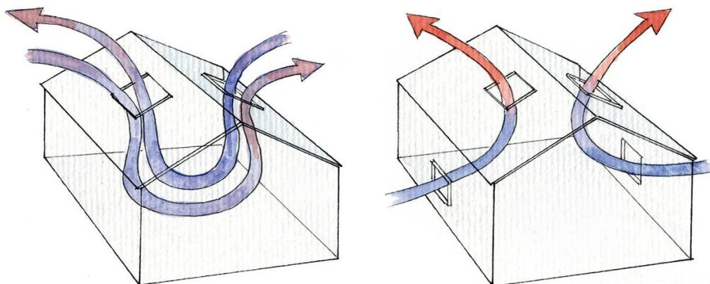
**Venting your greenhouse**—Installing at least one operable roof vent on each side of the ridgeline creates good air movement within the structure. Adding lower intake vents helps for cooling. Adding fans to the system greatly increases air movement.
