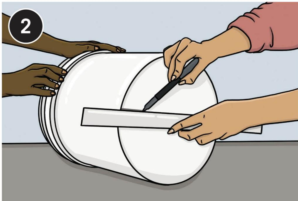
**With the lid securely attached,** carefully measure and mark a cut line across the center of the lid. Use a level to extend the cut line down each side of the bucket and across the center of the bottom.
