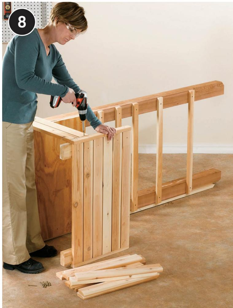
9. Attach the bottom supports to the front and back legs. The bottom of the front end of the bottom support should be flush with the bottom of the siding. The bottom of the back end of the bottom support should be positioned 2 inches up from the bottom of the back post. Drive one screw through the front end of the support and into the front leg and two screws into the back legs. Attach the bottom to the bottom supports with four 2-inch screws—two into each support.
