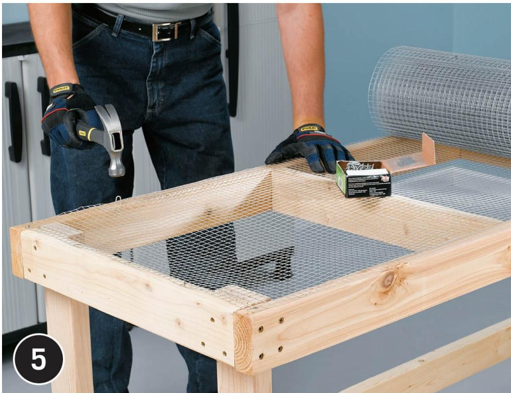
**Add the top and shelf surface material.** Galvanized wire mesh fencing is shown here (see next page for other options). Cut the 24"-tall fencing to length at 95", using aviation snips. Round over any sharp cut ends of wire with a metal file. Center the mesh over the top frame, leaving a  $\frac{1}{2}$ " margin at all sides. Fasten the mesh with  $1\frac{1}{2}$ " horseshoe nails. Trim and install the shelf mesh in the same fashion.
