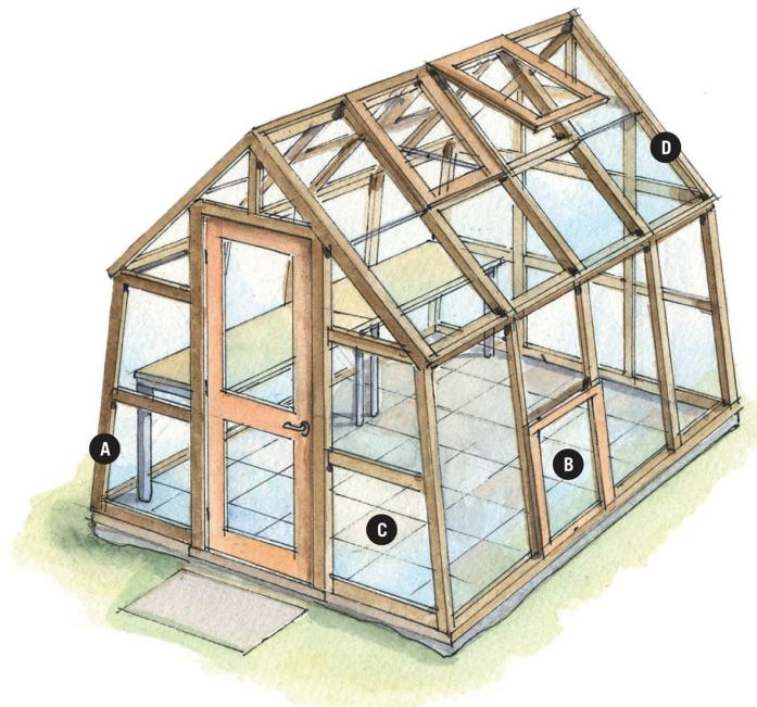
**Especially suitable for low-growing crops**, such as lettuce, this design has sloping sides that allow maximum light transmission. However, large panes of glass, which may be 30 by 59", are expensive to replace. The panes can be polycarbonate panels to save money or to diffuse light.
