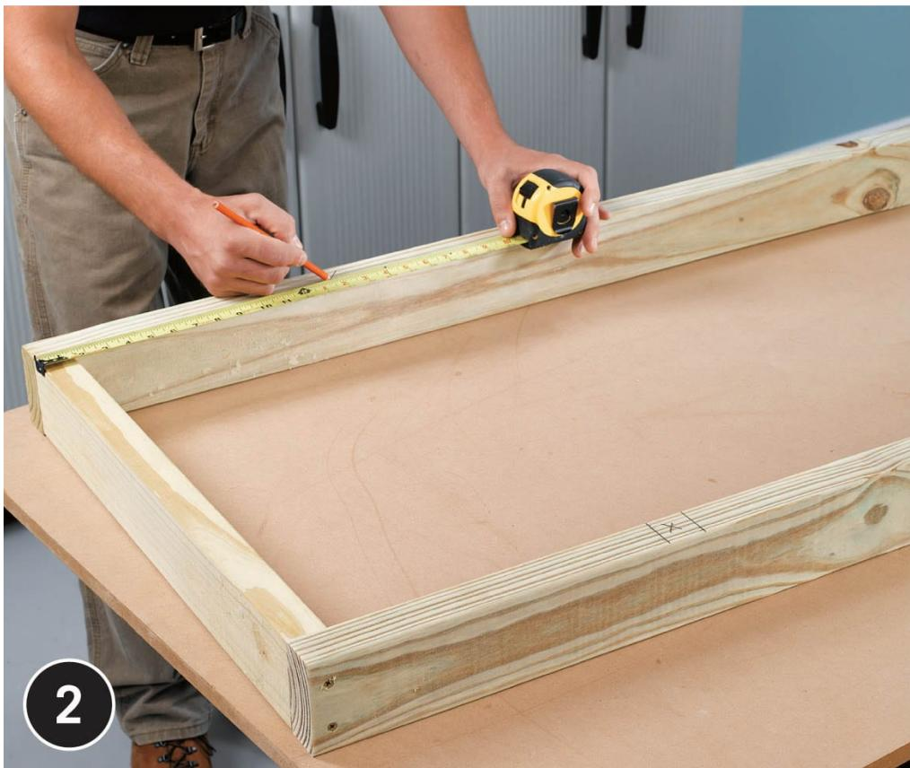
**Mark the layout for the top supports.** Measuring from one end of the top frame, mark both frame sides every  $13\frac{5}{8}$ ". Check the top frame for square, using a framing square. Install the top supports between the frame sides with  $3\frac{1}{2}$ " deck screws driven through the frame sides and into the supports. Make sure the supports and frame sides are flush across the top.
