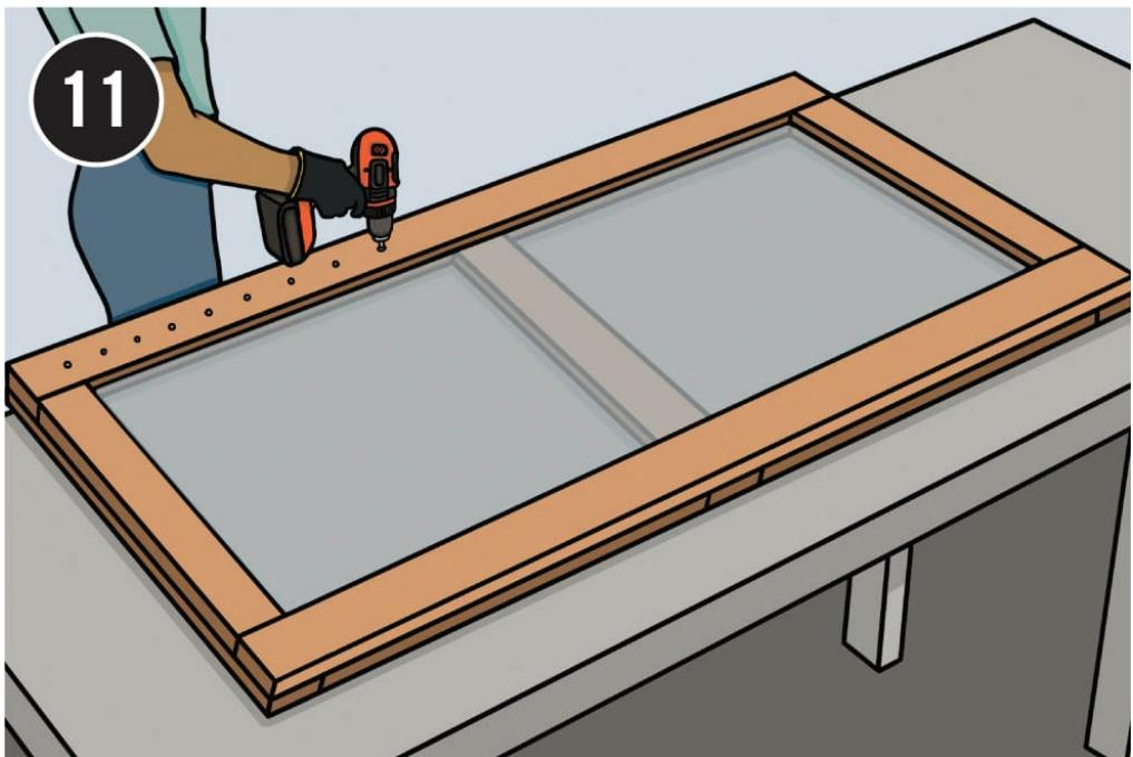
**Lay the bottom frame pieces** on top of the top frame. Make sure it is aligned all the way around, and then screw the frame boards to the top frame, using 1" deck screws. Use one screw every 3".
