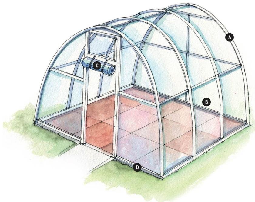
**Made of PVC or metal framing** and plastic glazing, this lightweight, inexpensive greenhouse is used for low-growing crops that require minimal protection from the elements. Because it does not provide the warm conditions of a traditional greenhouse, it is designed mainly for extending the growing season, not for overwintering plants. Ventilation in this style can be a problem, so some models have sides that roll up.
