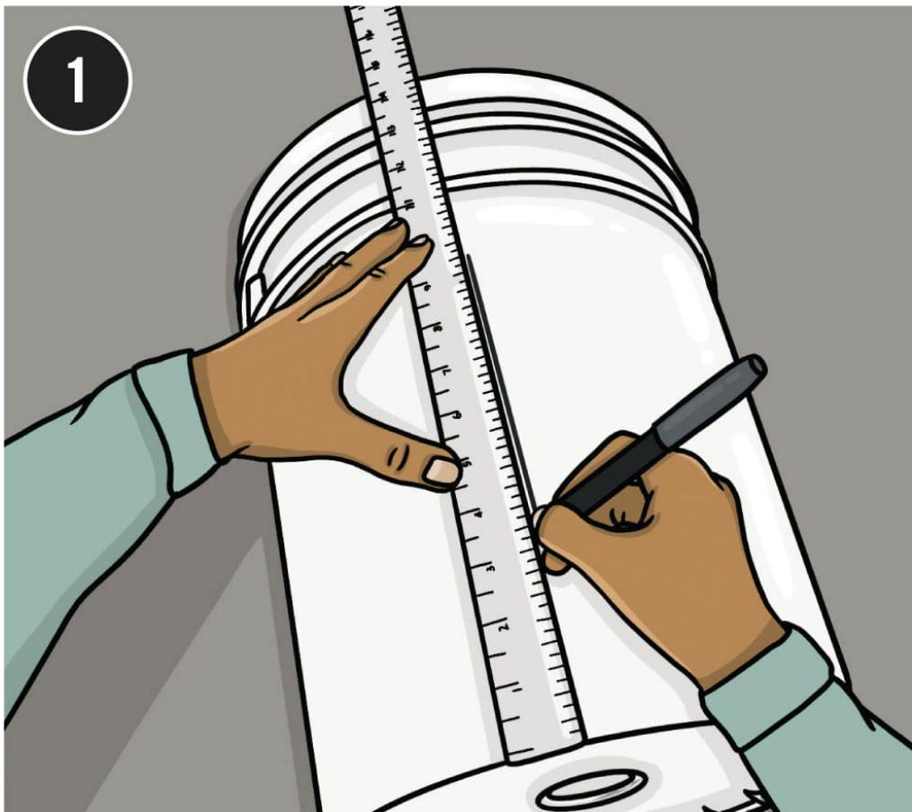
**Measure and mark** two 2" vertical spines on opposite sides of the bucket. The spines should run from right under the bottom ridge on the mouth of the bucket, down to 3" from the bottom. Use a flexible straightedge to draw a cut line from the bottom corner of each spine to the bottom corner of the opposite one, on each side. This will create the outline of two windows.
