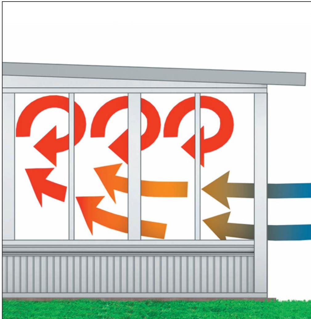
**Without roof vents, hot air is trapped in the sunroom,**
