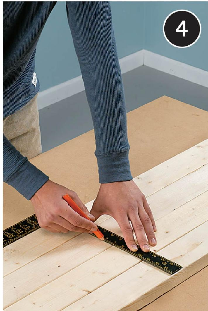
**Mark the shelf locations** onto the legs. Measuring from the bottom of one leg, make marks at  $7\frac{1}{2}"$ ,  $31\frac{1}{2}"$ , and  $55\frac{1}{2}"$ . These marks represent the top edges of the shelves; the top shelf is installed flush with the top ends of the legs. Use the framing square to transfer the layout marks to the remaining three legs.
