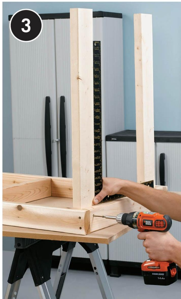
**Attach the legs** to the inside corners of the top frame, using 2½" deck screws. The top ends of the legs should be flush with the top edges of the frame. Use a framing square to make sure each leg is perpendicular to the frame before fastening.
