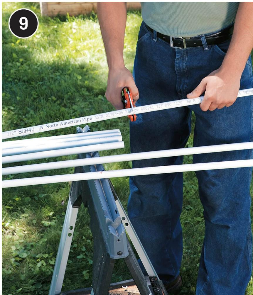
**Prepare the cover frame ribs** by cutting six  $\frac{3}{4}$ "-diameter PVC pipes to length at 96", using a hacksaw or tubing cutter. Then, make a mark at the midpoint (48") of each rib, and drill a  $\frac{3}{16}$ " hole straight through the pipe at each mark.
