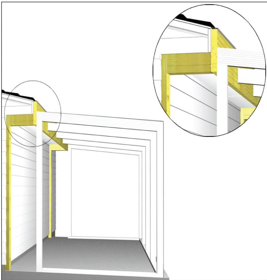
**If the maximum height of the sunroom** brings it up against or within 6" of the bottom of the eave overhang, extend the fascia on the eave downward and fill in with boards or siding between the cornice and the back post for the sunroom.
