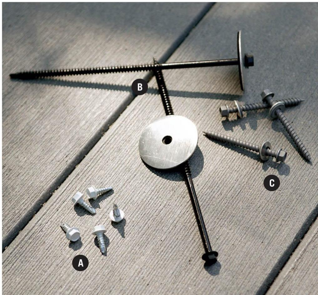
**Fasteners for this sunroom include** self-tapping hex-head screws (1") with low-visibility white heads (A), insulation screws (7") with 2"-dia. fender washers (B), and galvanized self-tapping hex-head screws (2") with self-sealing EPDM rubber washers (C).
