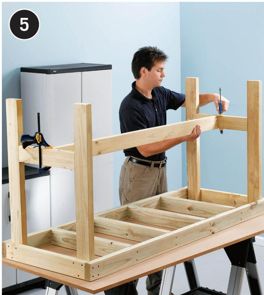
**Cut the 2 × 4 stretcher** to fit snugly between the leg supports, using the remainder of the 10' 2 × 4. Install the stretcher so it's centered side-to-side on each support, with the top edges flush. Drive 3½" screws through the outsides of the leg supports and into the stretcher ends.
