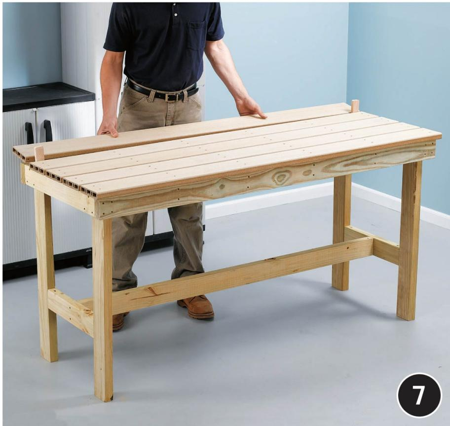
**Install the remaining deck boards** so all of their ends are perfectly aligned and each board is gapped  $\frac{1}{8}$ " from the next (without gaps, the joints would trap dirt). Use pieces of  $\frac{1}{8}$ "-thick hardboard or two  $\frac{1}{8}$ "-diameter drill bits to set the gaps. The last board should overhang the rear frame side by  $\frac{3}{4}$ ".
