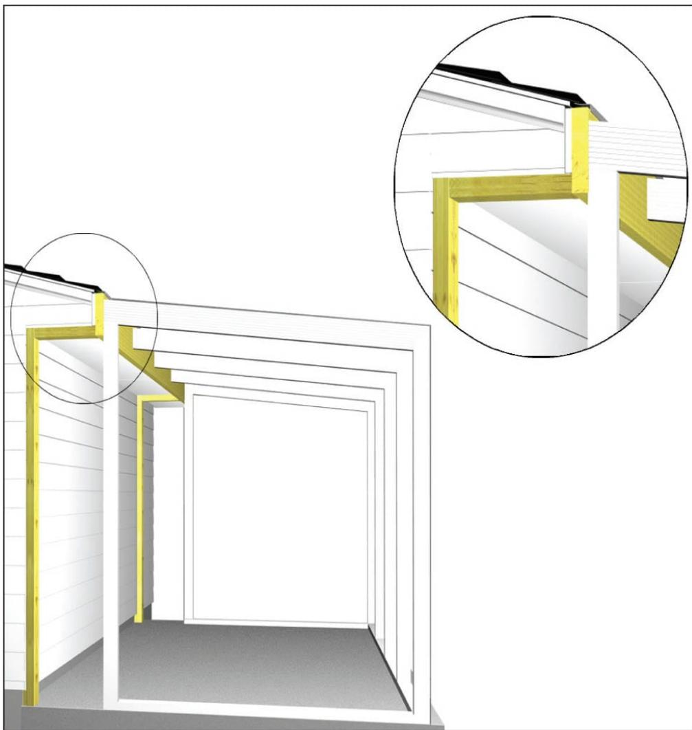
**The ledger for the sunroom** can be attached directly to the fascia board as long as the highest point of the sunroom roof remains slightly lower than the roof covering. Be sure to attach the ledger so the lag screws hit into the ends of the rafter tails.
