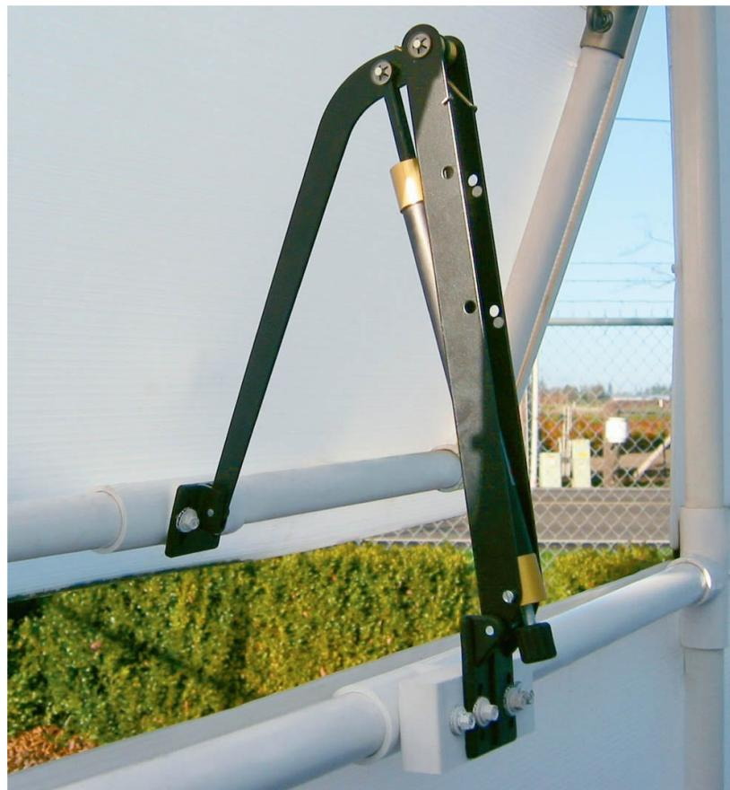
**A simple solar opener like this** can be retrofitted to a greenhouse vent window to open it whenever the heat increases on the inside of the greenhouse. A paraffin core expands, causing the opener to open the vent. Simple technology, but highly effective.
