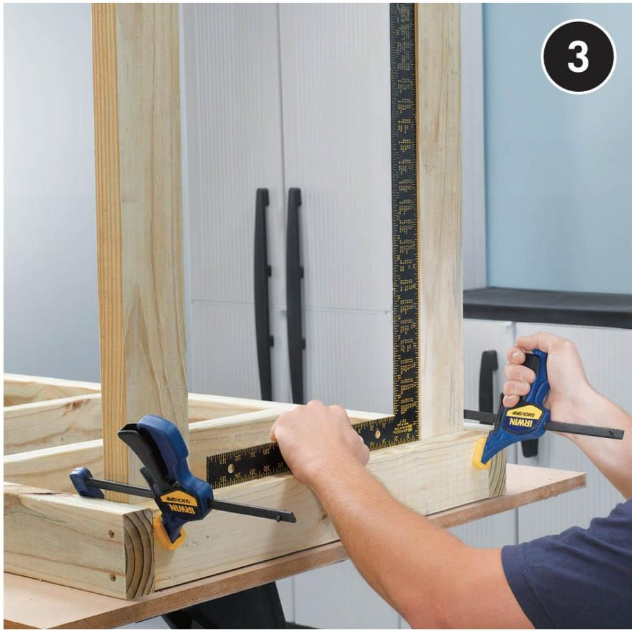
**Cut the four legs** from one 12' 2 × 4. Round-over the edges on the bottom end of each leg, using sandpaper, a file, or a router and roundover bit; this prevents splintering if the table is slid around. Install the legs at the inside corners of the top frame, driving 2½" deck screws through the legs and into the top frame ends. Also screw through the top frame sides and into the legs. Make sure the legs are square to the frame before fastening.
