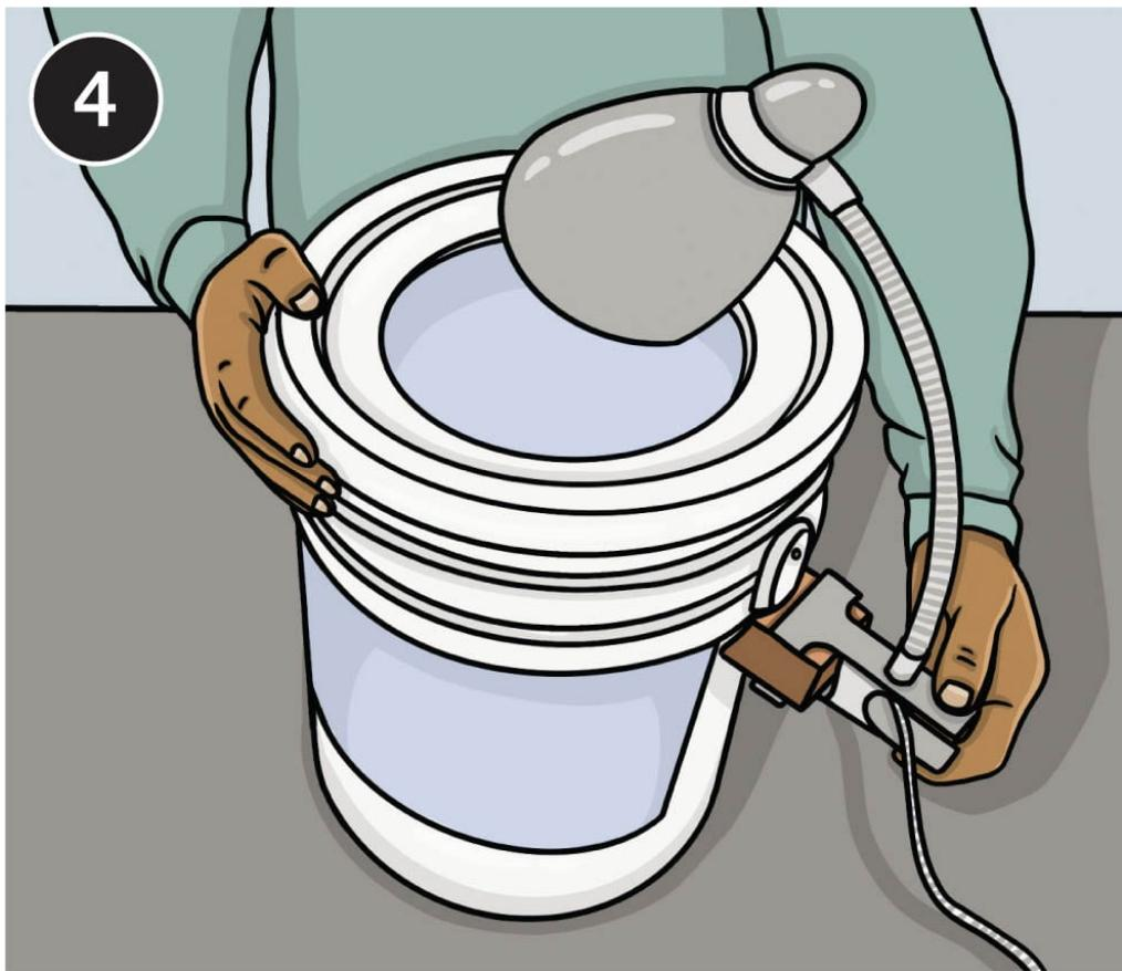
**Cut a 3" long mounting block** from a  $1 \times 2$  scrap. Use 2" deck screws to mount it at the top of one of the spines. Fill the base with potting soil and plant the seeds you want to grow. Place the bucket in its final location on top of the second lid. Clip a flexible stem grow light to the mounting block and set a timer at the plug.
