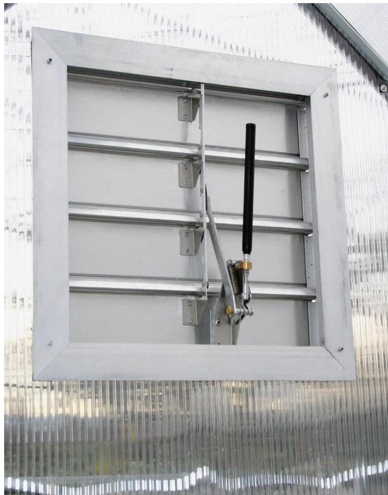
**This shutter assembly** comes as a kit; the probe automatically opens the shutter when the heat inside the greenhouse reaches a preset level.
