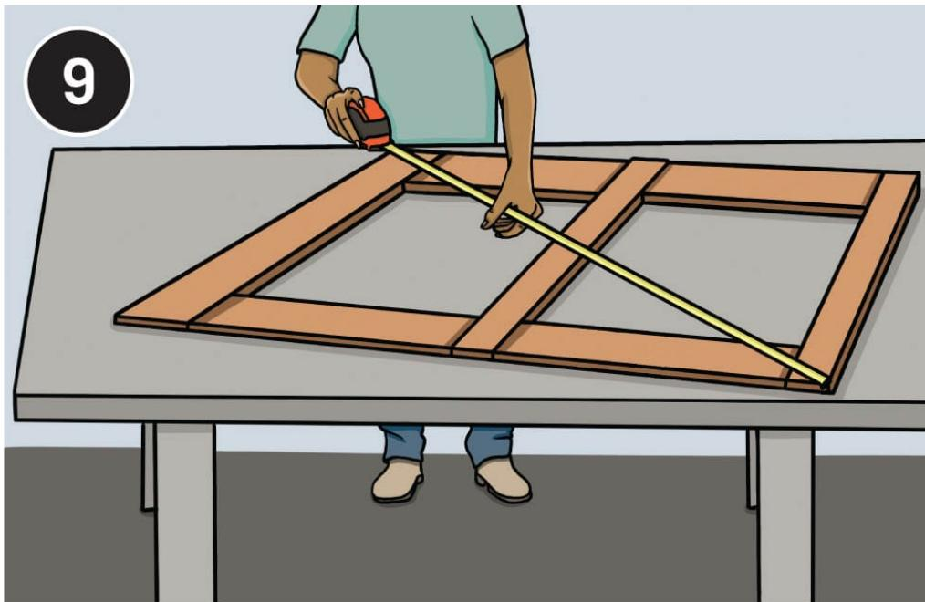
**Layout out the lid bottom frame** on the work surface, with short rails separating the three stiles at their ends. Check the diagonal measurements to ensure the frame is square, then staple the boards together.
