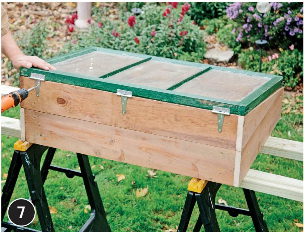
**Mark the placement** of the three hinges and screw them to the window frame and rear box frame. Measure and mark for the sash handle on the front of the frame and screw it in place. If desired, cut a 1x scrap piece to about 15" long to use as a support post to hold the window open when you work in the cold frame.
