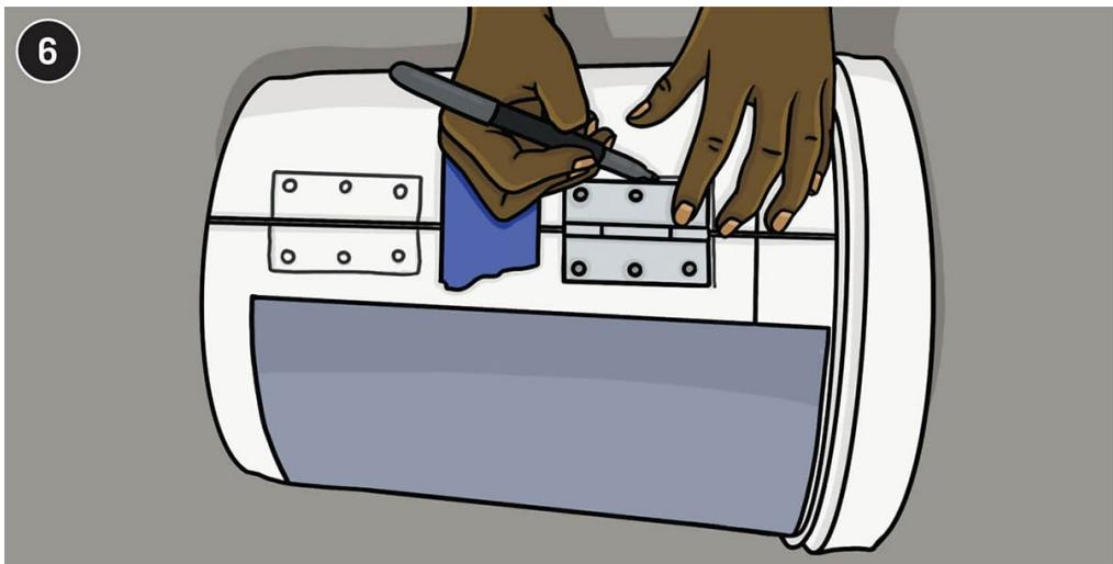
**Using painter's tape** to tape the two bucket halves together and mark one long side for the placement of the hinges. They should be centered along the line, about 6" apart.
