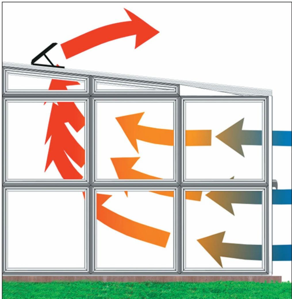
**A single roof vent creates an escape route for hot air,** allowing you to regulate the temperature and keep the room cooler during hot weather. Multiple roof vents increase the ventilation efficiency but increase the chances for leaks.
