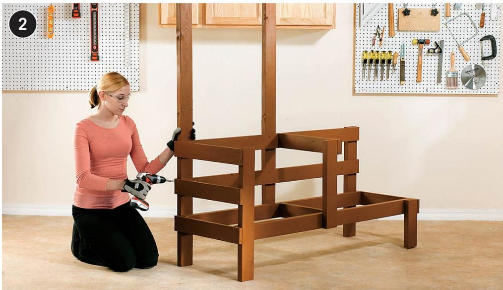
**Attach two back rails and one bottom rail** to the long leg, back strut, and back right mid-length leg with 2" deck screws. Check that all of the parts intersect at 90° angles. Attach the front rail and one bottom rail to the left front mid-length leg, front strut, and short leg. Connect the back assembly and front assembly by attaching them to the cross supports.
