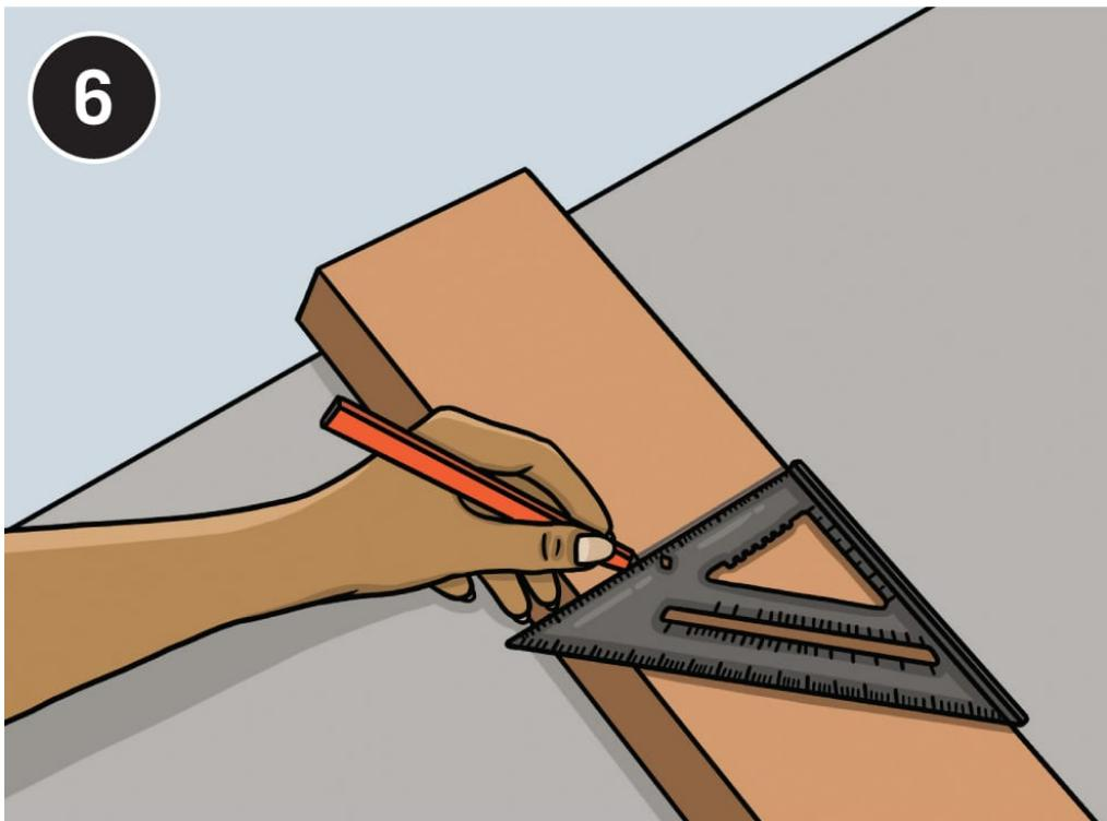
**Measure up from the bottom** of the legs and use a speed square or straight edge to mark lines 10" up from the bottom of each leg. Use the lines as guides for positioning the lower skirt board. Drill pilot holes and screw the boards to the legs as before. Repeat the other two legs.
