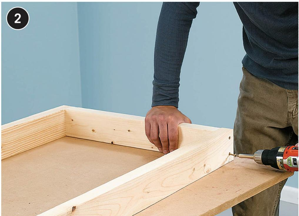
**Assemble the shelf frames** with 3½" deck screws. Position the side pieces of each frame over the ends of the end pieces and so their top edges are flush. Drive two screws through the sides and into the ends. Complete all four shelf frames using the same technique.
