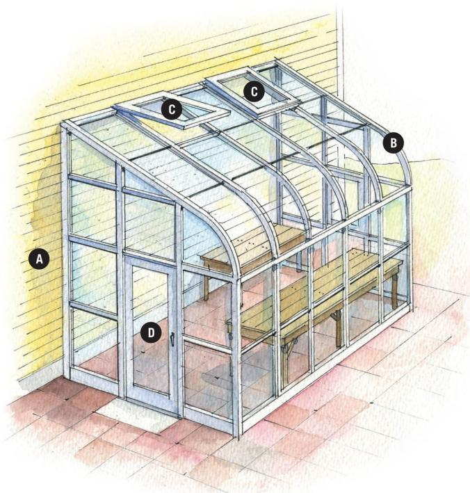
**Because it is attached to the house,** a lean-to absorbs heat from the home and offers easy access to utilities. This model shows curved eaves, a glazed roof, and glass-to-ground construction. Lean-tos can be built on kneewalls to provide more headroom and better heat retention than glass-to-ground styles. Sinking the foundation into the ground about 2 to 3' can conserve even more heat.
