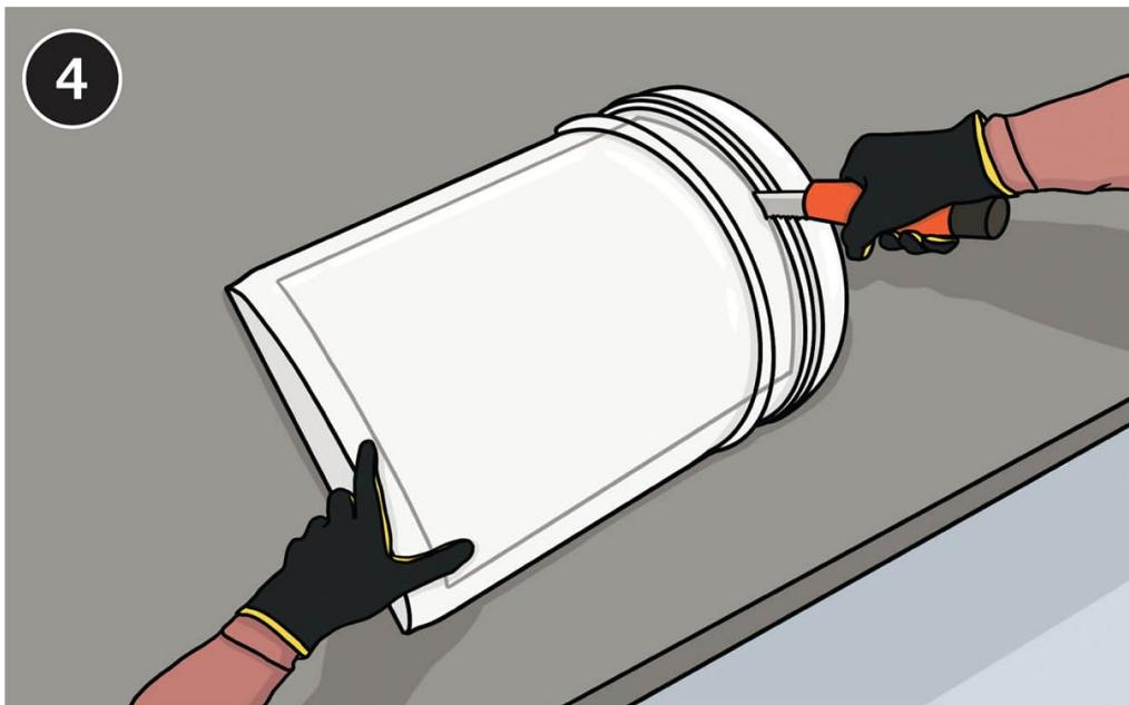
**Measure and mark** a 10" × 16" window in the bucket half with the end windows, centered across the body of the bucket. Drill an access hole and cut out the window. Note: A good shortcut for this is to cut out a 10" × 16" piece of stiff cardboard and use it as a template to mark the cutout.
