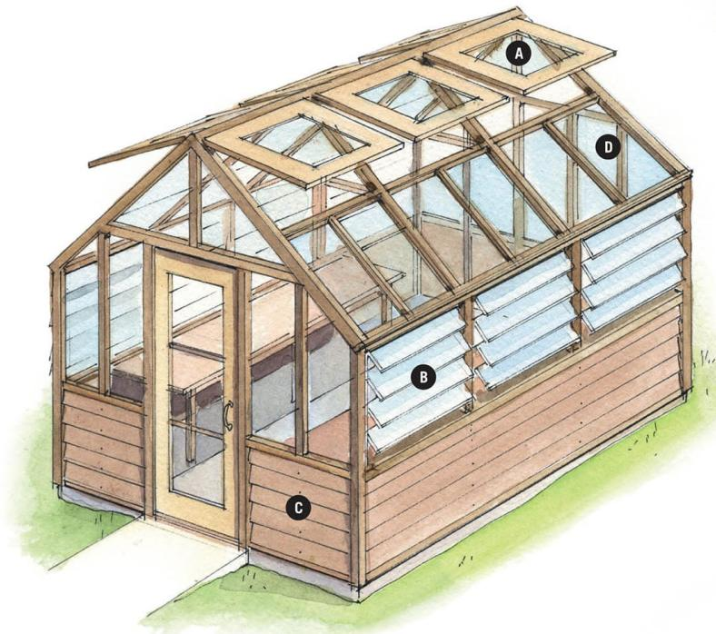
**Specifically designed for plants** that normally grow at high elevations and thrive in bright, cool conditions, this alpine house is unheated and has plenty of vents and louvers for maximum ventilation. Doors and vents are left open at all times (except in winter). Many rock-garden plants—edelweiss, sedum, and gentian, for example—thrive in the alpine house environment.
