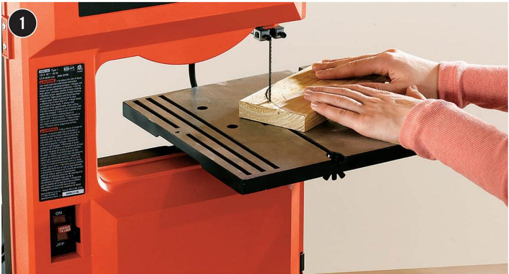
**Cut all of the frame and shelf parts** to length. Draw a  $3\frac{1}{2}$ -inch radius on the front bottom corner of each shelf support. Cut along the radius lines with a jigsaw or bandsaw. Sand the profiles smooth.
