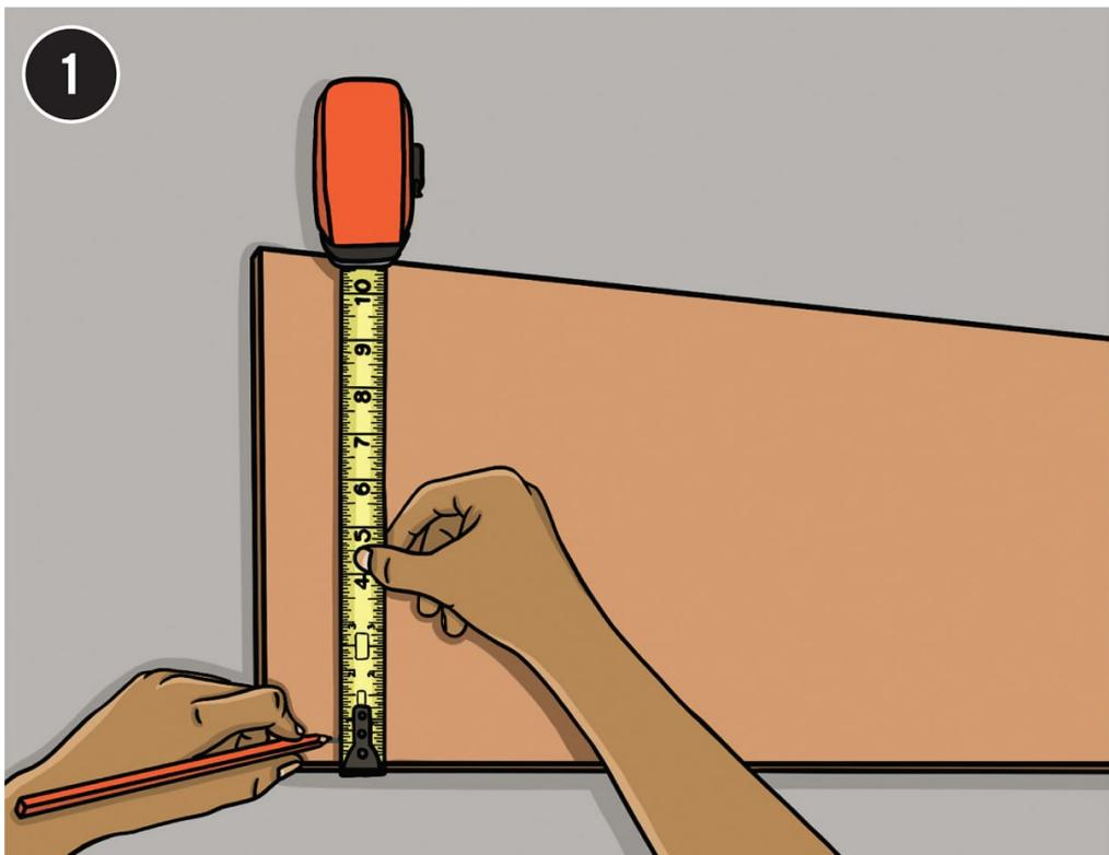
**Measure, mark, and cut** the plywood sheet according to the cut diagram ([here](#)). Cut the other lumber for the project to size.
