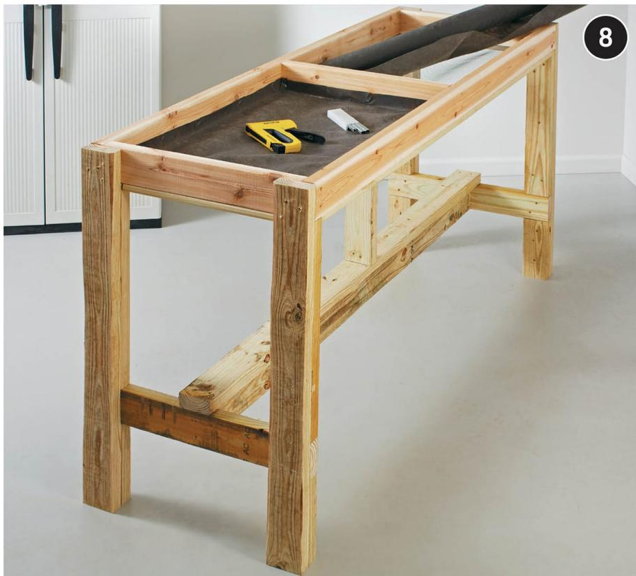
**Finally,** staple on landscape fabric or aluminum screen on the inside of the tray to hold the soil in. Fill the tray with a soilless growing media and fertilizer—not ordinary topsoil. For best results, replace the soilless mix every year, as it becomes compressed over time.
