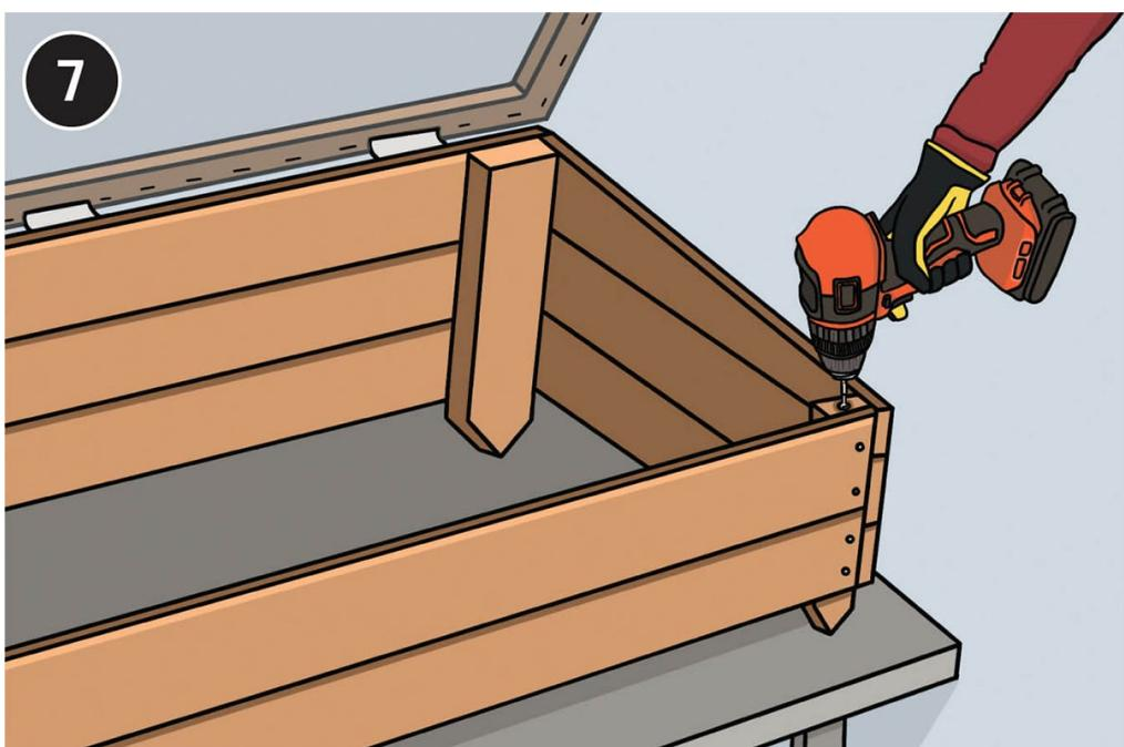
**Drill a shallow  $\frac{1}{4}$ " hole** in the top of one front corner post. Drill a matching hole in the frame corner, where it sits over the post. Use a  $\frac{1}{4}$ " dowel to prop the lid open as necessary for ventilation and temperature control.
