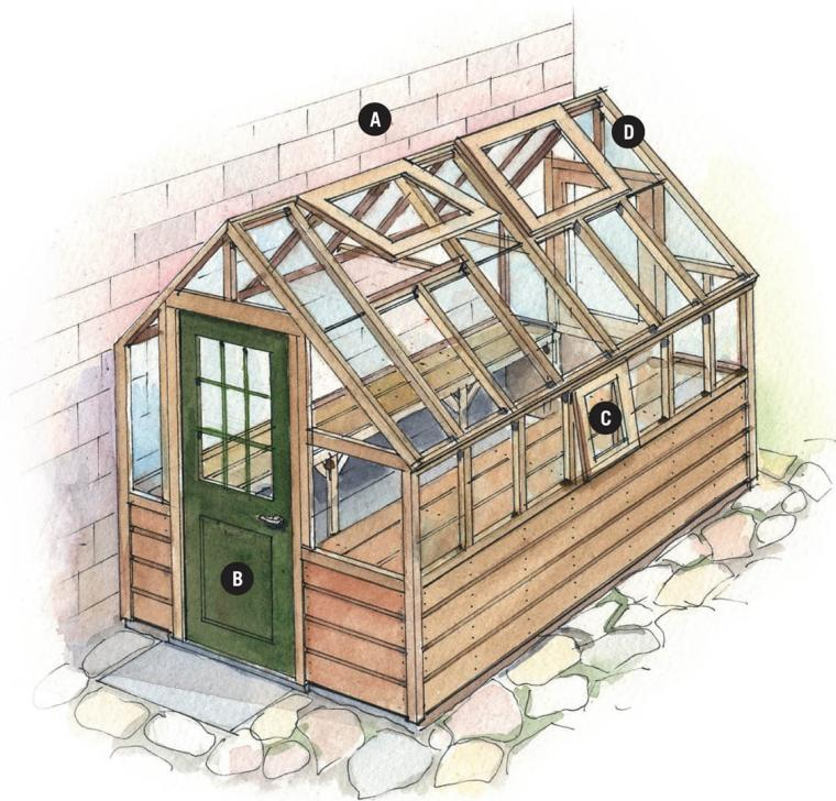
**Also attached to the house,** this type of greenhouse offers the benefits of a lean-to with even more headroom and better light transmission (though it offers less light than a freestanding model). Because of the additional framing and glazing, this style is more expensive to build than a traditional lean-to.
