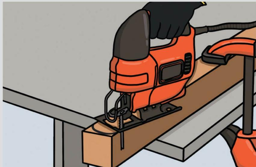
**OPTION:** For a more polished look, cut one end of each  $2 \times 2$  leg to a half-circle. Measure down 3" from one end, and mark a point centered side to side. Use that point to anchor a carpenter's compass or homemade trammel, to mark an arc along the end of the leg. Cut the arc using a jigsaw.
