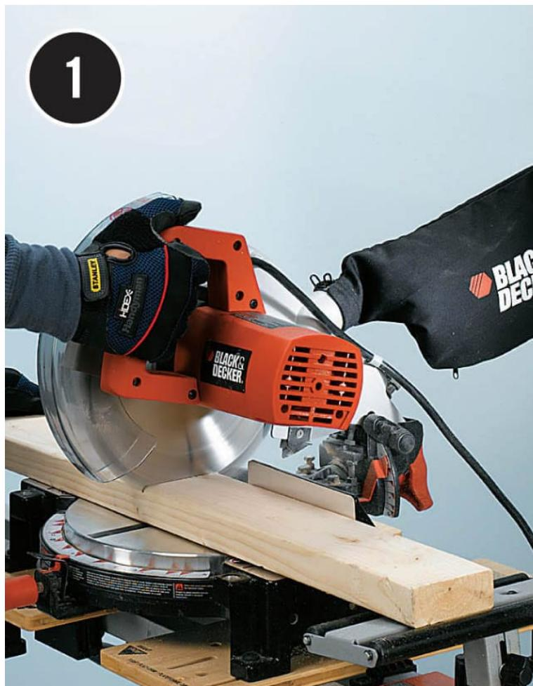
**Cut all of the wood** for the shelf frames, using a circular saw or power miter saw. Cut one shelf frame side and two shelf frame ends from each of four 8' 2 × 4s, and cut the remaining four shelf frame sides from two 10' 2 × 4s. Cut each of the four legs from an 8' 2 × 4.
