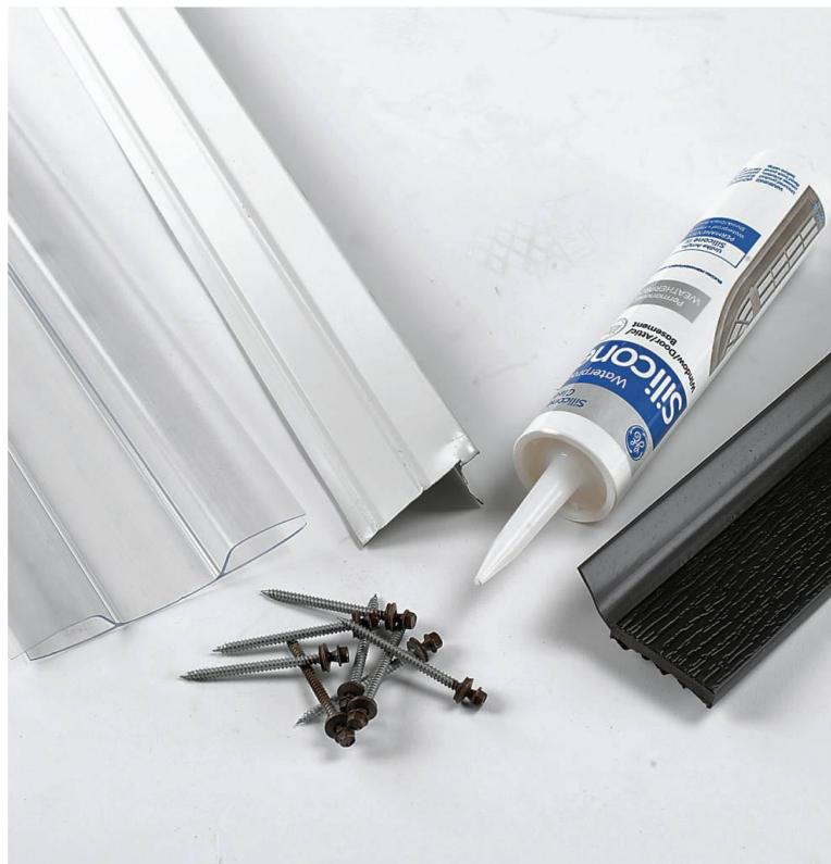
**Products for joining and fastening panels** include a panel seam trim, which has wide flanges on both edges to accept two panels that butt together; 100% silicone caulk for sealing seams (check with the panel manufacturer for compatibility of adhesives and caulk); and rubber-gasket pole barn screws for fastening panels to rafters or purlins.
