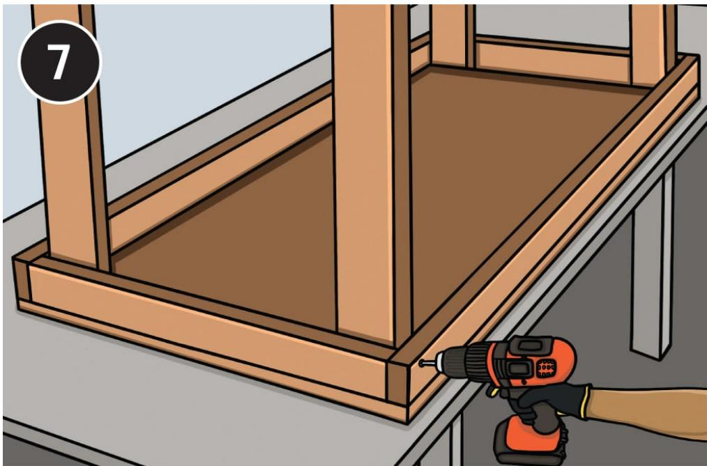
**Stand the leg pairs upside down** on the work surface, on their ends, parallel to one another (the skirt boards should be facing out). Position a top front skirt board between the legs, overlapping the ends of the side skirt boards you attached in step 6. Drill pilot holes and screw the board in place. Repeat with the second skirt board, and then the opposite side to complete the base.
