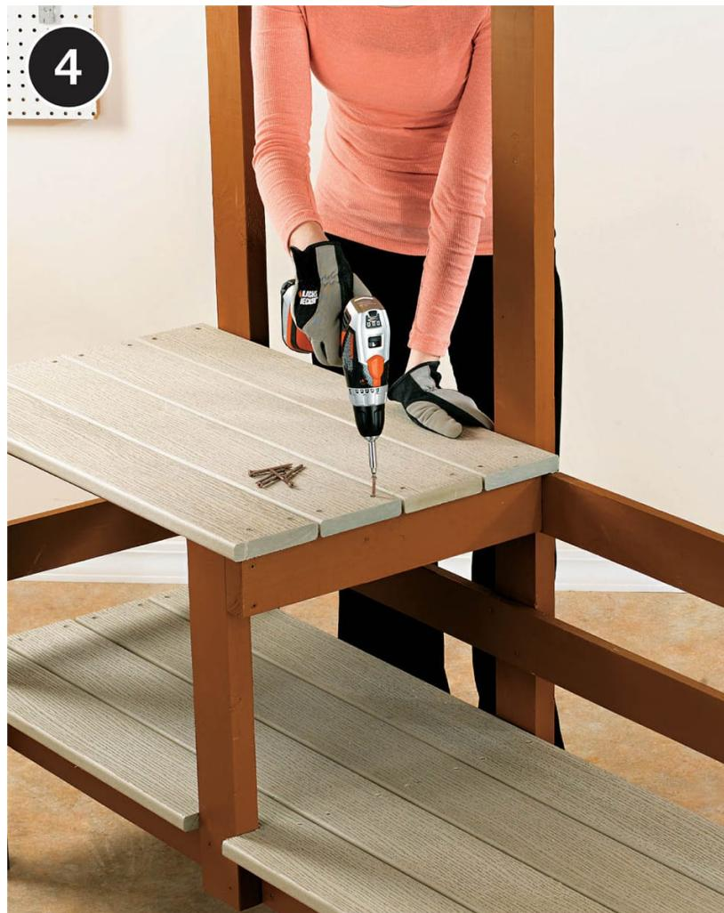
**Place the top and bottom** deck boards on the cross supports, leaving a  $\frac{1}{4}$ -inch space between the boards. Attach the deck boards with 2-inch deck screws. If you are using composite deck boards, use the recommended decking screws.
