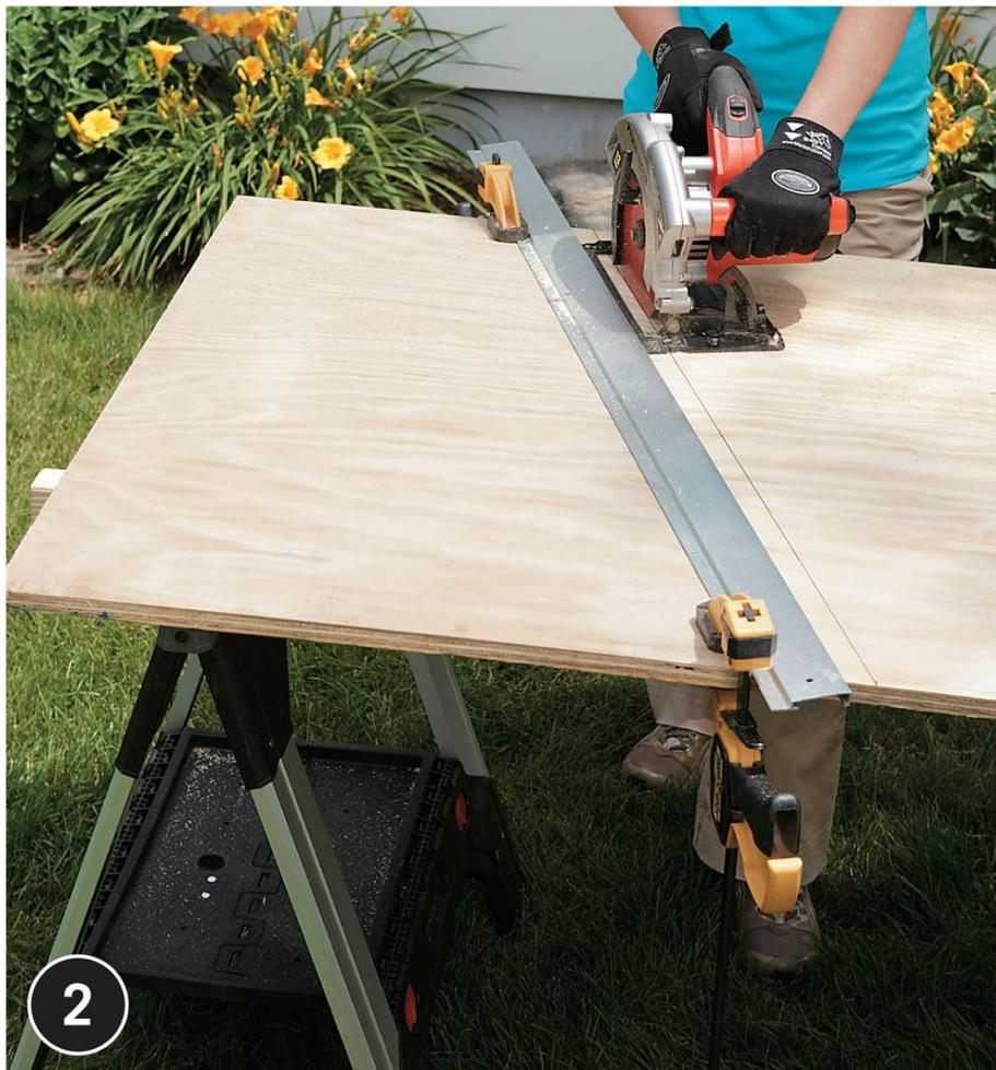
**Cut the parts to size** with a circular saw or jigsaw and cutting guide. Mark the cutting lines first (See diagram, previous page).
