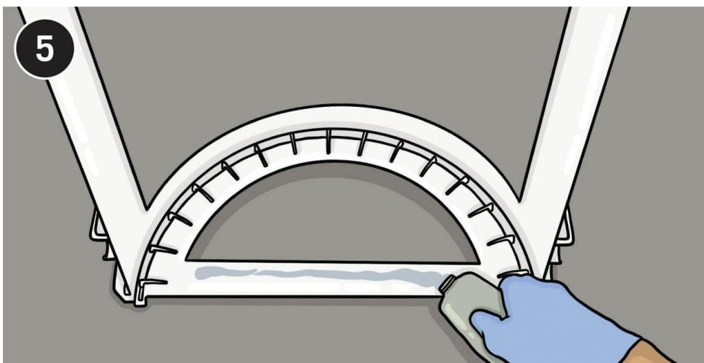
**Use plastic epoxy** to glue the 6-mil plastic windowpanes in place on the inside of the bucket, covering the window openings.
