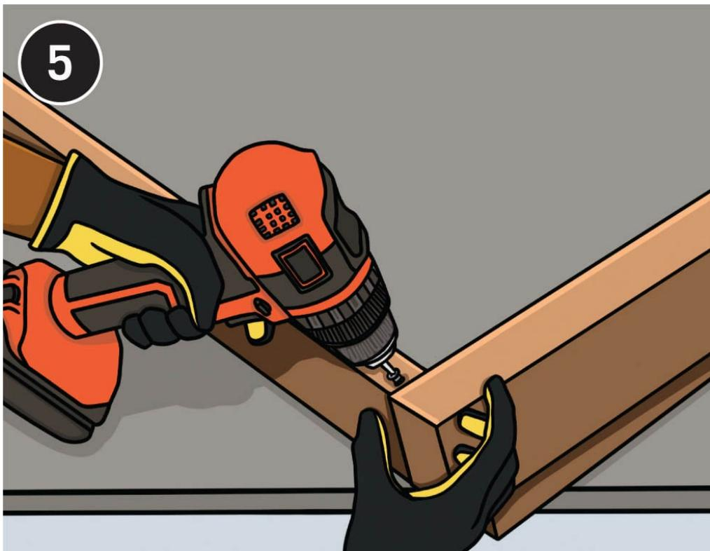
**Set the long brace** across the leg pairs. Drill pilot holes and screw the brace to the edges of the outside legs, flush all around. Repeat with the opposite, shorter base brace.
