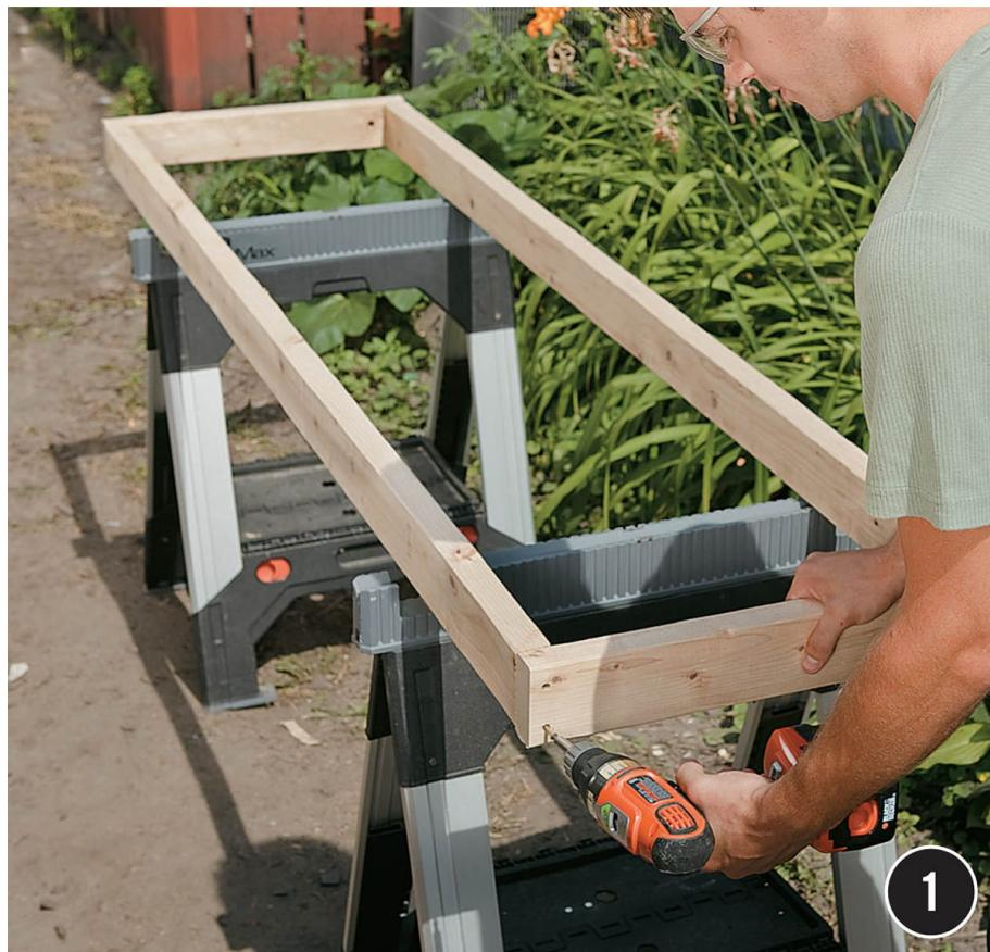
**Pre-assemble the frame** that is the benchtop support. Cut the  $2 \times 4$  front, back, and ends to length and then join them with 3" deck screws and exterior-rated wood glue.
