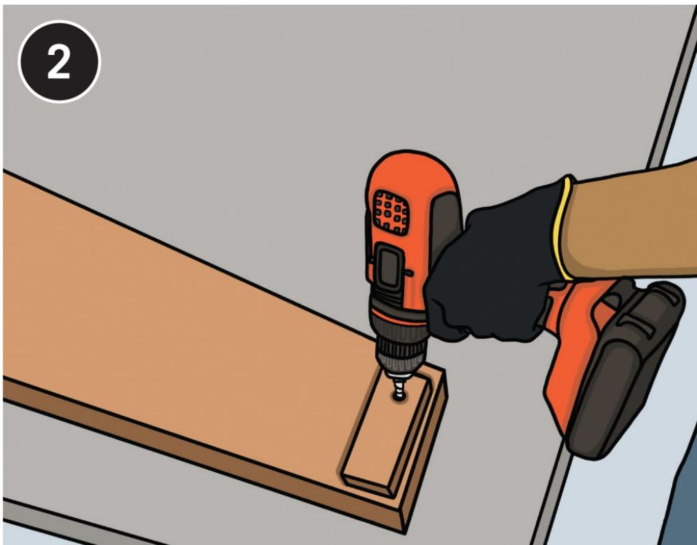
**Align a rear (long) cleat** along the back edge, with the bottom of the cleat at the mark. Screw the cleat to the side using 1 $\frac{3}{4}$ " deck screws. Repeat with the front cleat, along the front edge. Screw the cleats to the second side panel.
