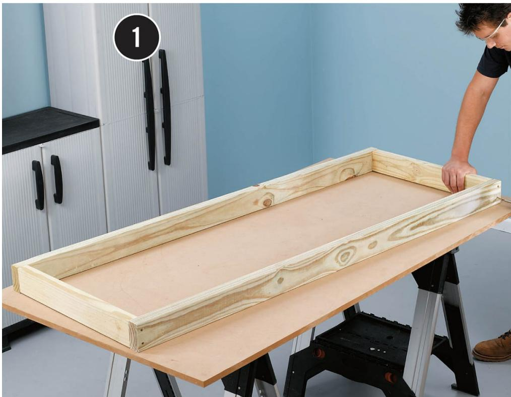
**Cut the two top frame sides** from one 12' 2 × 4, using a circular saw or power miter saw. Cut the two top frame ends and the four top supports from another 12' 2 × 4. Fit the side pieces over the ends of the end pieces so all top edges are flush. Fasten the pieces together with two 3½" deck screws at each joint.
