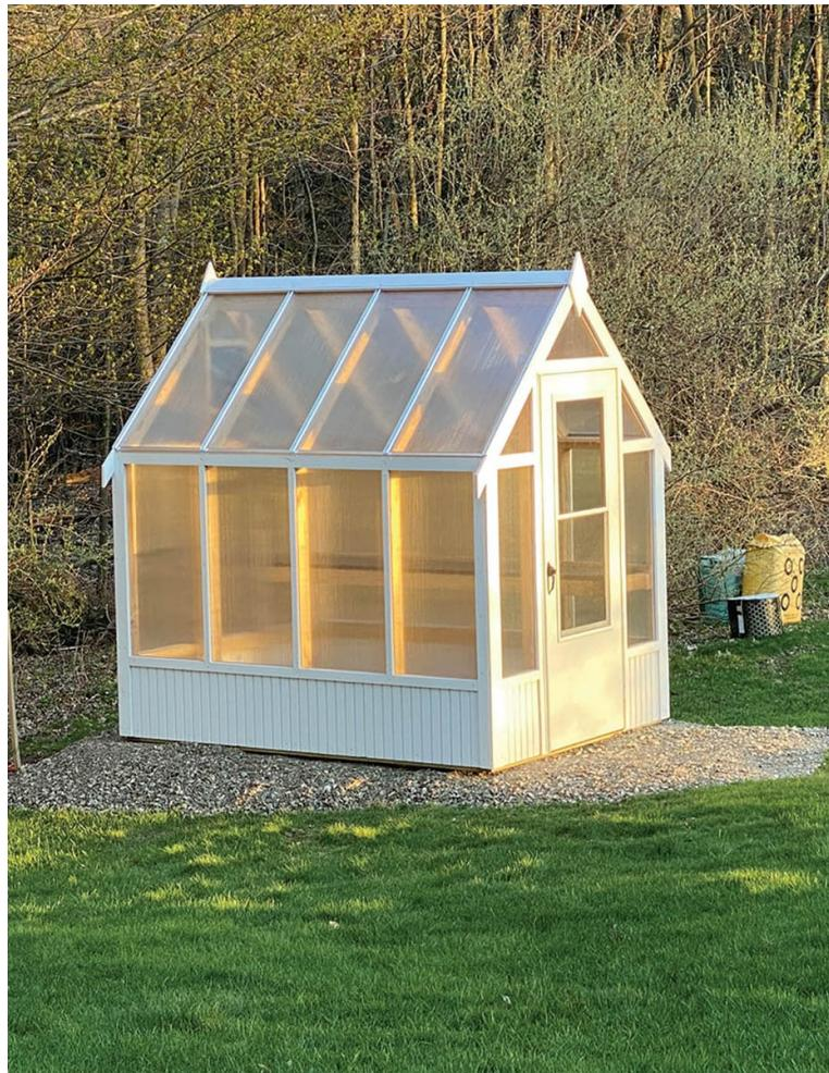
**Go prefab for quick and easy beauty.** This particular greenhouse is a prefab, not a kit. It's delivered as a completed structure, and is a handsome one. It features southern pine framing, UV-resistant, 8 mm twin-wall polycarbonate panels, and options like interior hanging plant hooks. The details that include a built-in kneewall and gable peak finial are the icing on the cake.
