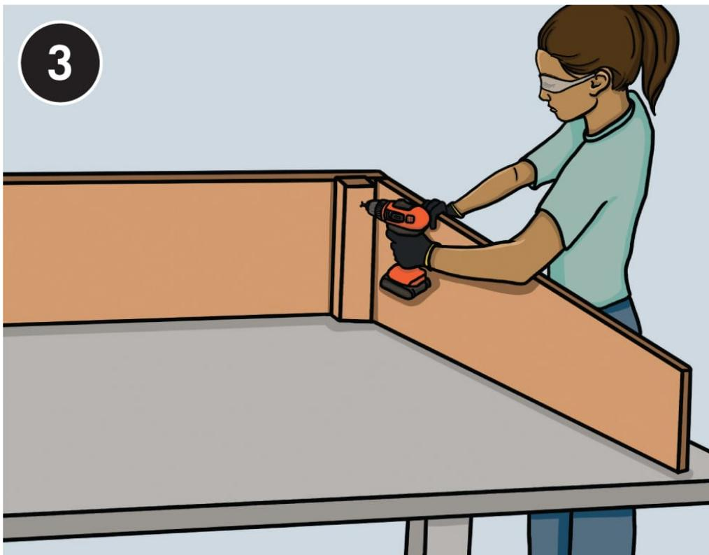
**Assemble the box frame** on a flat, level work surface. Align the box back along the back edge of one side, and screw the cleat to the back with  $1\frac{3}{4}$ " deck screws. Repeat the process to attach the second side to back. Finish the frame by screwing the front cleats to the front.
