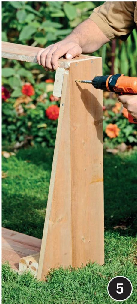
**Drill pilot holes** and screw the posts in place in each corner of the box.
