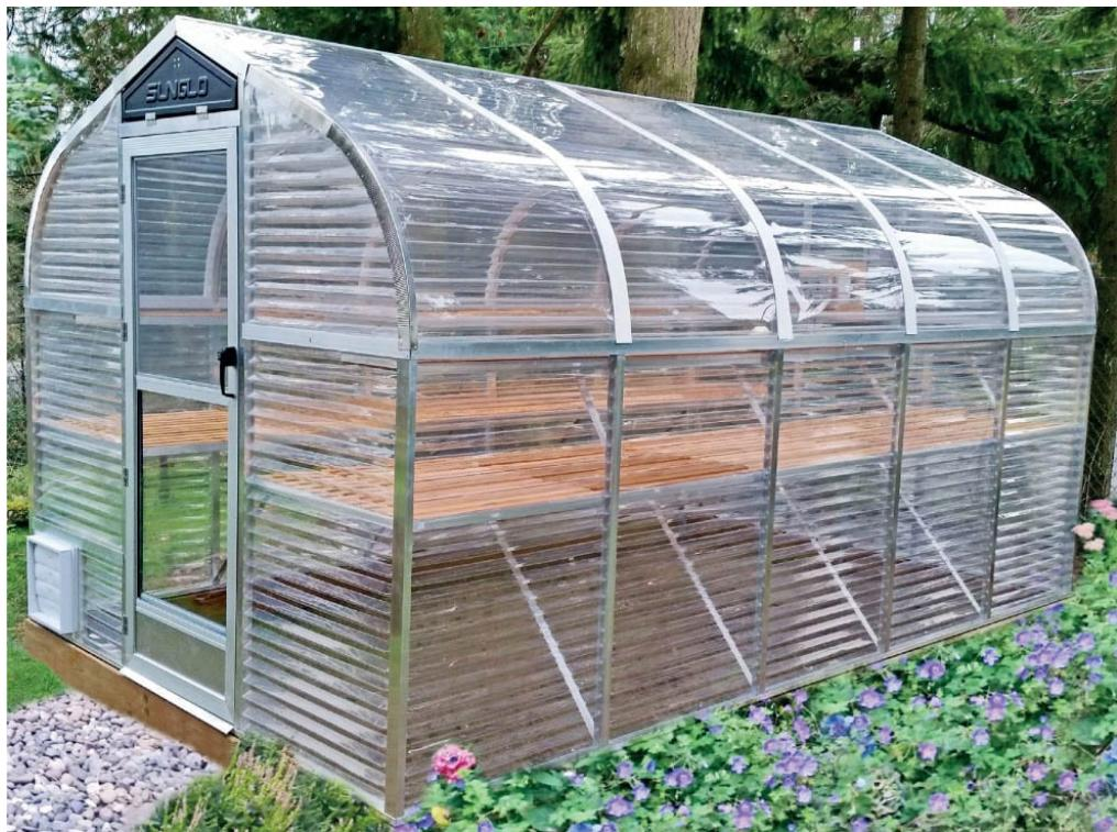
**Prep for greenhouse success.** This is another Gothic arch-style prefab greenhouse that has been set up for longevity and efficiency. It sits on a framed foundation, with a dirt floor that can be used for growing and is forgiving of spills or accidents. The slotted benches are ready to hold plants in need of sun and tender care, and the stone path ensures slip-free accessibility in any season.
