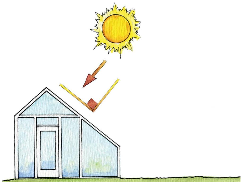
**For maximum heat gain**, orient your greenhouse so the roof or wall with the most surface area is as close to perpendicular to the sunrays as it can be.
