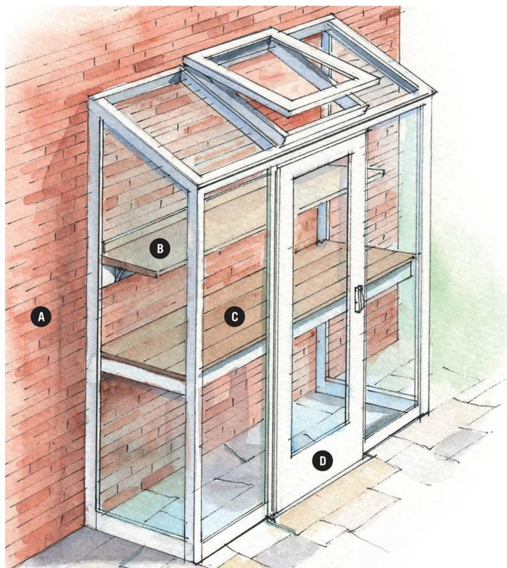
**A relatively inexpensive option** that requires little space, this greenhouse is typically made of aluminum framing and can be placed against a house, a garage, or even a fence, preferably facing southeast or southwest, to receive maximum light exposure. Space and access are limited, however; and without excellent ventilation, a mini-greenhouse can become dangerously overheated. Because the temperature inside is difficult to control, it is not recommended for winter use.
