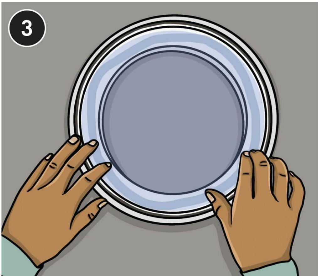
**Use scissors to cut** 6-mil plastic sheeting into panels that are  $\frac{1}{2}$ " larger on all sides than the windows in the bucket. Cut the circular window for the lid 1" larger in diameter than the opening. Use duct tape or silicone adhesive to fasten each window on the inside of the bucket and underside of the lid.
