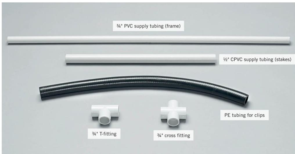
**Plastic tubing and fittings** used to build this hoop house include: light-duty 3/4" PVC tubing for the frame (do not use CPVC—it is too rigid and won't bend properly); 1/2" CPVC supply tubing for the frame stakes (rigidity is good here); polyethylene (PE) tubing for the cover clips; T-fittings and cross\* fittings to join the frame members.
