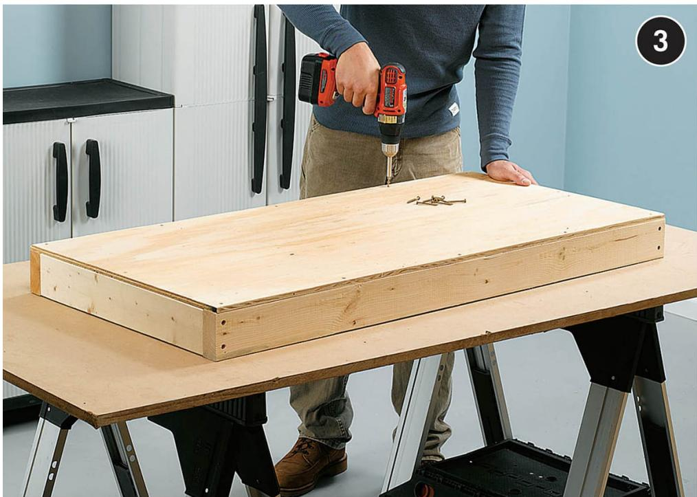
**Add the shelves.** Cut four shelves  $24 \times 48"$ , using a circular saw and straightedge cutting guide. Check each shelf frame with a framing square, then lay the shelf over the frame so it's centered side-to-side and end-to-end. Fasten the shelf to the frame with  $1\frac{1}{8}"$  deck screws.
