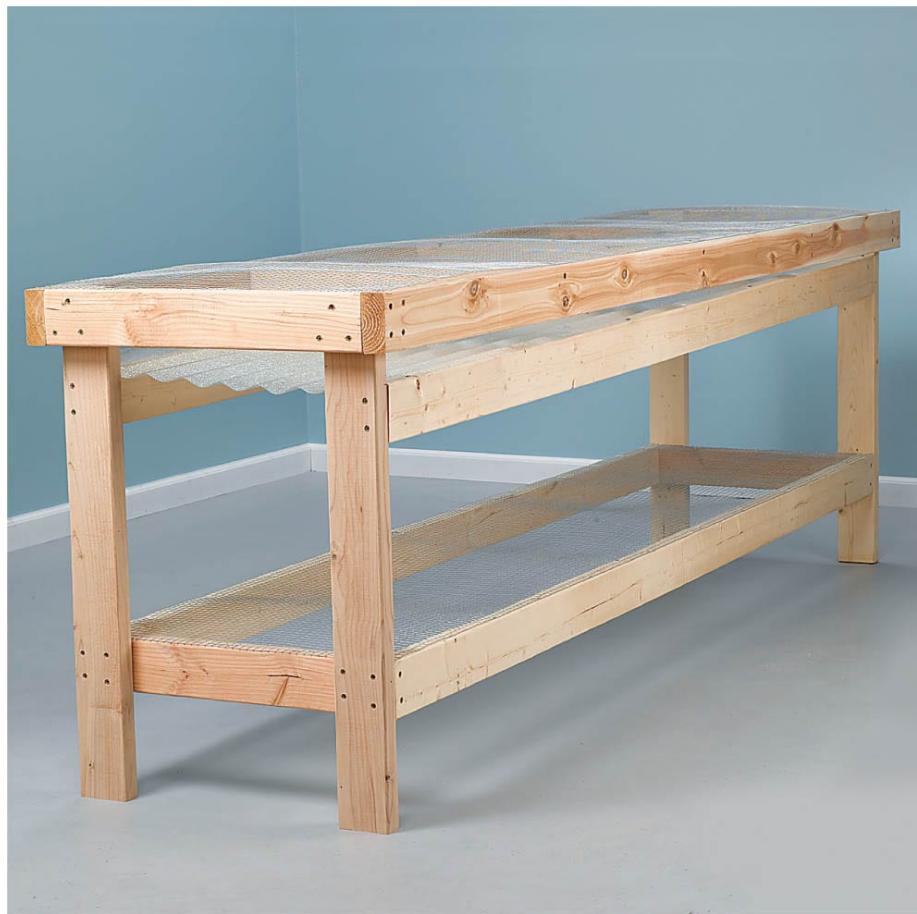
**Protect stored items from draining water** with a simple “roof” made with a single panel of corrugated plastic or fiberglass roofing. Use 2 × 4s between the leg pairs to support the panel, sloping the panel down toward one end at  $\frac{1}{4}$ ” per foot. Secure the panel at the top end with a couple of screws.
