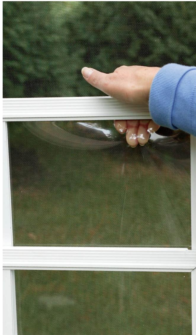
**Clear vinyl glazing** stretches under impact and will not shatter or crack. It is also light enough that sunroom kits often can be installed without structural reinforcement that may be required for units with glass-glazed windows.
