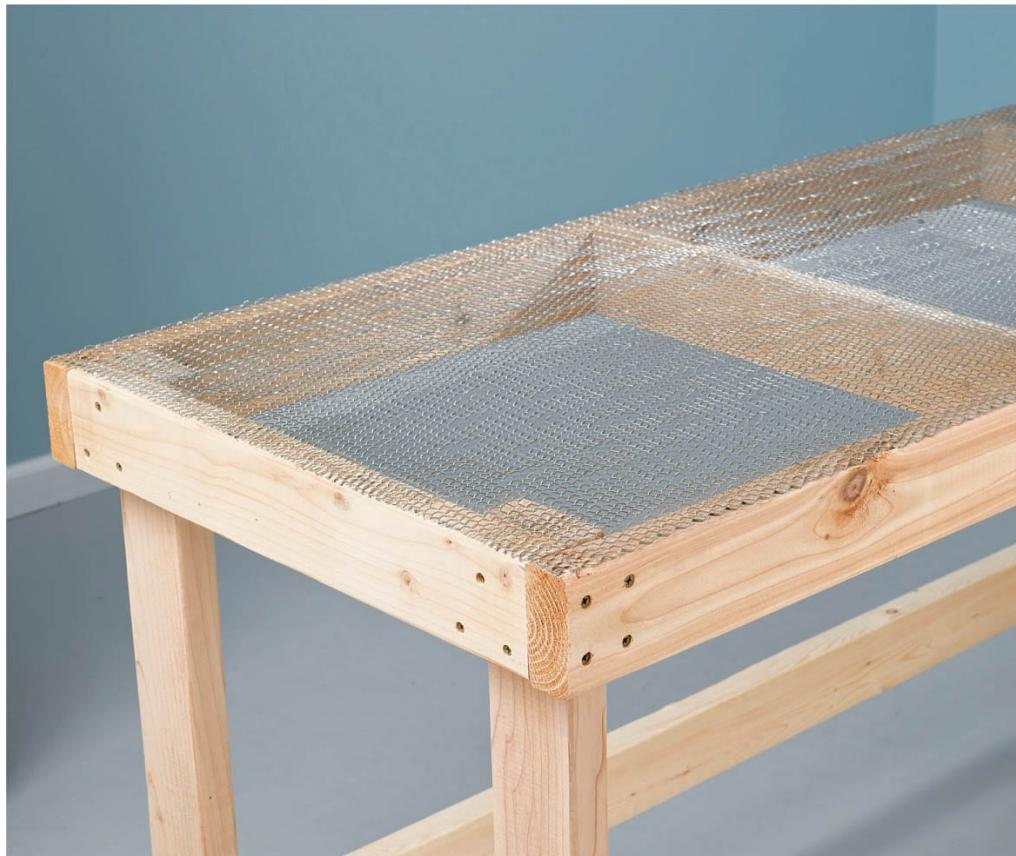
**Expanded steel mesh** is stiffer and has smaller holes than metal wire fencing, offering a more solid surface while maintaining permeability. Fasten steel mesh to the frame parts with heavy-duty staples or horseshoe nails. Do not use stucco lath, which has a rough surface and sharp steel edges.
