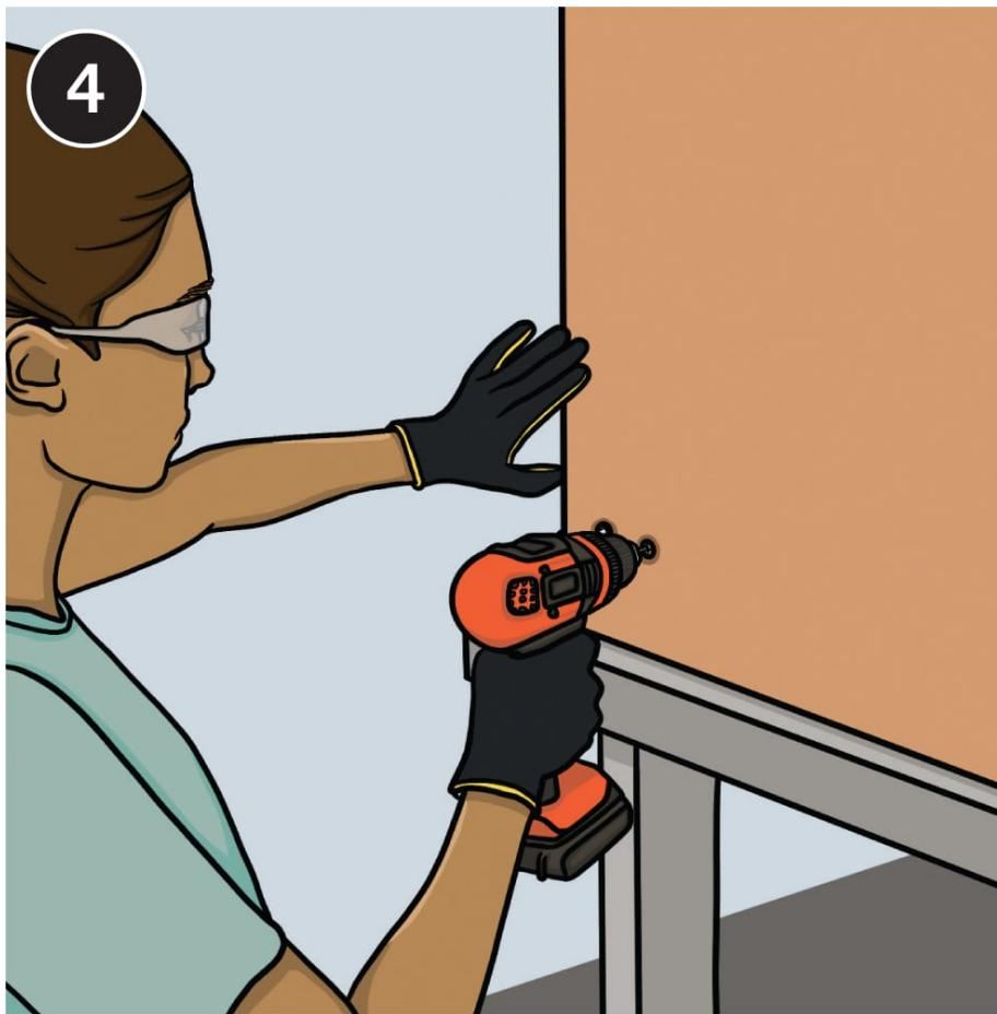
**Drill a random pattern** of  $1/16"$  or  $3/32"$  holes across the box floor, for drainage. Set the box frame on its side and screw the floor to bottom of each cleat.
