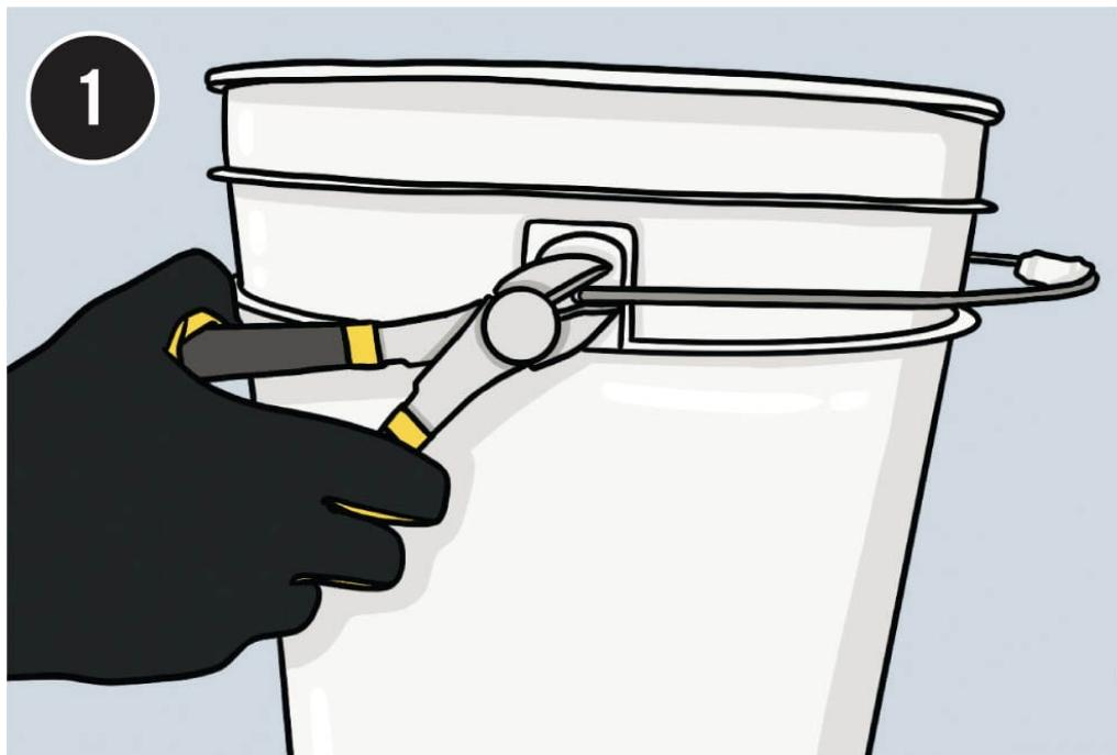
**Clean the bucket thoroughly.** Remove the bucket handle, by cutting each side where it goes into the bucket, with heavy-duty cutting pliers.
