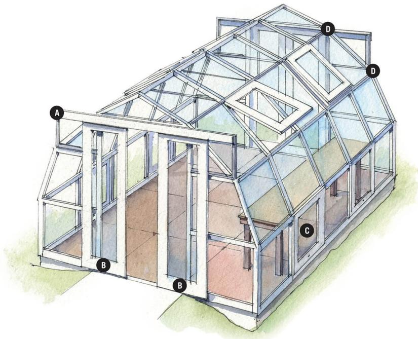
**The slanting sides and roof panels** that characterize the mansard are designed to allow maximum light transmission. This style is excellent for plants that need a lot of light during the winter. The downside is that this type of construction takes up a lot of room and can be an expensive greenhouse to build.
