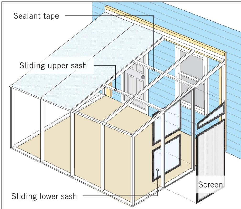
**Sunroom kits with plastic panels** can be mounted on practically any hard surface because they are light enough that they do not require a reinforced floor. You do need to make sure the floor is level, however, and that the base channels you lay out create square corners.
