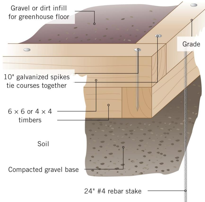
**Timber foundations** are simple frames made with  $4 \times 4$ ,  $6 \times 6$ , or larger landscape timbers. The timber frame is laid over a leveled and compacted gravel base (which can also double as the floor or floor subbase for the greenhouse interior) and pinned to the ground with rebar stakes. One level, or course, of timbers is suitable for small greenhouses, while two courses or more are recommended for larger structures.
