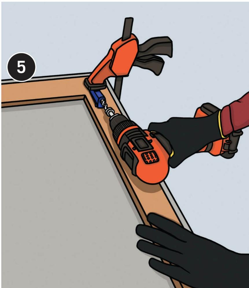
**Cut and rip two window frame rails**  $2 \times 36"$ , from deck boards. Cut and rip two stiles  $2 \times 21\frac{1}{2}"$ . Lay out the frame on a flat, level work surface with the longer rails butted to the inside of the stiles. Measure the diagonals to ensure square, and clamp the pieces to the work surface. Drill pocket holes in the rail faces using a pocket jig. Screw the frame together using  $3"$  wood screws.
