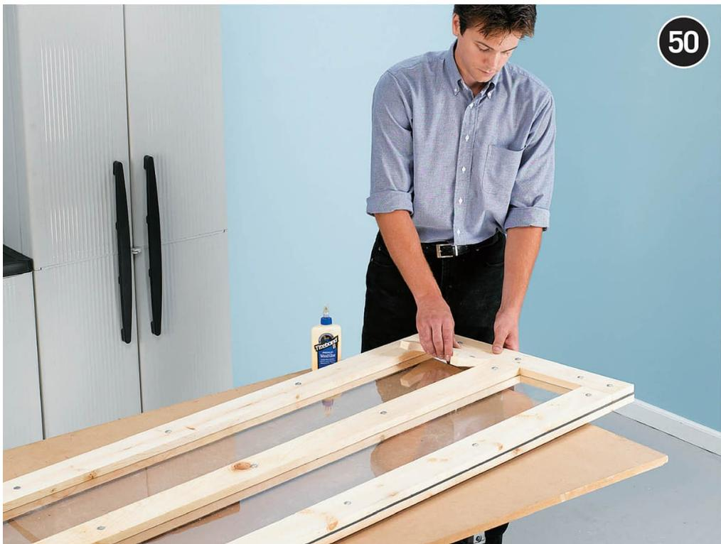
**Cut the door panel inserts with a jigsaw** and sand them smooth. Insert them into the framed openings as shown in the diagram on [this page](#). Secure them on both sides of the glazing, using glue and brads or pin nails. Paint the door frame before installation and touch up after.
