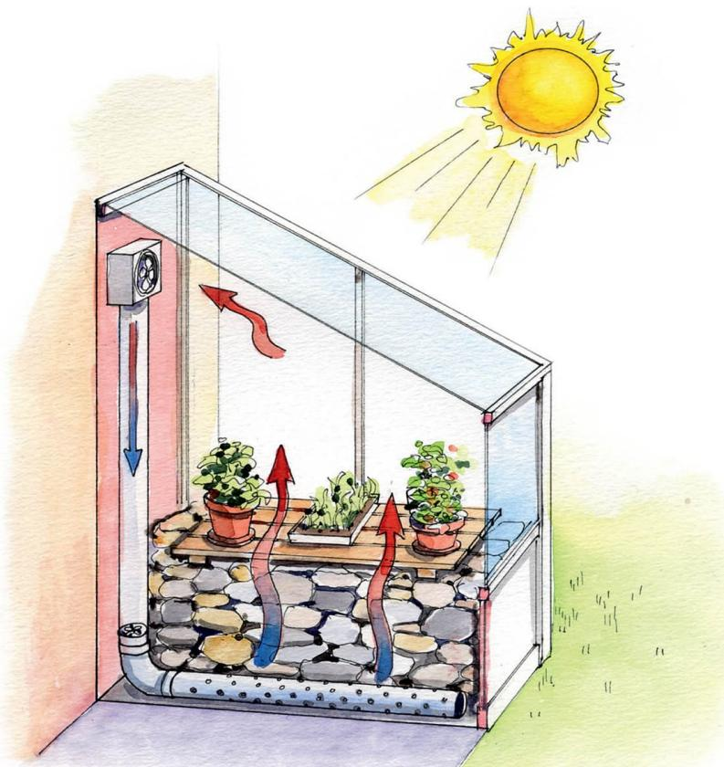
**This heat sink system** uses solar energy to heat the greenhouse. Air heated by the sun is drawn in by the fan and blown into the rock pile, which also absorbs solar heat. Heat is radiated back into the greenhouse after the sun goes down.
