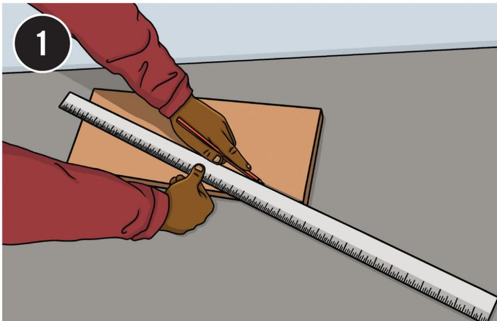
**Saw four 4 × 20" side-panel boards** from the pallet deck boards. Saw two 6 × 20" side-panel boards for the top of each side. Measure and mark these boards for trapezoid cuts from one corner to 1" above the opposite corner using a metal straightedge or 4' level. Cut each top board to the angle marked.
