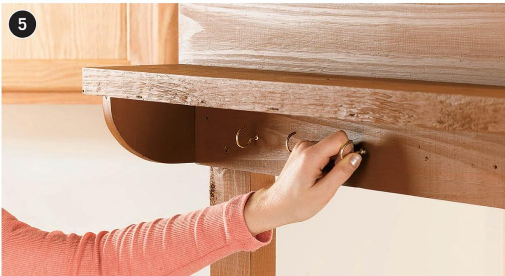
**Attach the shelf** back, shelf hook rail, and shelf supports to the long leg and back strut with 2½-inch deck screws. Attach the shelf to the shelf supports with 2-inch deck screws. Fasten the hooks to the shelf hook rail.
