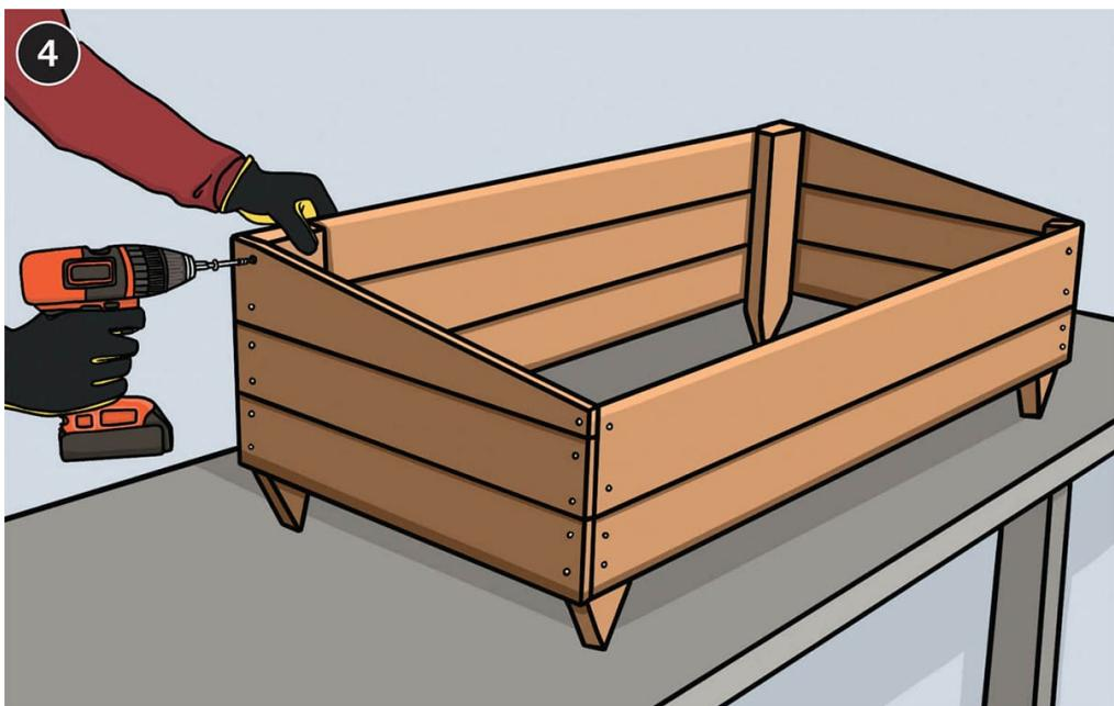
**Screw the wide end** of the triangular top boards to the back wall stakes. Drill pilot holes and screw the front, narrow ends to the front wall stakes.
