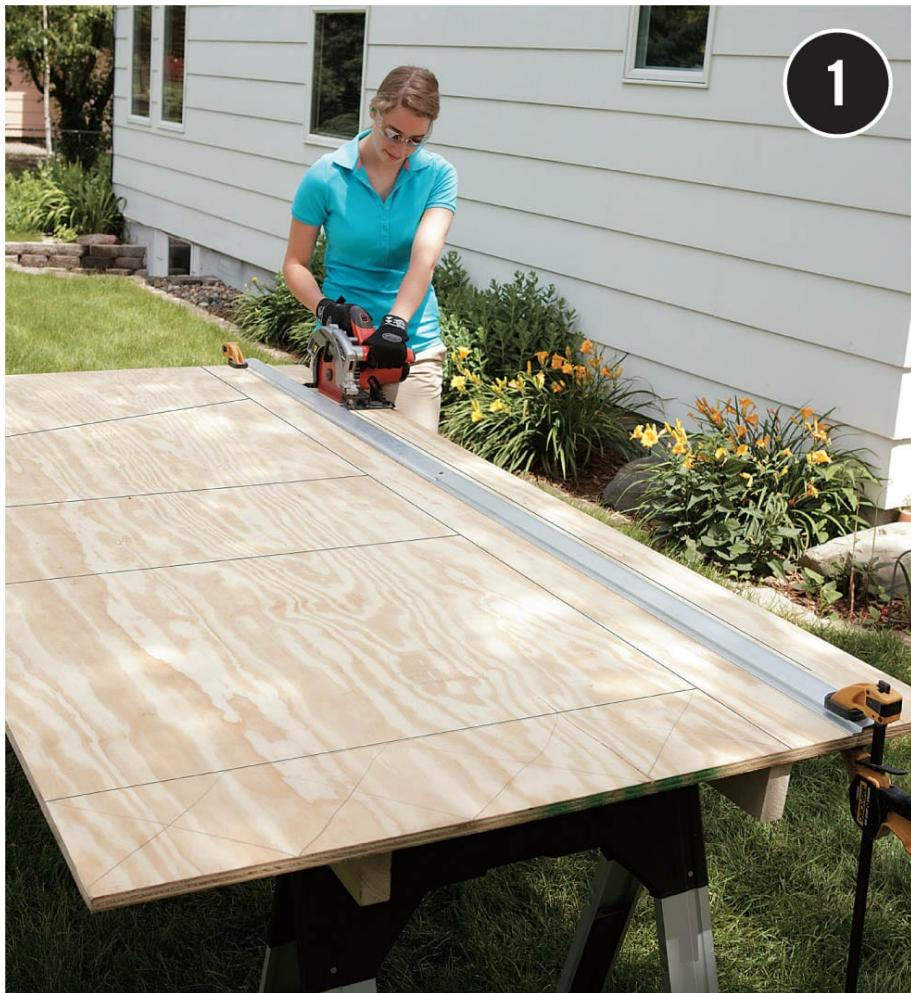
**Cut the parts.** This project, as dimensioned, is designed to be made entirely from a single 4 × 8 sheet of plywood. Start by cutting the plywood lengthwise to make a 36"-wide piece.
