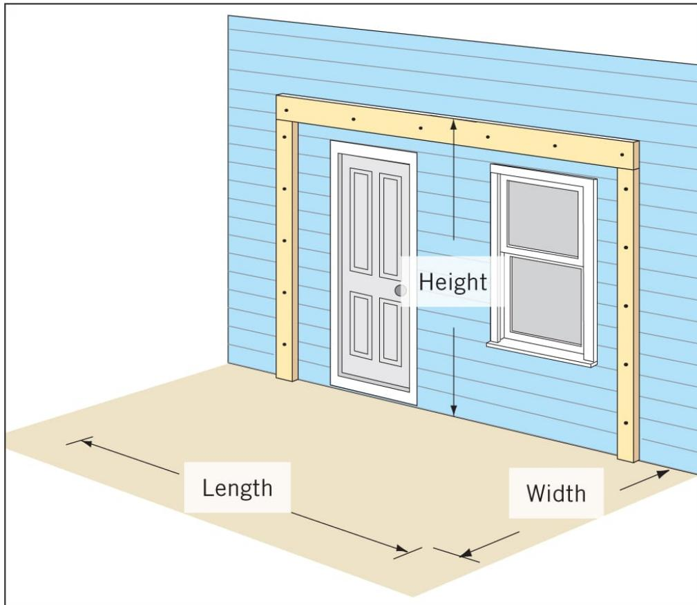
**Attach a sunroom to an exterior wall** by fastening a  $2 \times 6$  or  $2 \times 8$  horizontal ledger at the sunroom's roof height. Fasten  $2 \times 4$  vertical side cleats under either end of the head cleat.
