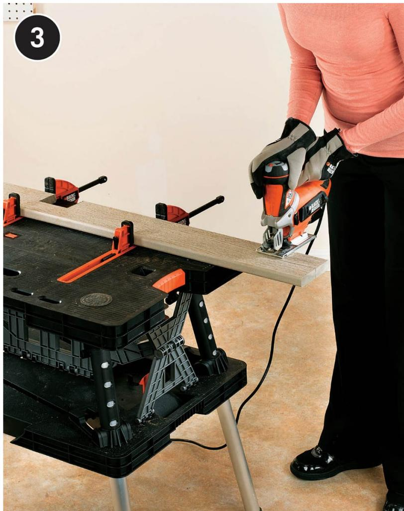
**Cut the composite deck boards** for the work surfaces. Place the front deck board for the lower work surface against the backside of the front left leg and front strut. Mark the point where the front leg and strut intersect the deck board. Using these marks, draw the  $3\frac{3}{4}$ " deep notch outlines and cut out the notches with a jigsaw.
