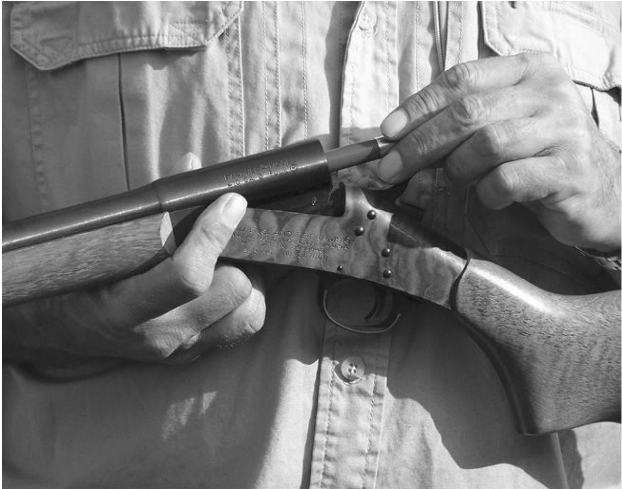
Break-open shotguns are the easiest to load, unload, and check. This is a New England Firearms .410 single-shot.
