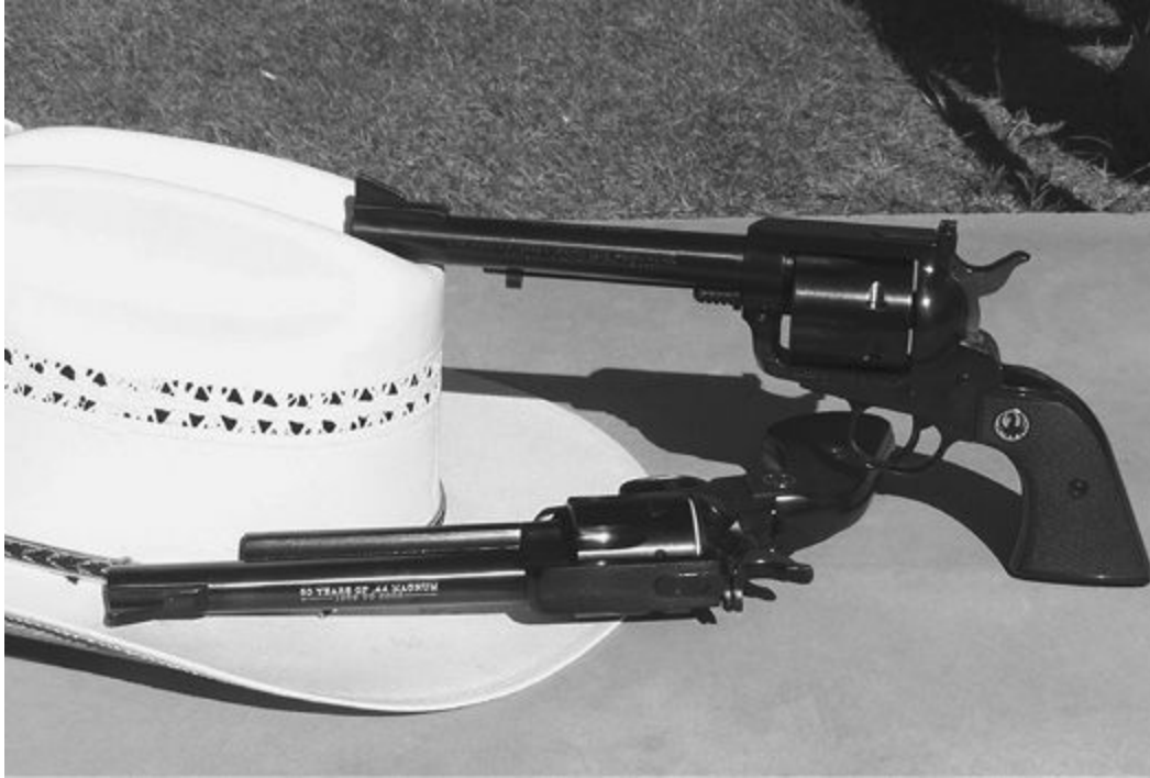
Single action revolvers like these operate differently from the more commonly seen double action designs. This is author's pair of Ruger Blackhawk .44 Magnums.
