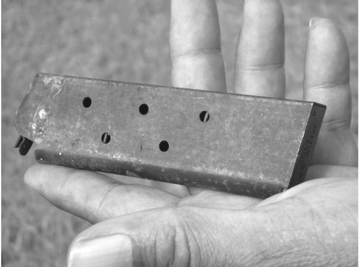
Badly rusted, this neglected 1911 .45 magazine is no longer reliable.
