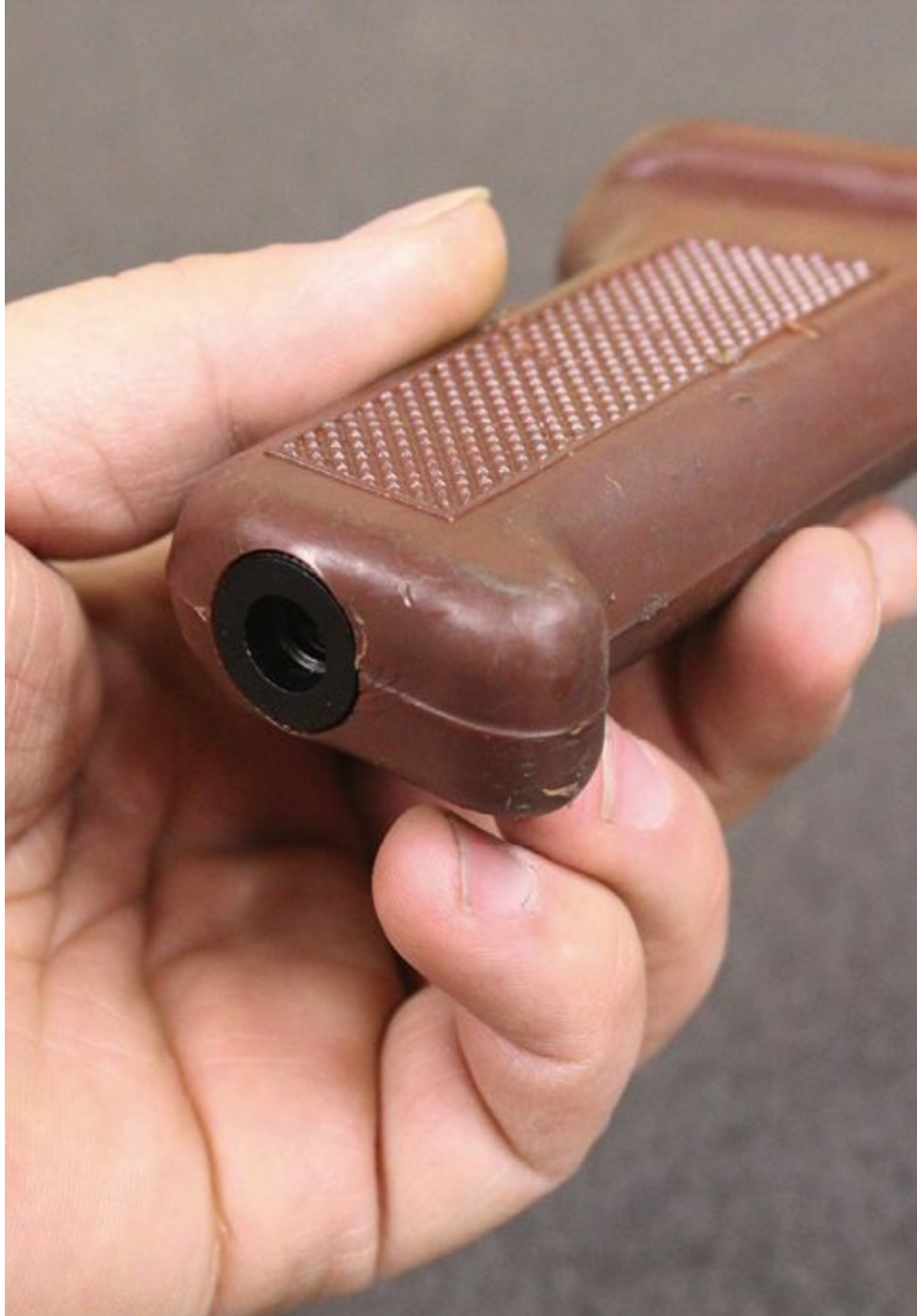
AK grips are also retained by a single screw.
