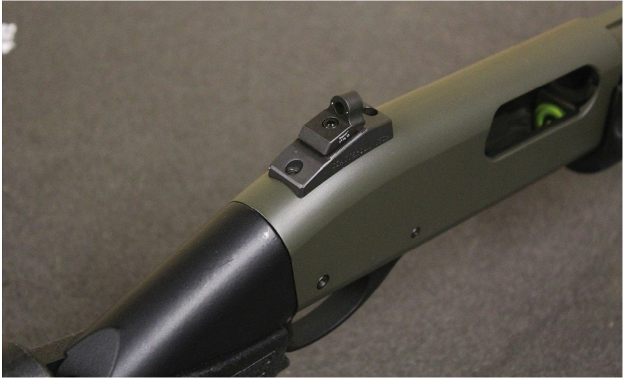
Ghost ring rear sight from Scattergun Technologies/Wilson Combat mounted on the back of a Rem. 870. It is adjustable for elevation and windage and includes Tritium vials, as does the epoxy front sight.
