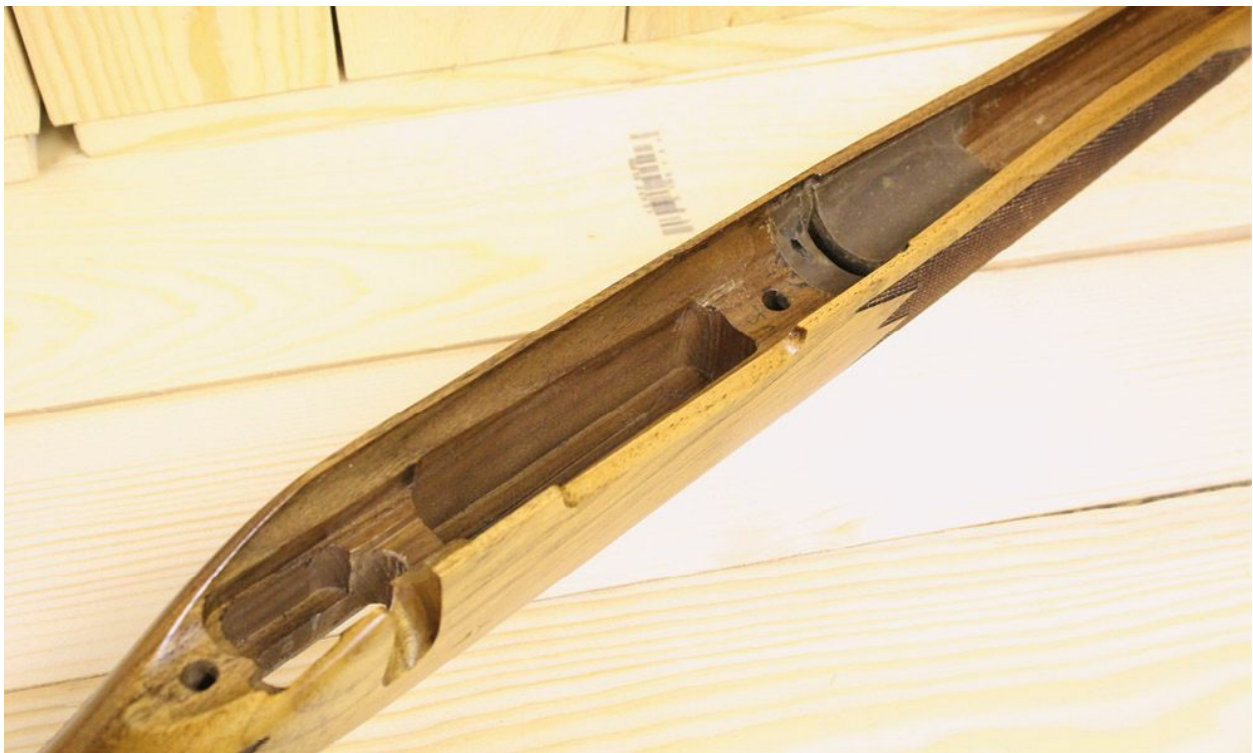
The inside of a Rem 700 wooden stock. Compare it to the synthetic stock.
