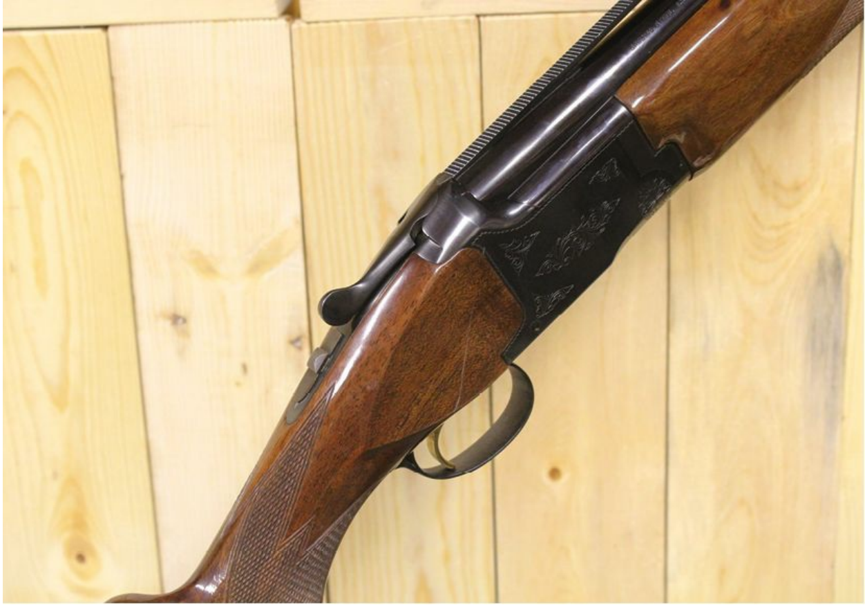
A two-piece stock where the stock and forend are separate pieces, and the pistol grip is integrated into the stock.
