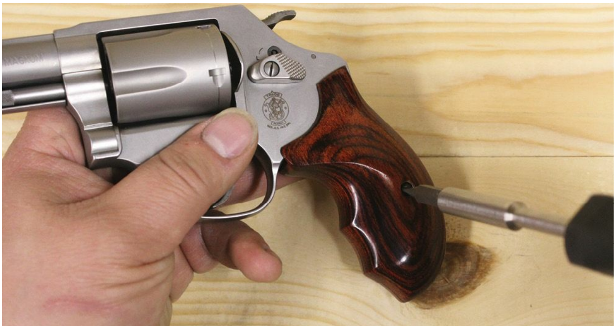
The single grip screw can be removed simply.
