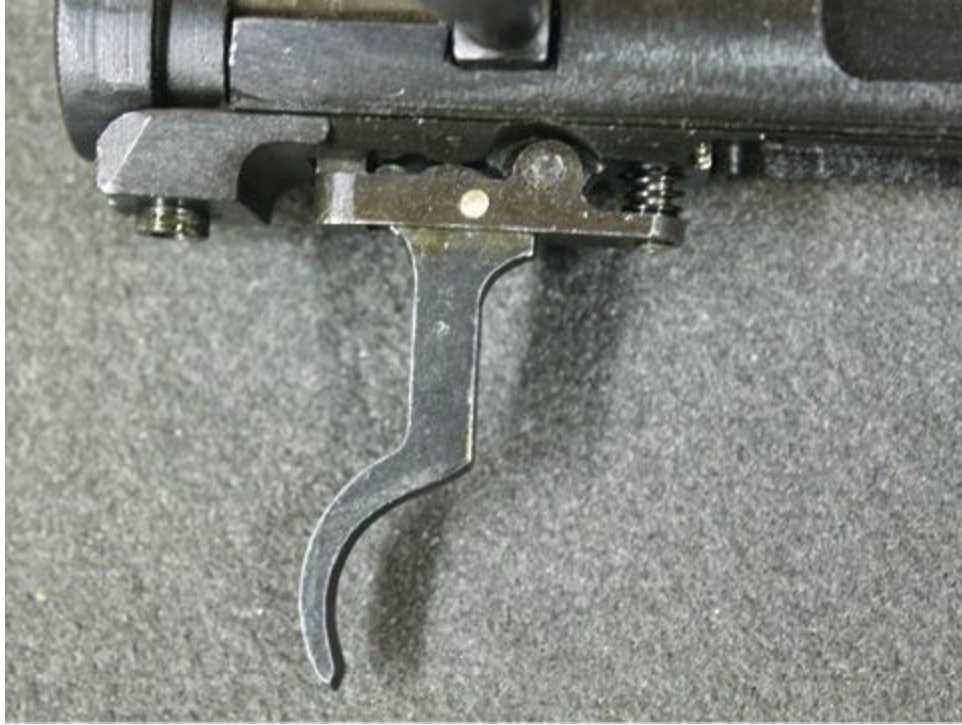
Old Mauser style direct action trigger from an Arisaka rifle. Pulls were long and heavy.
