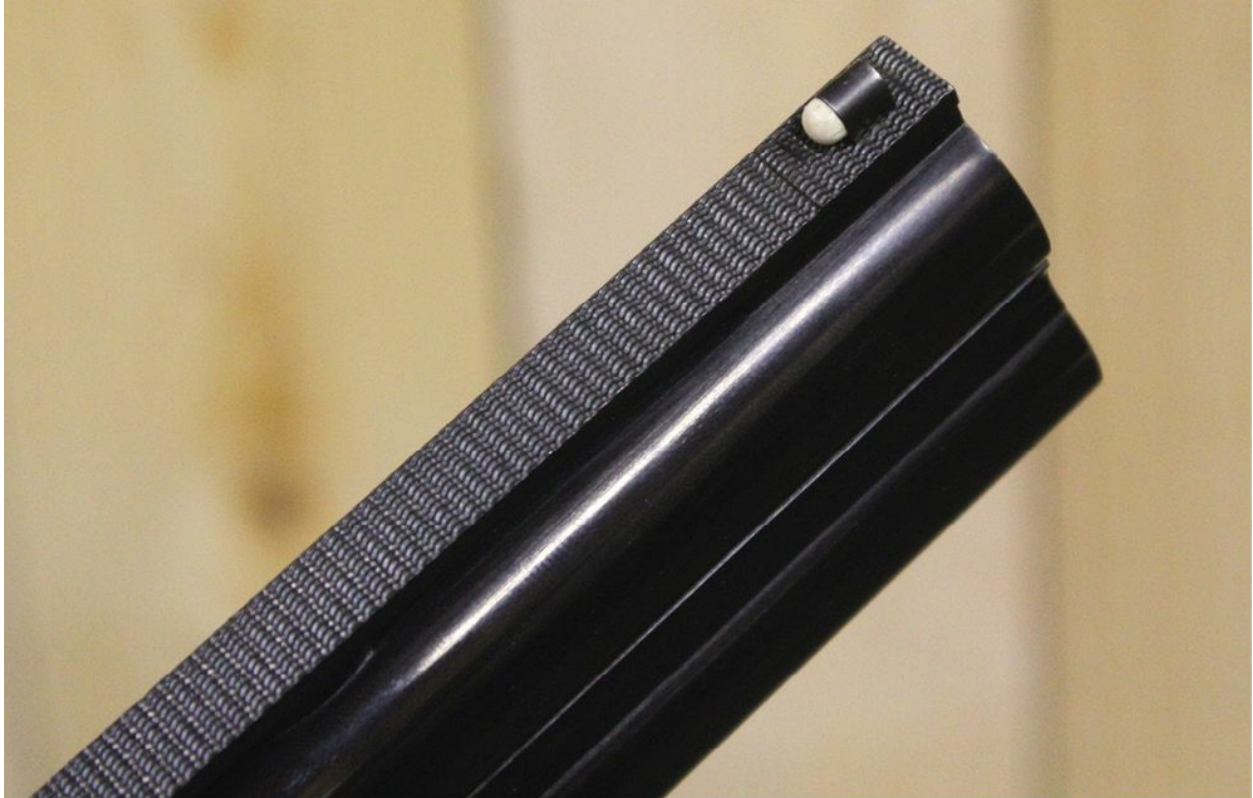
Typical 21st-century front bead. Steel housing with white plastic easy-see insert.
