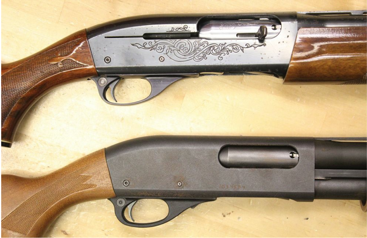
The Remington 1100 and 870 shotguns use many similar or same parts. The receivers are different, for example, but are very alike in appearance and styling. The 1100 is semi-automatic and the 870 is a pump gun.
