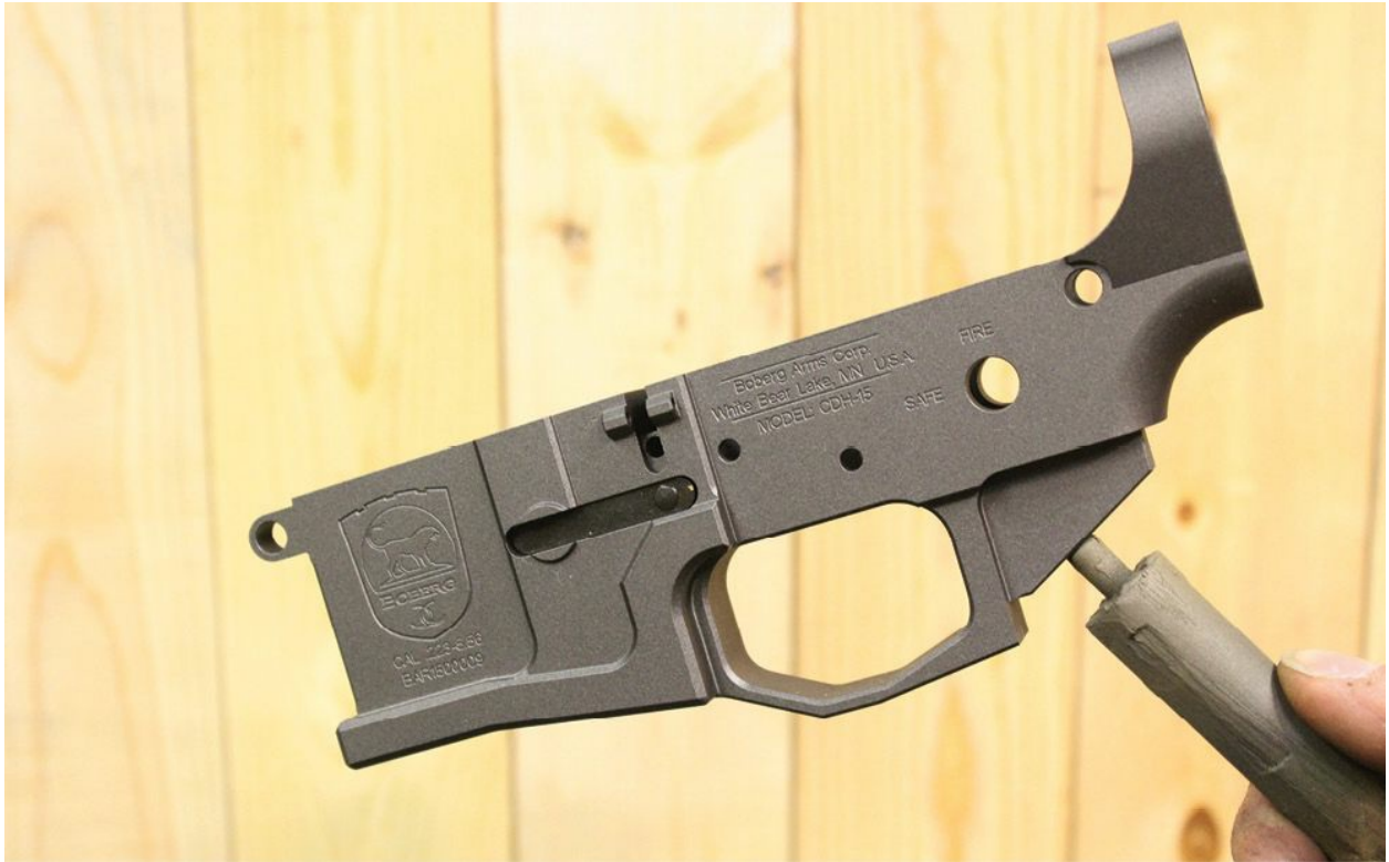
The same concept of fixturing is used on the lower receiver. Use the design to your benefit. In this case, a ¼-28 bolt was glued to a ½-inch wood dowel. The bolt is screwed into the pistol grip screw hole.
