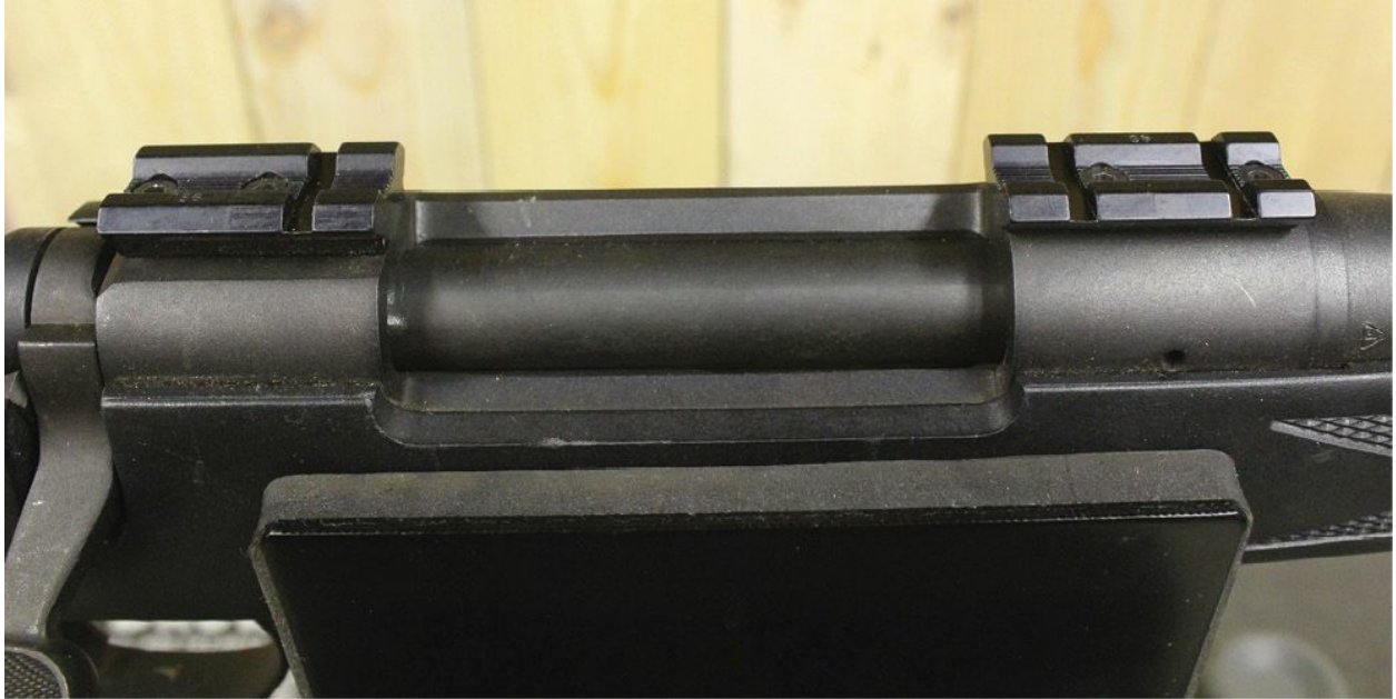
These Weaver mounts offer a choice of mounting points. Extension rings will make this flexibility even greater.
