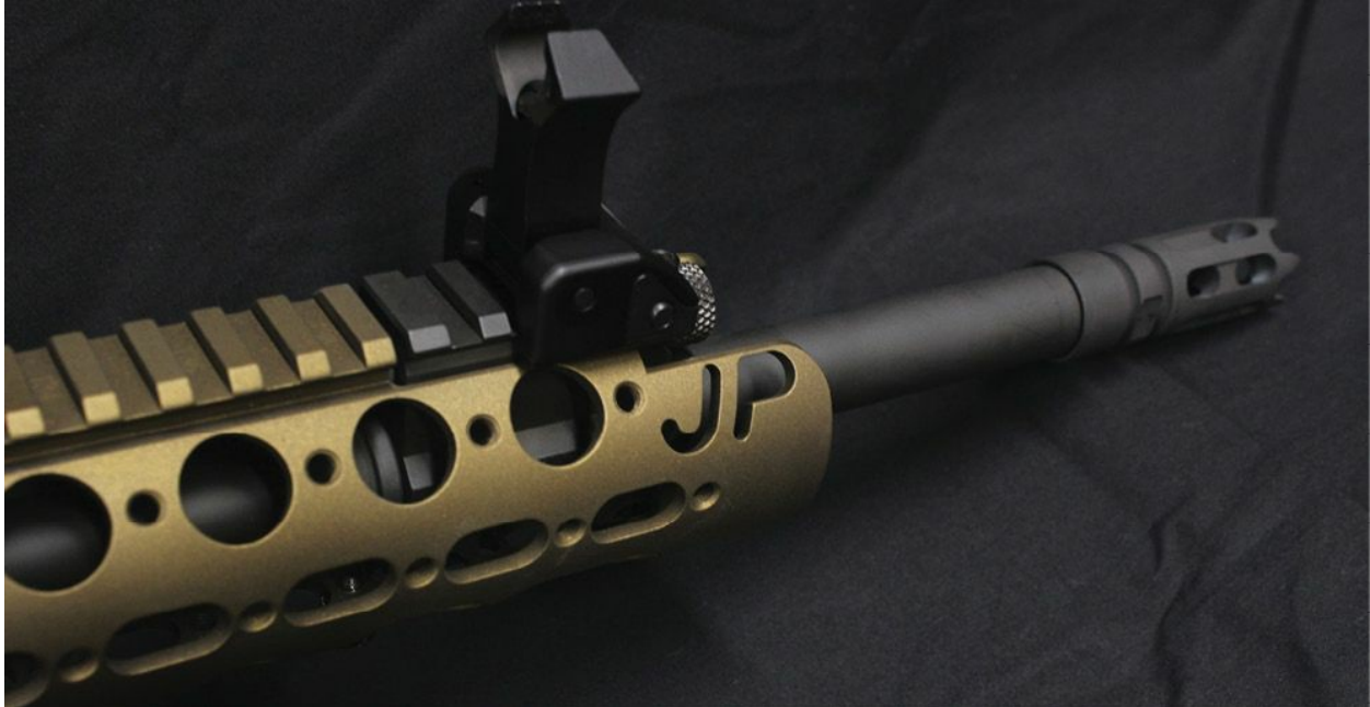
A piston upper using a JP tube and Adams Arms Piston upgrade. Cerakote Burned Bronze color.
