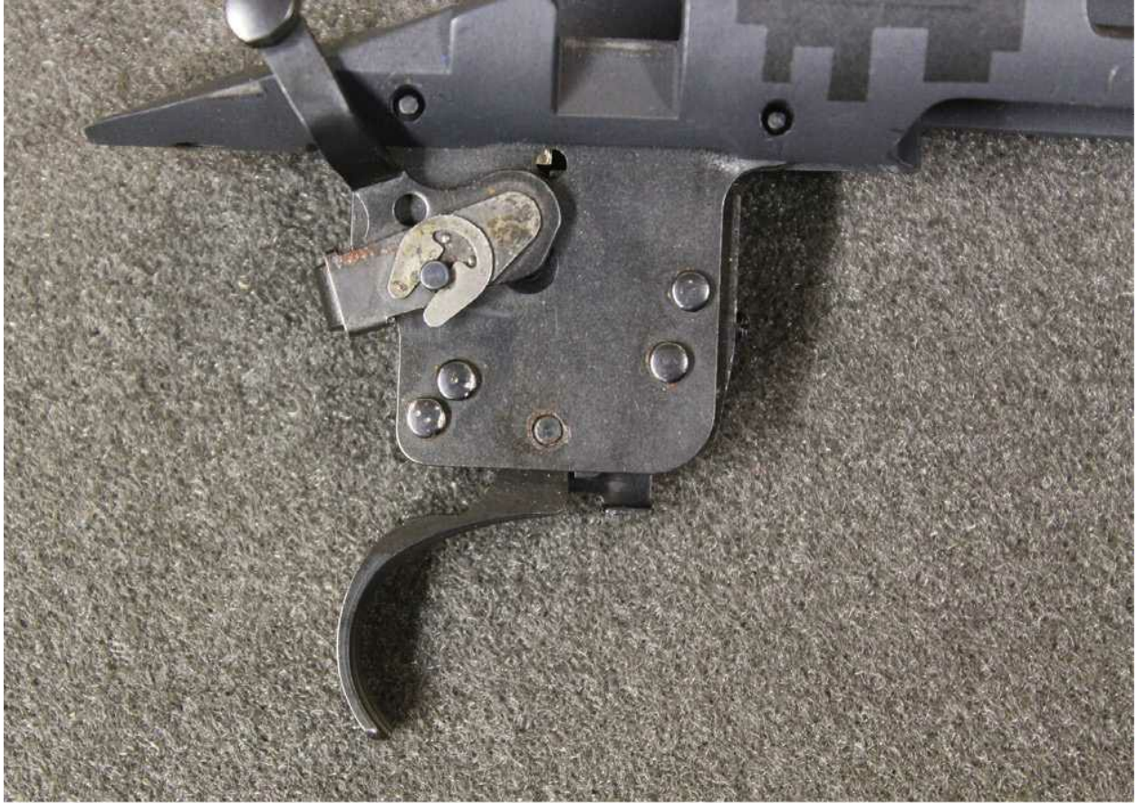
An old-style Remington 700 trigger with a bit of rust, awaiting replacement
