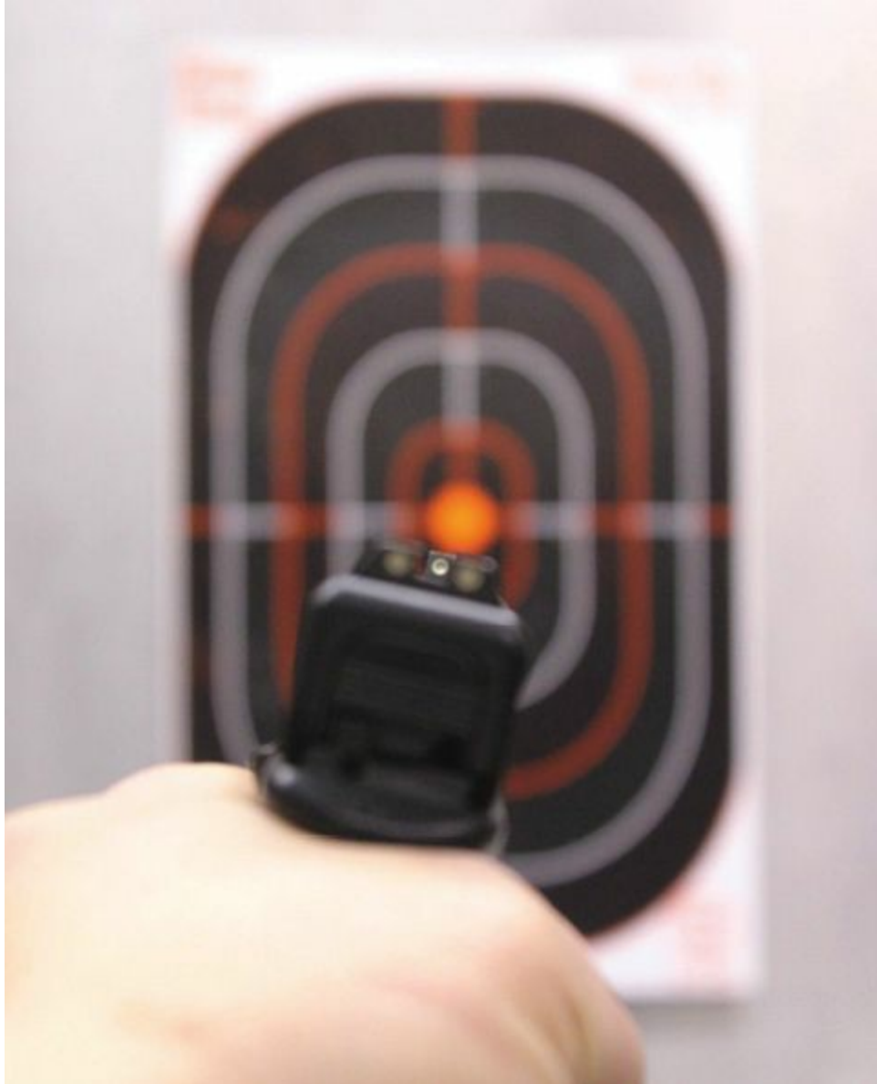
Very common three dot type of sight used on most handguns.
