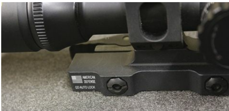
The right side of the ADI mount showing the adjustment bolt heads. Turning these octagonal screws clockwise will tighten the tension when the lever has been closed. This is to be able to adjust to any rail that it is mounted on.
