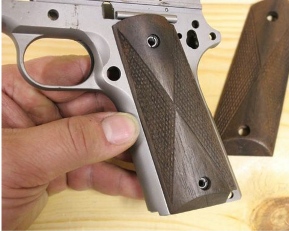
I made these grips using a fixture made from a cut-off barrel spud. They look okay and worked great, but I didn't reinforce them. There is a crack at the bottom.
