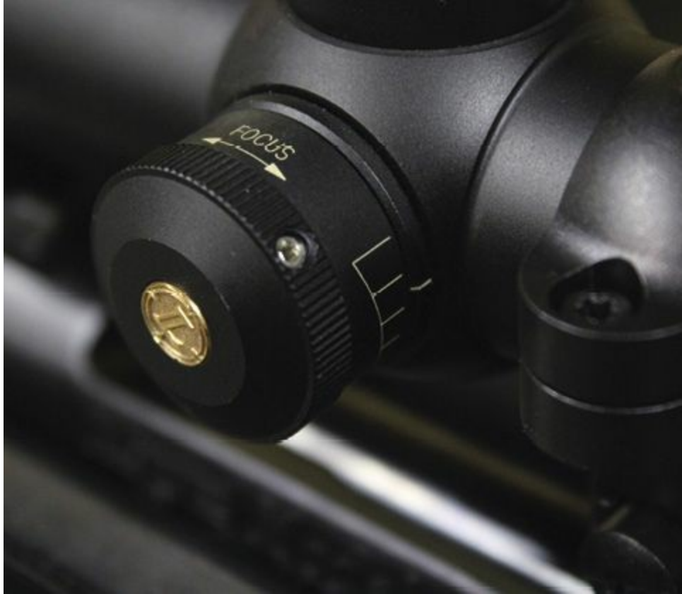
This Leupold varmint scope has a side parallax adjustment.
