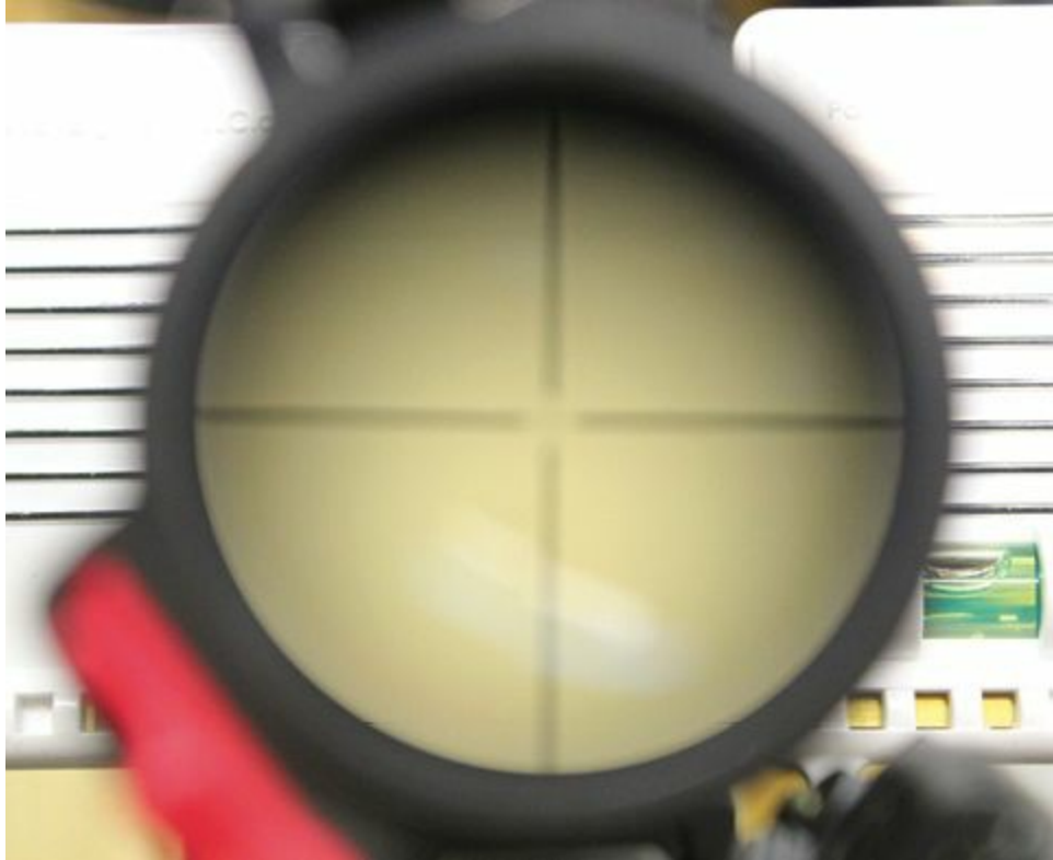
The Segway reticle leveler at work. The scope is canted to the right.
