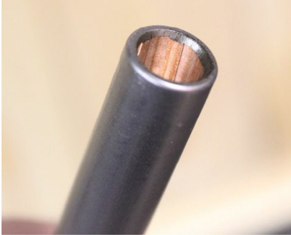
The standard cut rifling in an FNS-9 barrel. The intersections between the lands and grooves are sharp and square.
