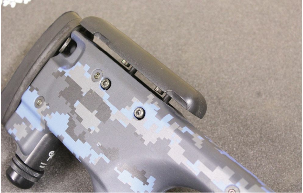
The AICS has an adjustable comb, for height and for left and right motions.
