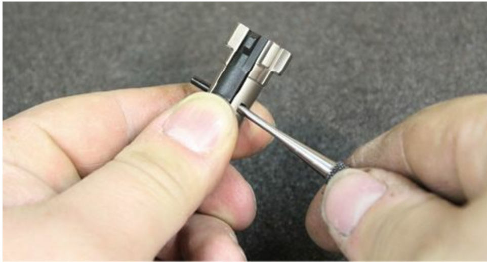
Remove the extractor by pushing out this pin.
