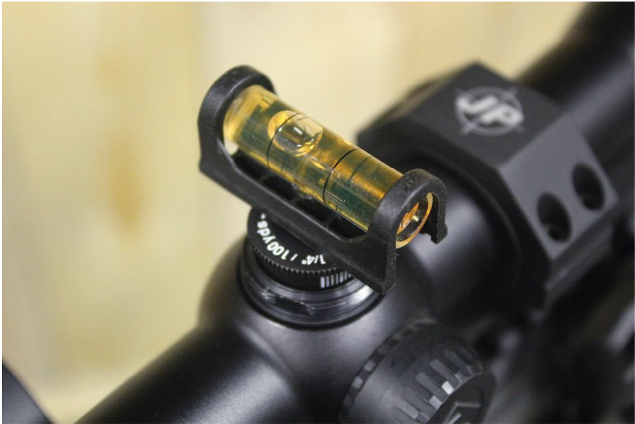
A level mounted on the turret of a scope for boresighting purposes.
