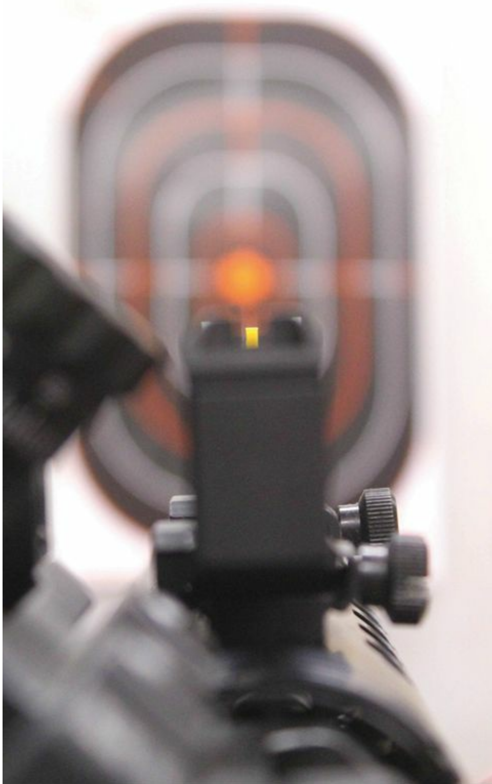
The JP SRTS on line with the target. It is used for close shots that would be difficult to engage quickly with the primary optic.
