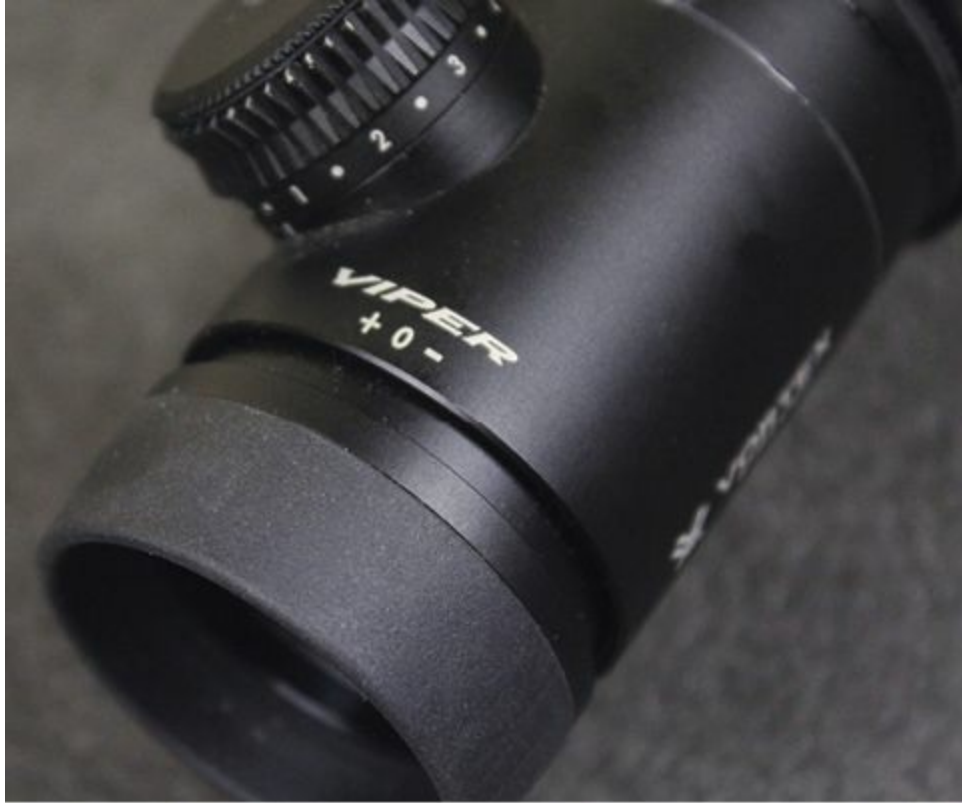
The diopter adjustment on the ocular end of the rifle scope. The + and – gives it away.
