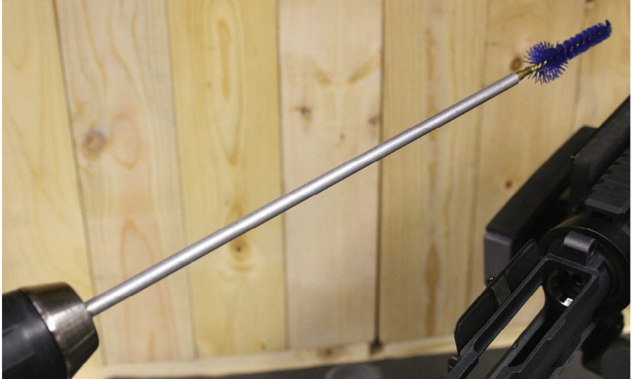
A brush on a rod in a hand drill. Good for spinning in chambers.
