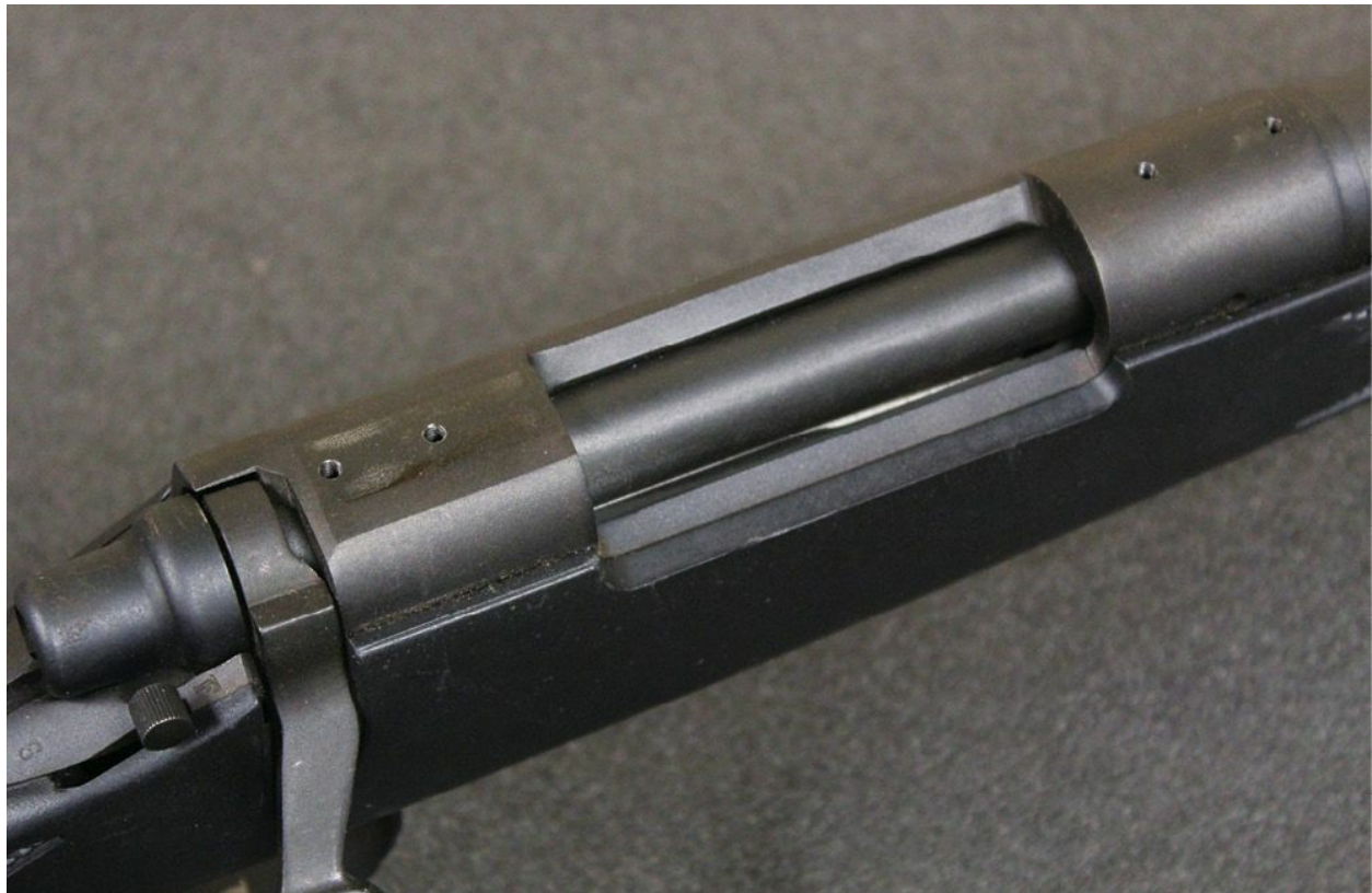
When you see holes like this on a receiver, it is just begging for an optic.
