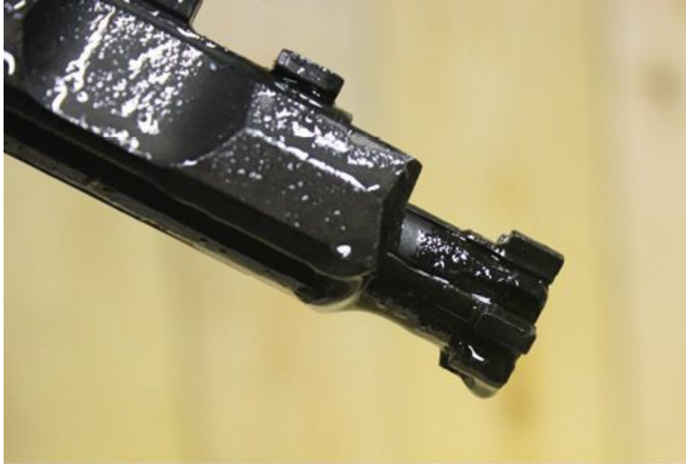
AR bolt carrier assembly, wet, properly lubricated.
