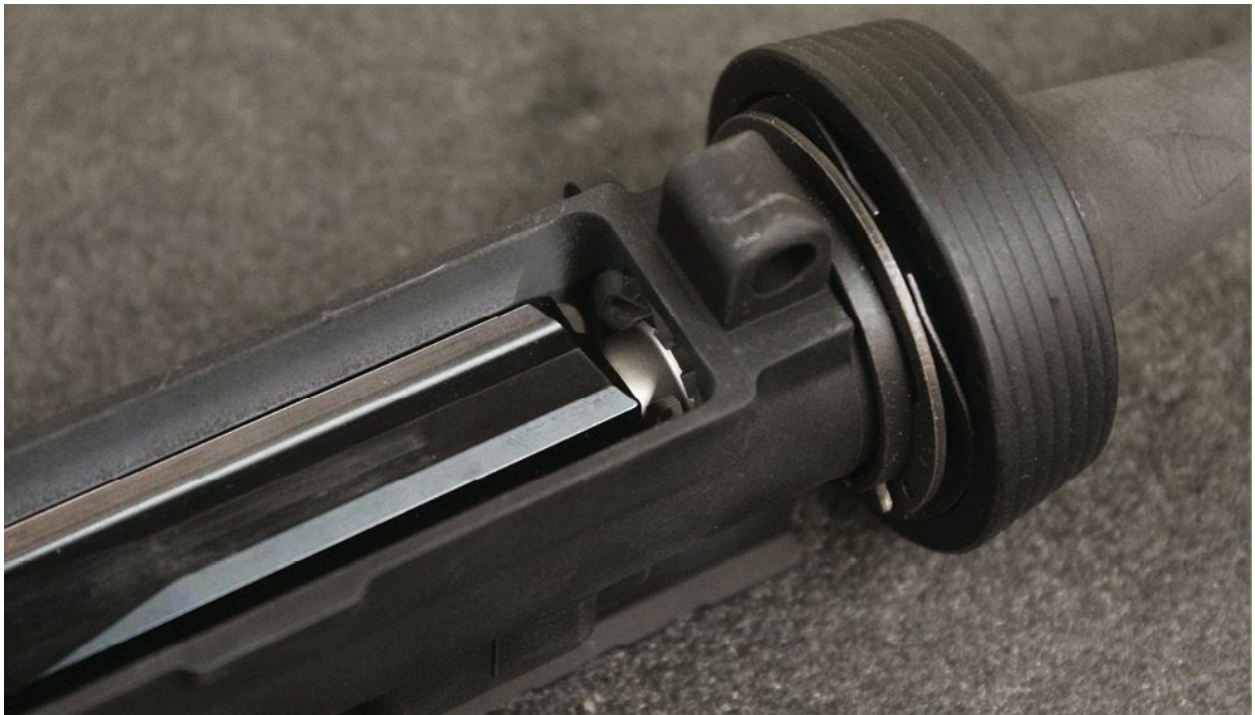
The NOGO gauge is in the chamber and the carrier is not fully closed.
