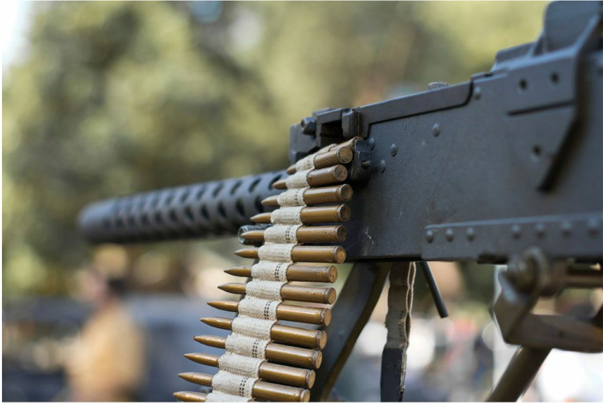
Machineguns mostly used belts to feed the guns, like this Browning M1919.
