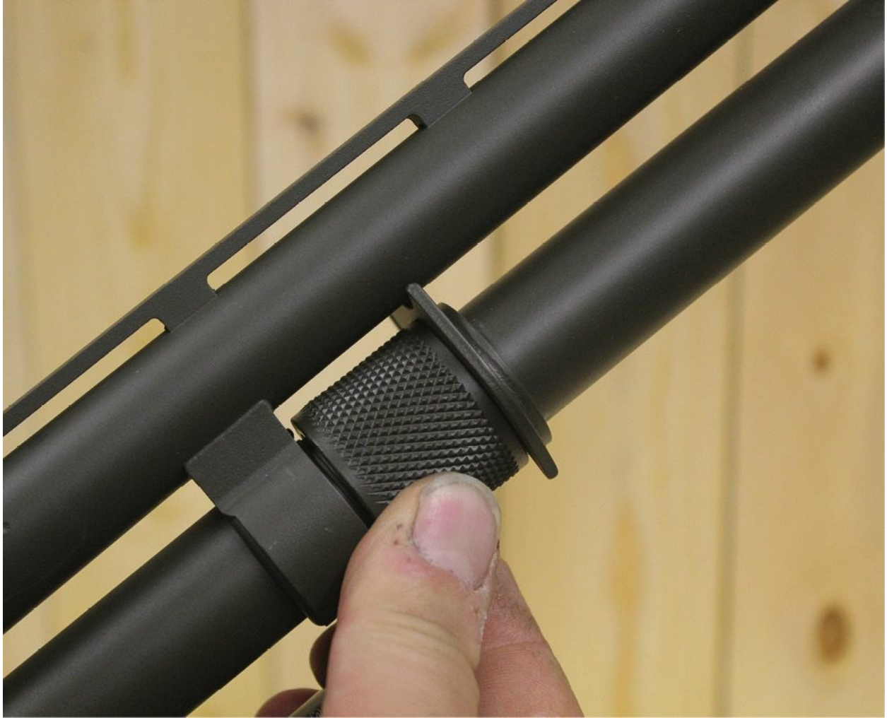
Unscrew and remove the magazine tube cap.
