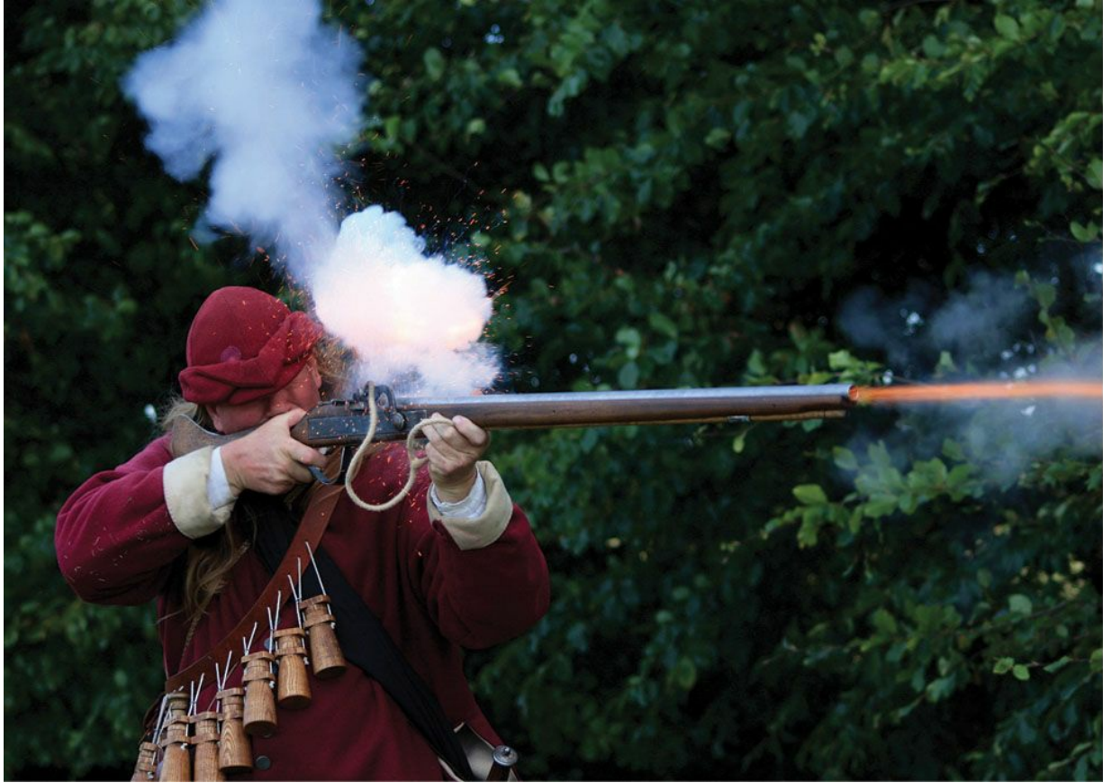
A reproduction matchlock musket being fired. The trigger is a simple lever that allowed the match to be lowered into the flash pan, igniting the powder. No fun at all.
