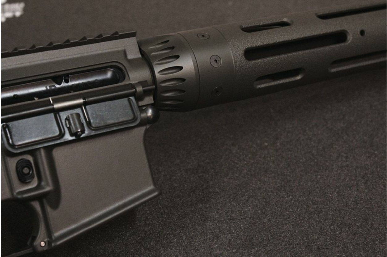
A MagPul OD Green AR. The upper and lower receivers along with the handguard are painted.
