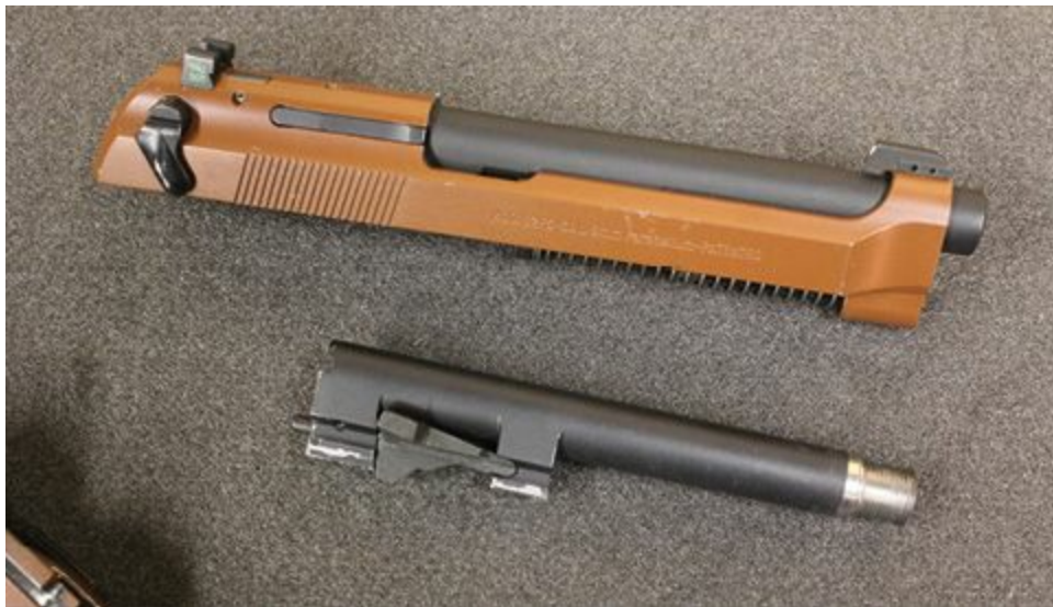
An aftermarket threaded barrel next to a Beretta 92 slide. An additional locking block and pin needed to be procured to place in the rear lug of the barrel.
