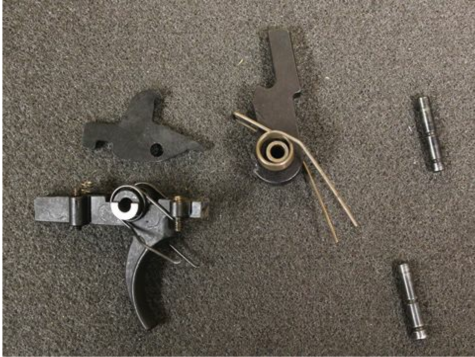
A JP Enterprises Match trigger with speed hammer. These are usually available with anti-walk pins as well.
