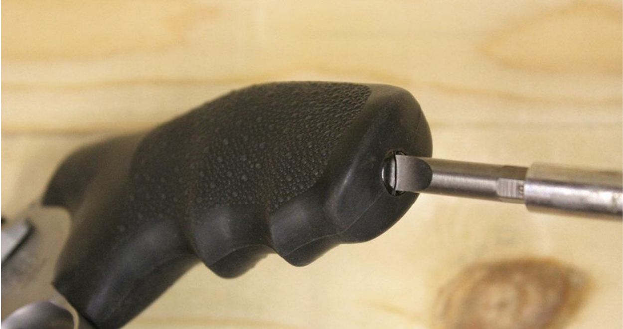
Slide the Hogue grip onto the frame.
