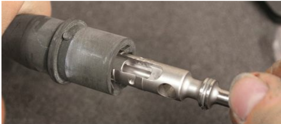
Headspace should be determined, if possible, before the barrel is installed.
