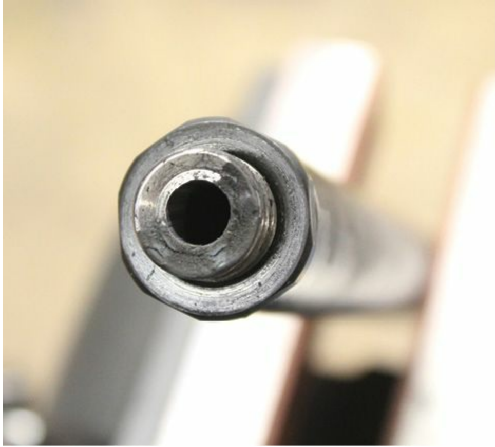
Starting to remove the false crown.
