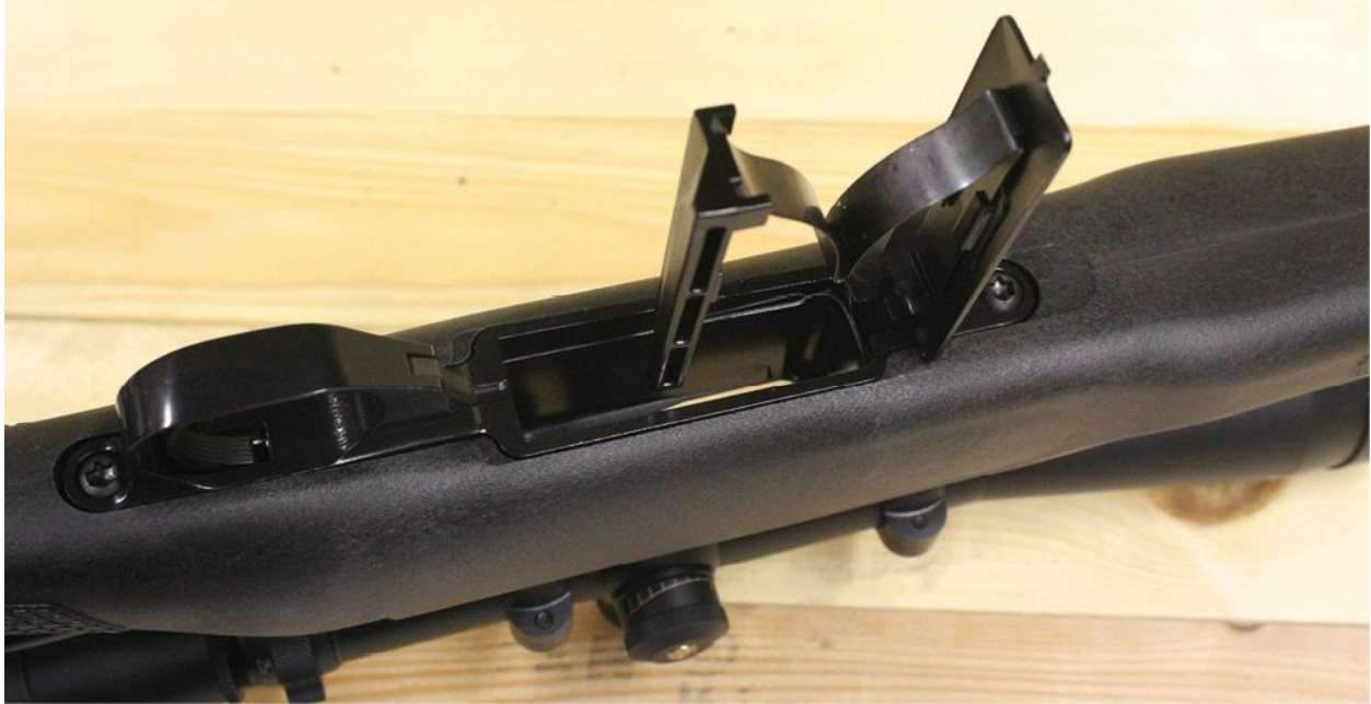
Internal blind box magazines soon gave way to internal magazines with removable or pivoting floor plates.
