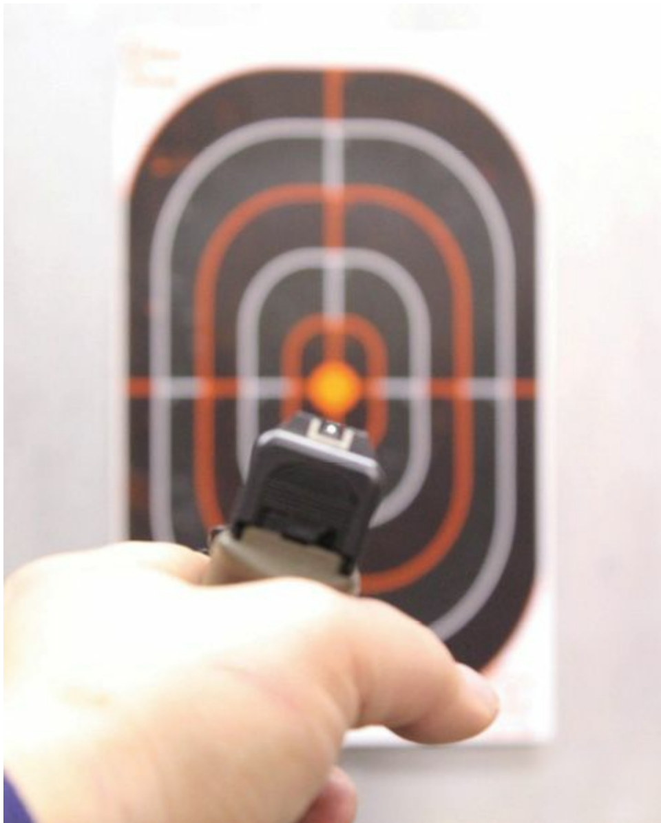
Glock sight picture with factory white line notch in rear.
