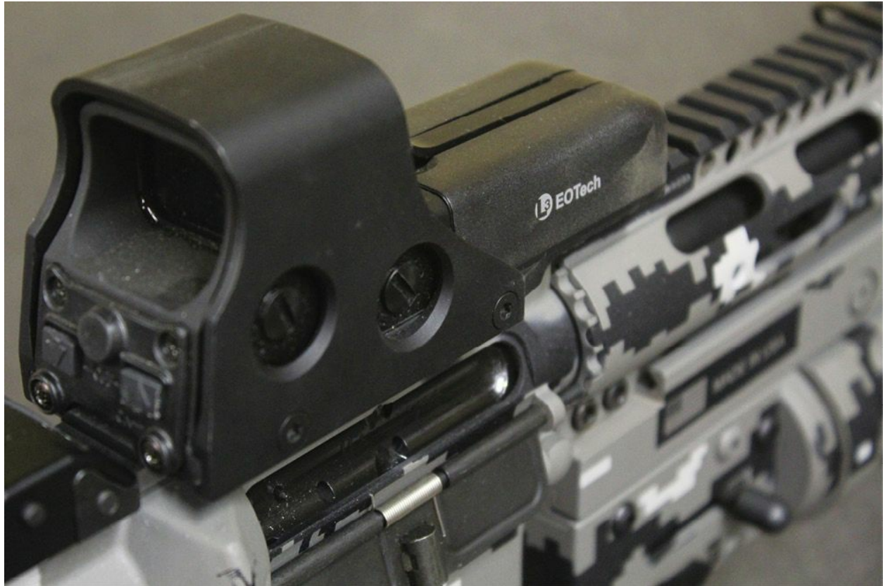
The EoTech Holographic Sight uses a circle dot reticle. It uses holographic technology rather than a red diode.
