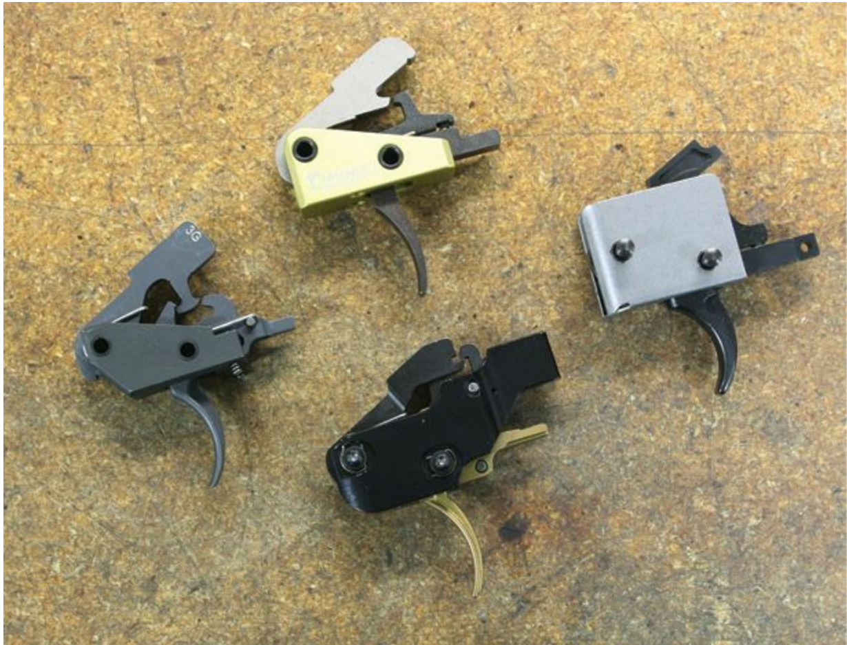
This is the standard trigger, hammer, disconnector of an AR-15 that comes in most factory rifles.
