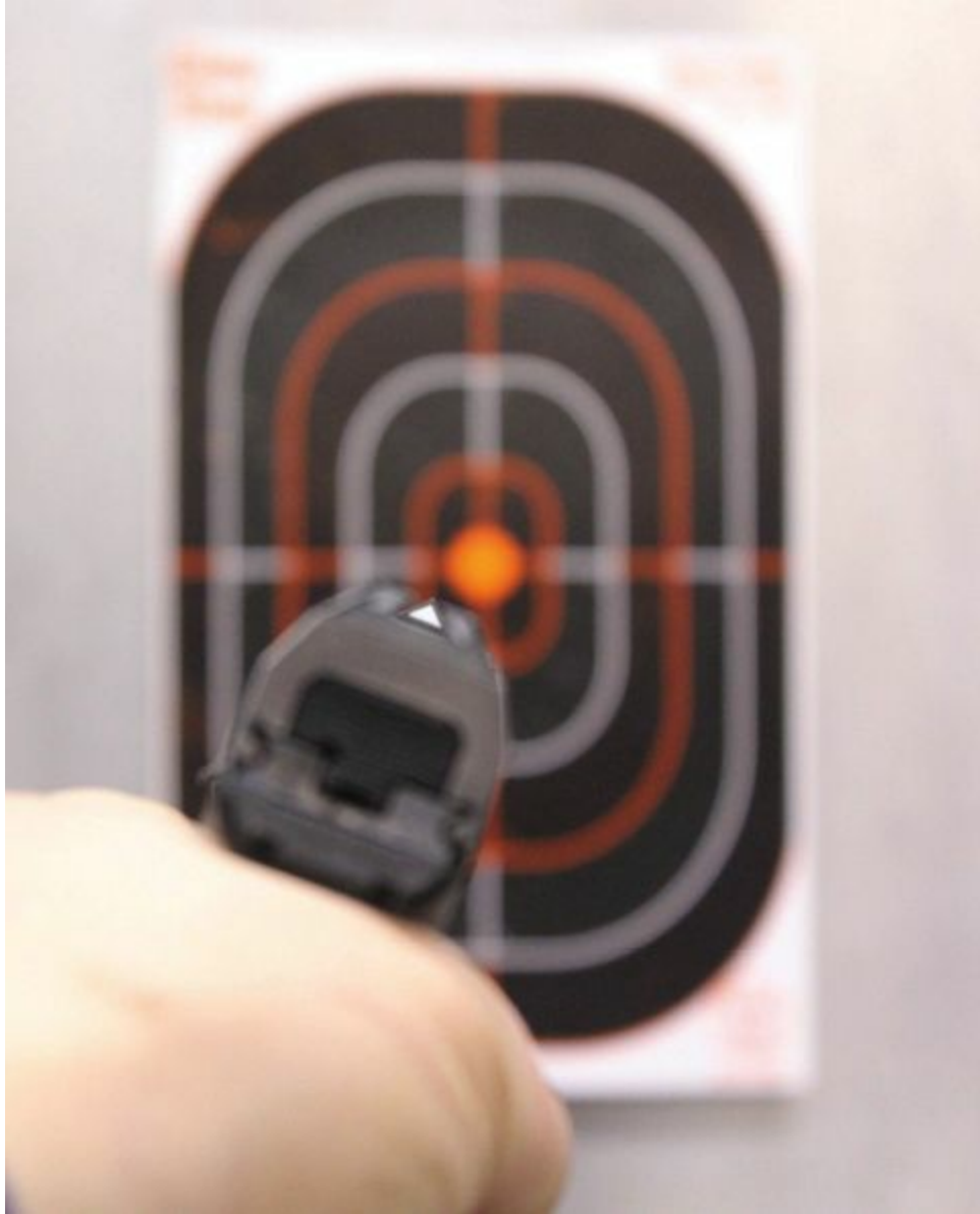
Steyr pistol sights with pyramid front sight and angled line rear.
