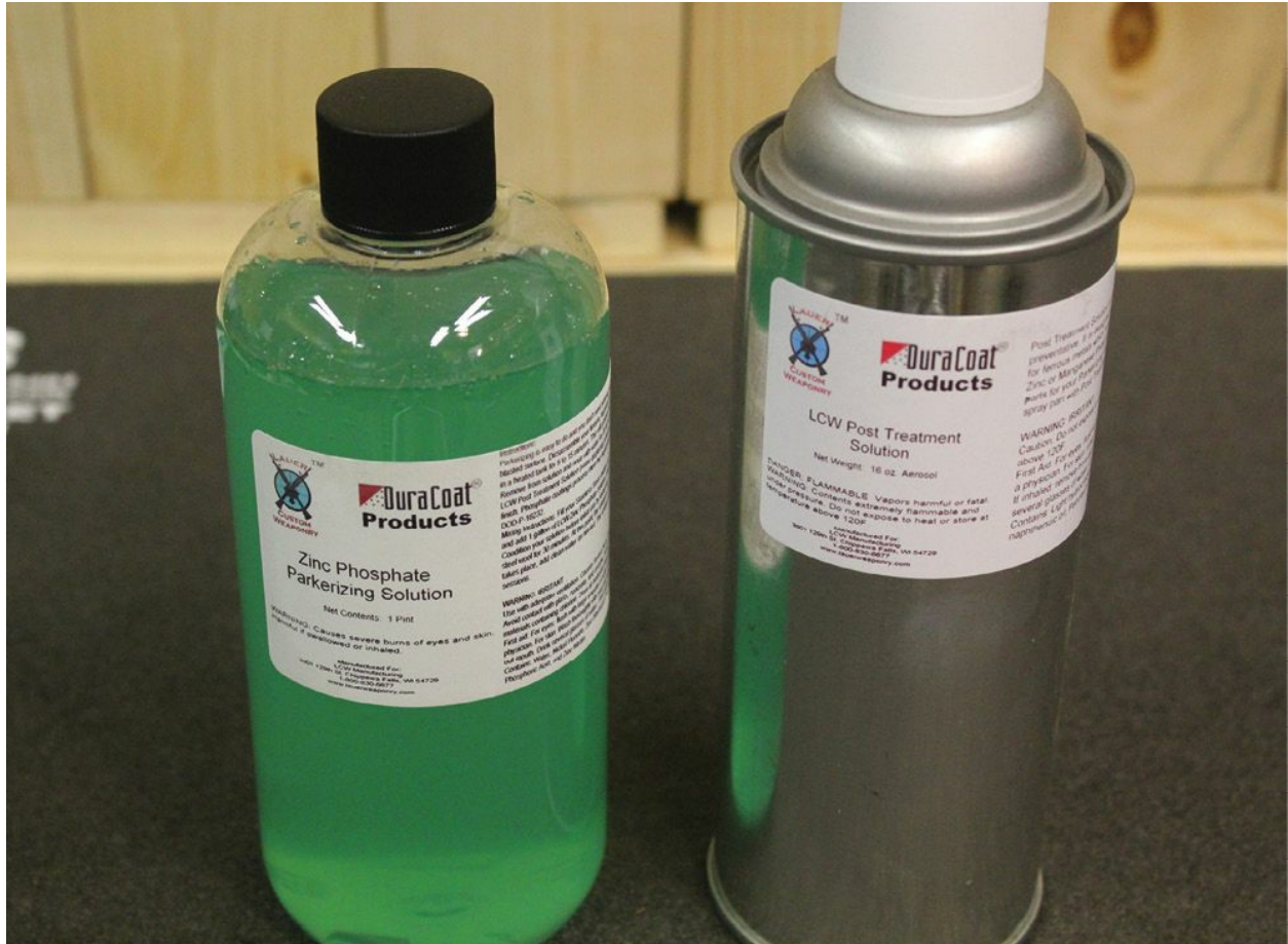
The Lauer Custom Weaponry zinc parkerizing kit. Parkerizing can be done on a standard kitchen oventop.
