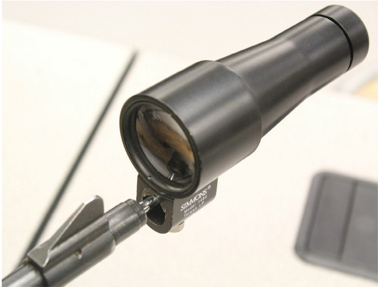
An arbor mounted optical boresighter set up in a Mini-14 rifle. It is not adjustable for height without an extension.
