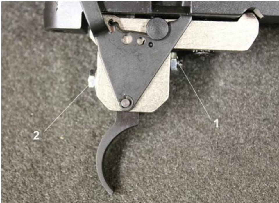
The Howa 1500 trigger. 1 is the weight adjustment with lock nut. 2 is the sear engagement with lock nut. Overtravel is fixed.
