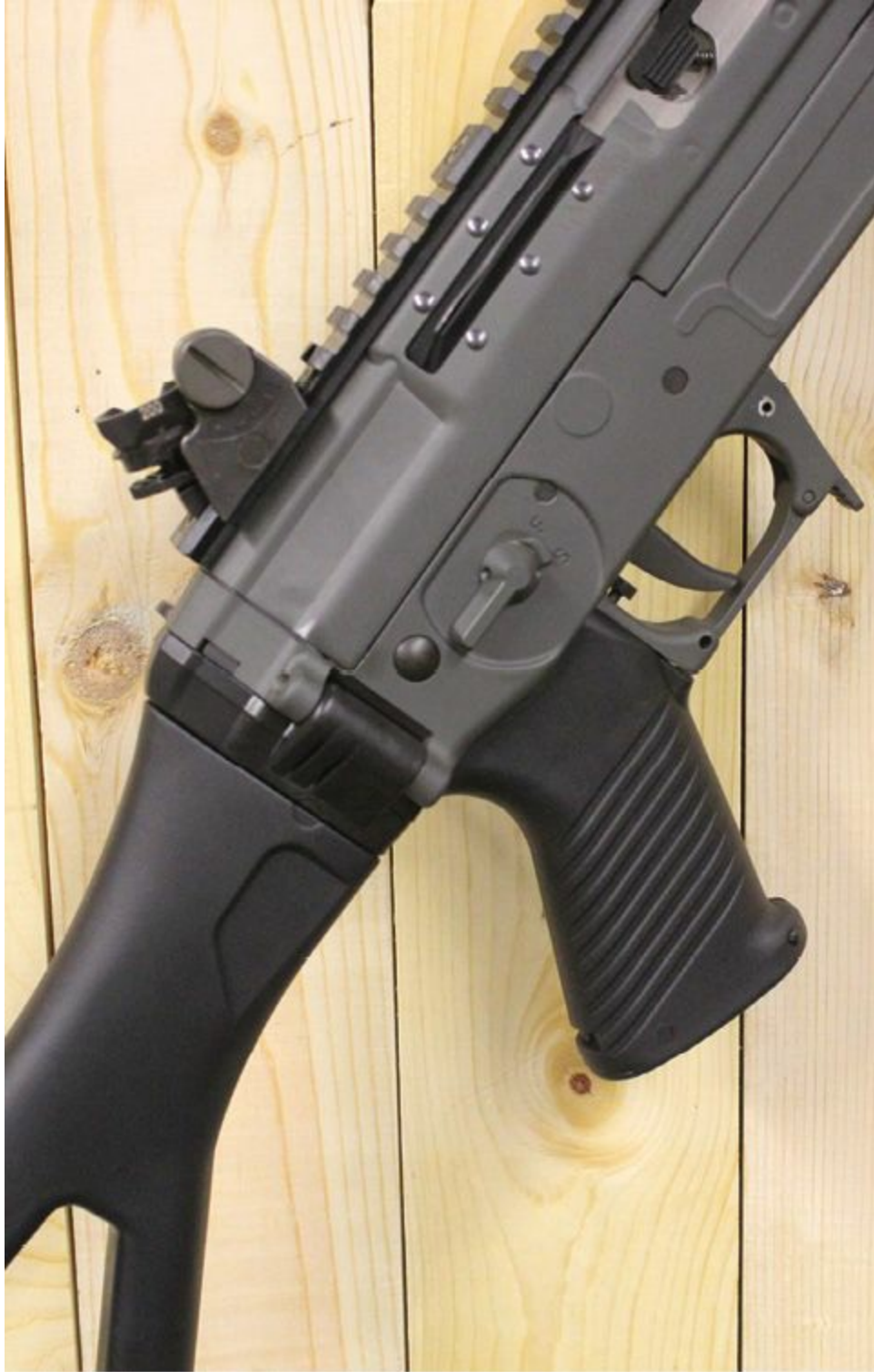
A protruding pistol grip typifies the modern sporting rifle. The pistol grip, stock, and forend or handguard are almost always separate pieces.
