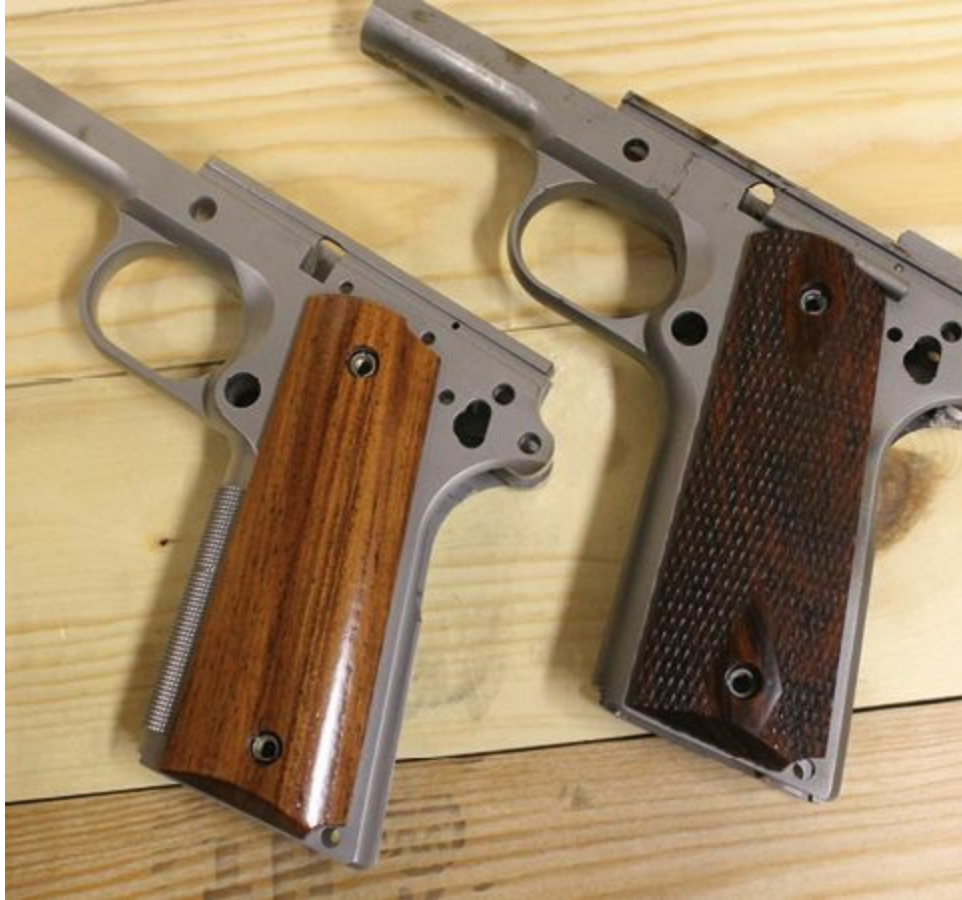
Smooth rosewood grip panel on the left, and checkered cocobolo grip panel on the right. The exotic woods have interesting grain patterns and colors.
