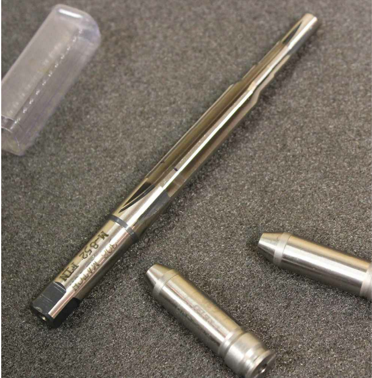
Manson M-852 chamber reamer with .308 headspace gauges.
