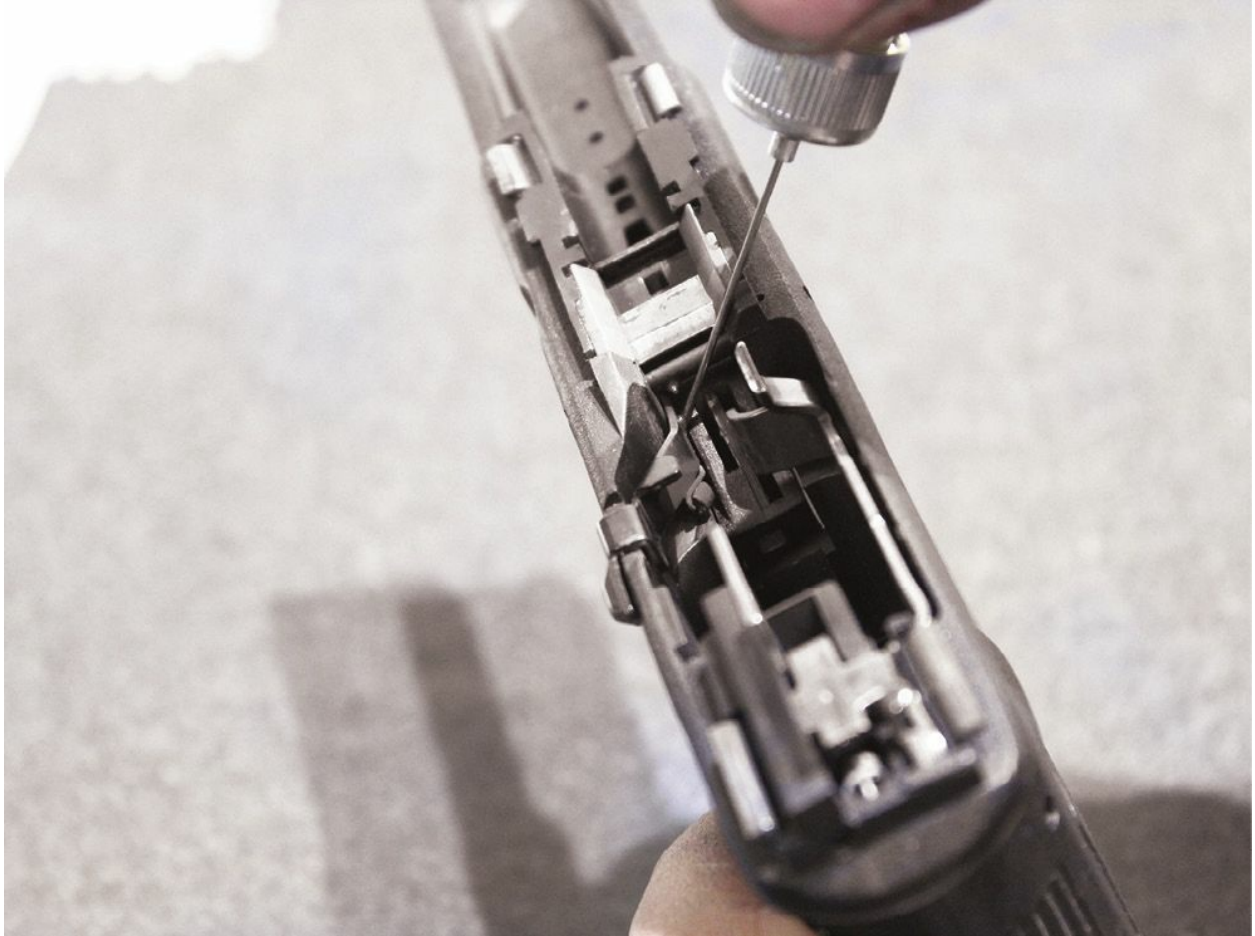
Oil here on the trigger pin. Just a drop or two.
