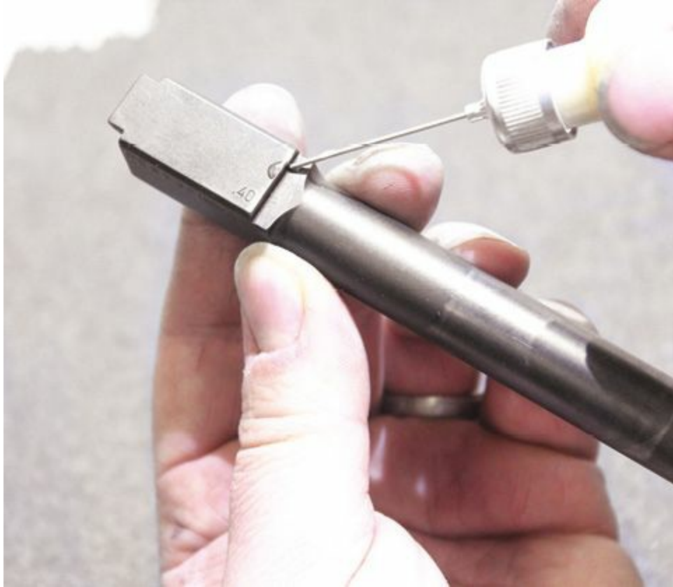
Oil here in front of the barrel hood.
