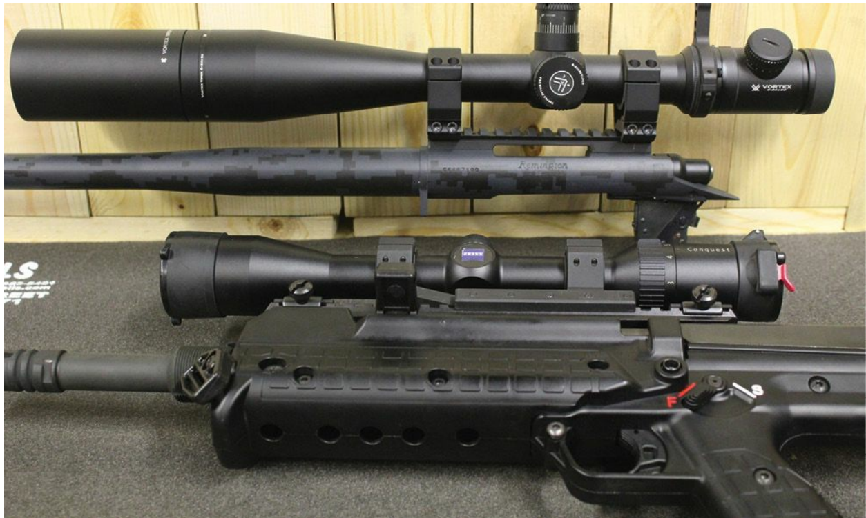
A newer 30mm tubed long range Vortex riflescope with illumination and front focal plane reticle, next to the plain old standard Zeiss.
