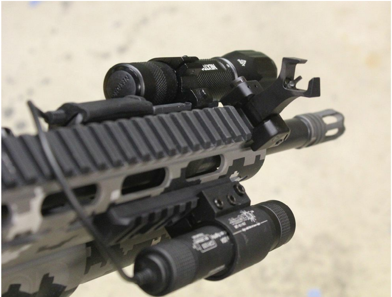
Those tiny hex wrenches are for adjusting the direction of the laser, so that it can be zeroed.
