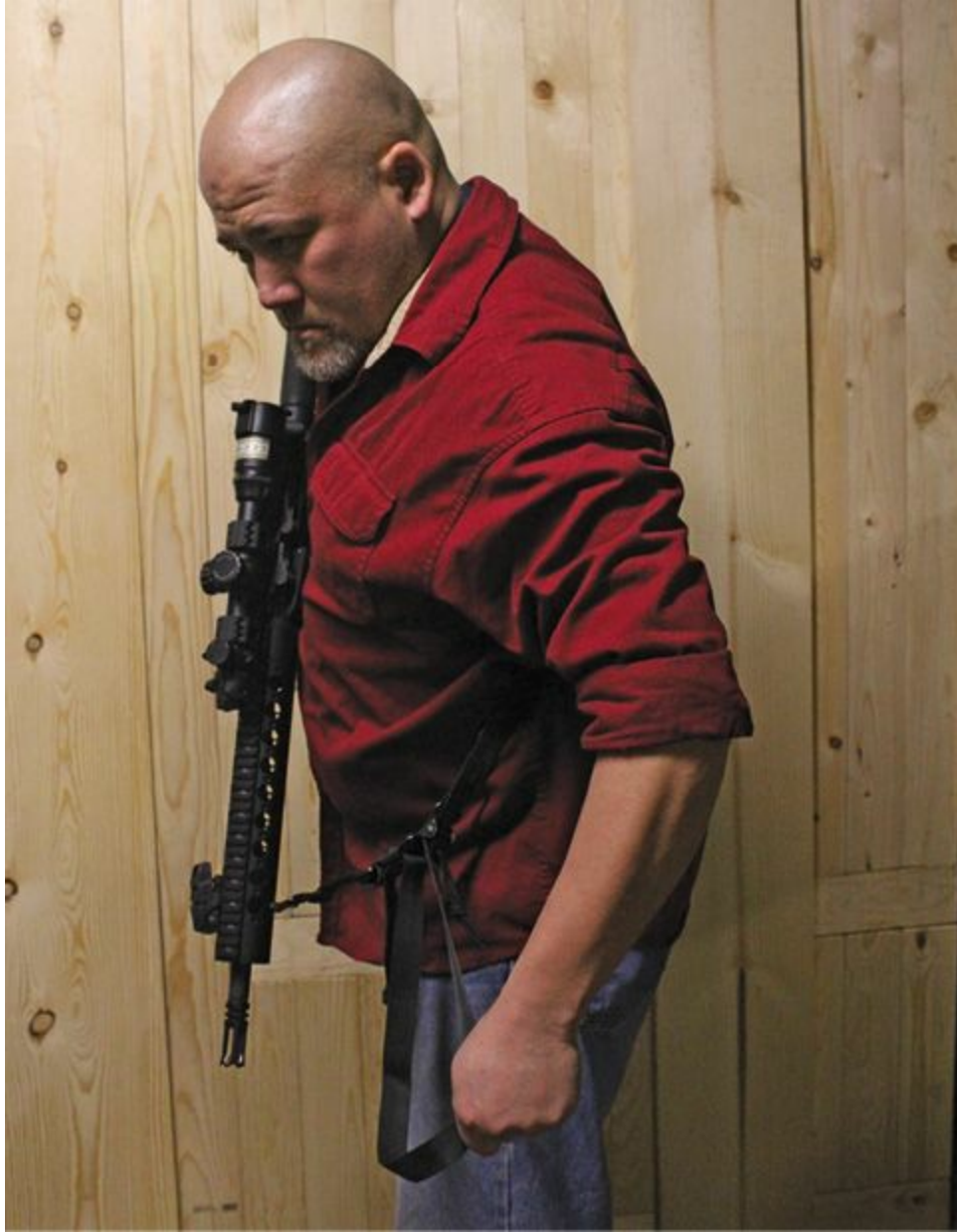
Pulling this strap on the Viking Tactics sling tightens the rifle to your chest.
