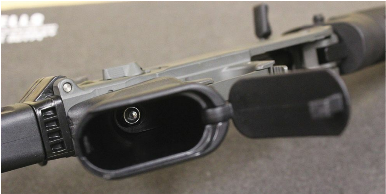
AR grips are held by a simple \frac{1}{4} -28 screw.
