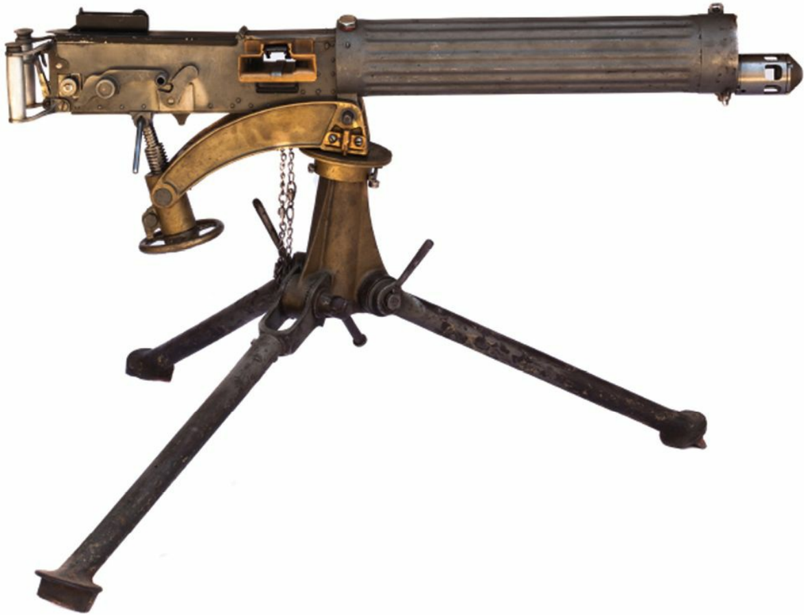
Belt fed Vickers machinegun, cooled by water in the large jacket surrounding the barrel.
