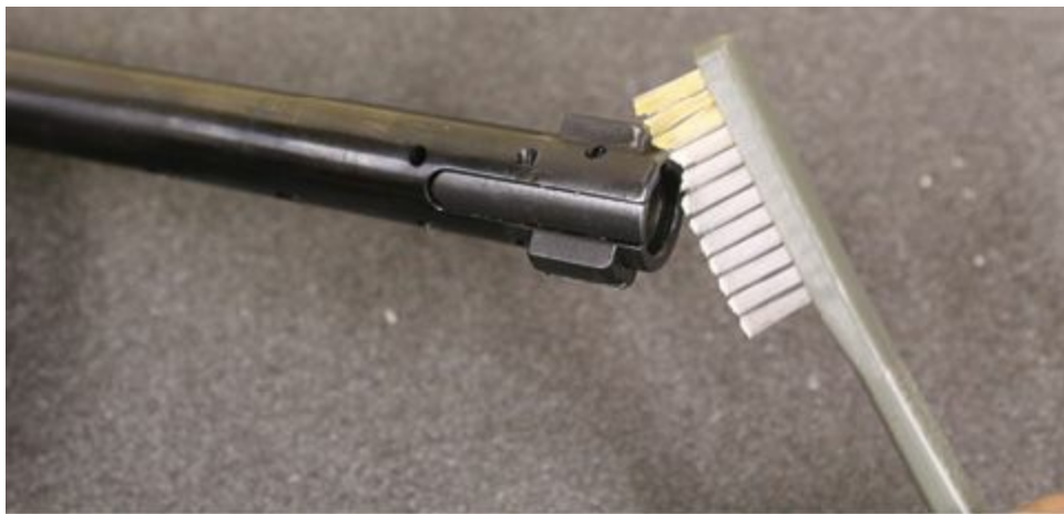
Use a brush to clean off the bolt.
