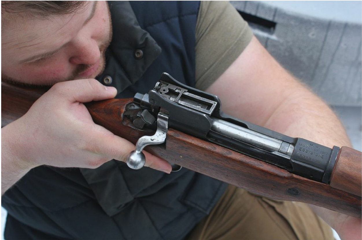
The Model 1917 Enfield had extremely rugged, well-guarded aperture sights.
