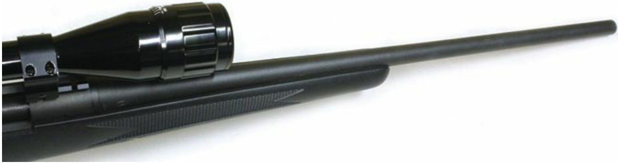
This 700 ADL had front and rear sights, but the rear sight was removed to accommodate a low mounted scope.
