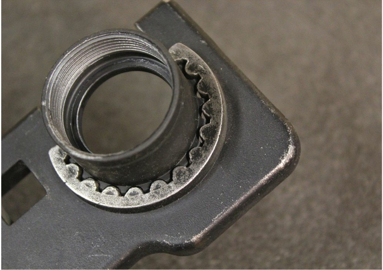
A standard AR barrel nut shown without the delta spring ring. The teeth fit into the slots in the wrench.
