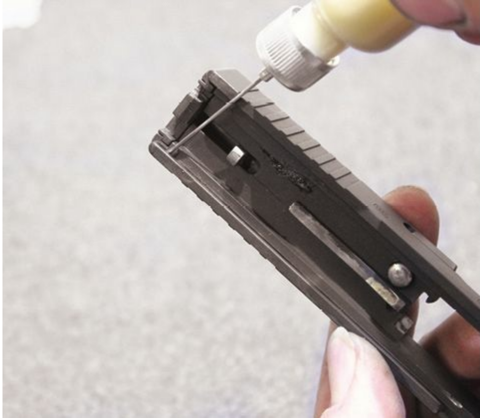
Oil here on the slide rails.
