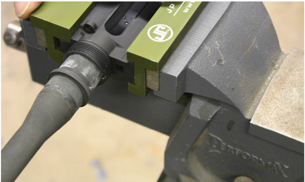
Pulling the old barrel out.
