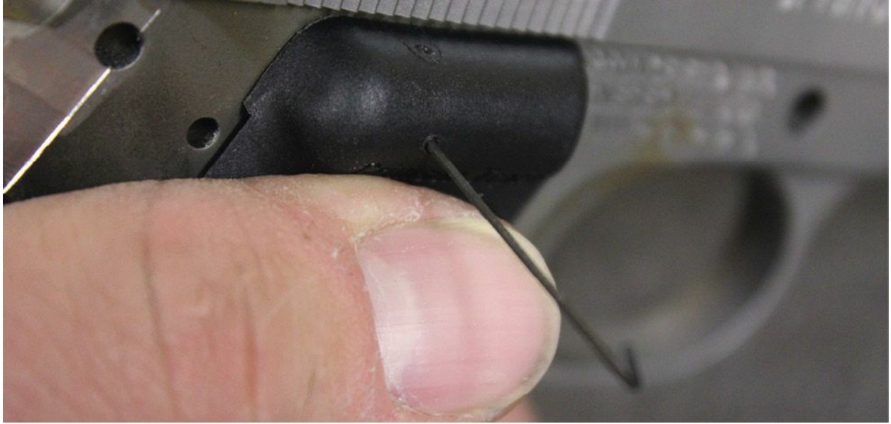
Those tiny hex wrenches are for adjusting the direction of the laser, so that it can be zeroed.
