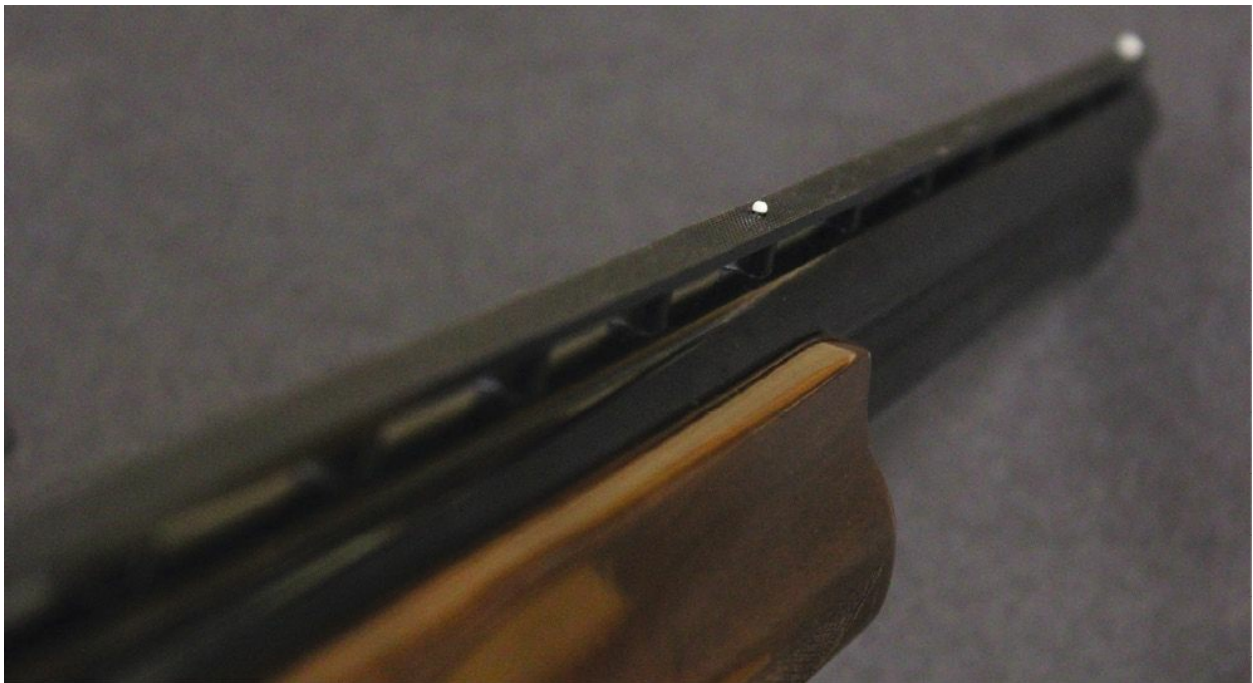
Brass is still the most common component for mid-rib beads. As the name suggests, they are placed halfway down the barrel.
