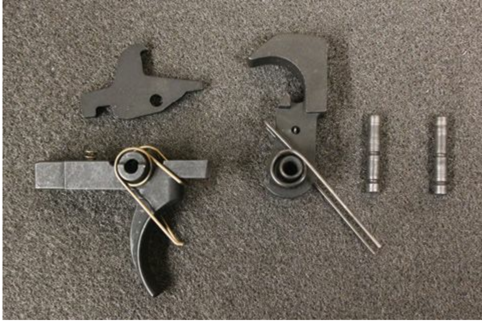
This is the standard trigger, hammer, disconnector of an AR-15 that comes in most factory rifles.
