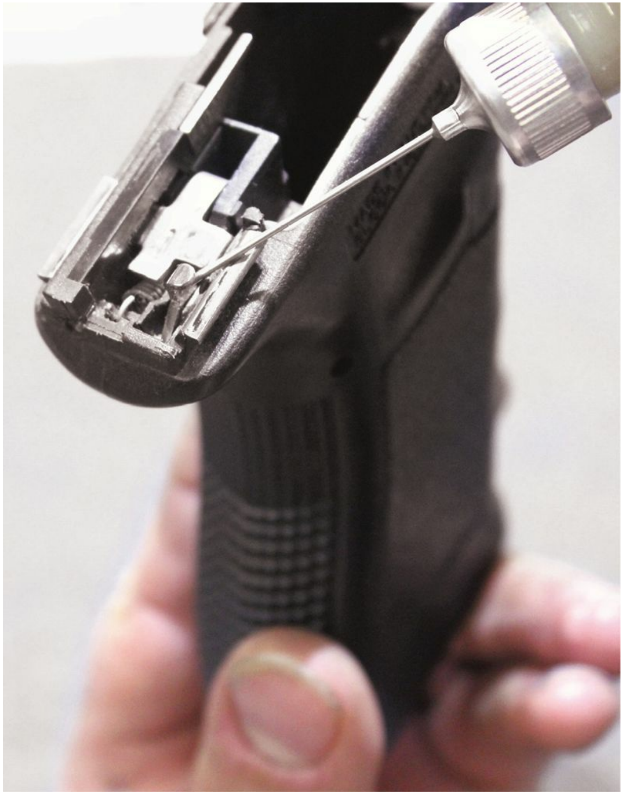
Oil here on the connector bar/trigger bar interface.
