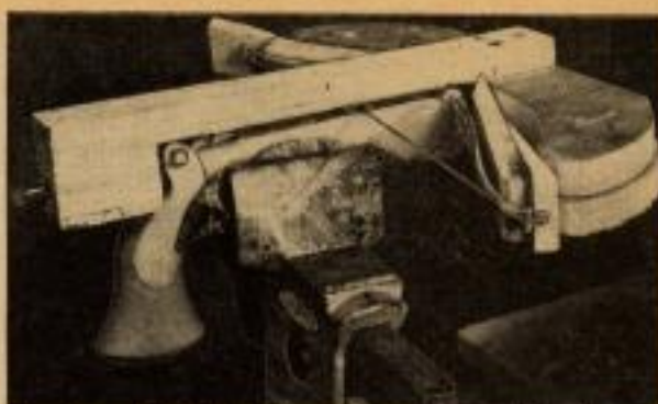
Fig. 4. Turning belt in butt end of this scrap-wood jig bends the bow until free end of the bowstring loop slips into its neck.
