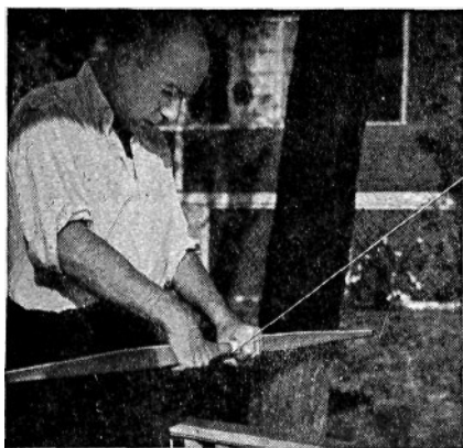
Wrapping the grip with crab line. The line is clove-hitched to a convenient nail or hook
