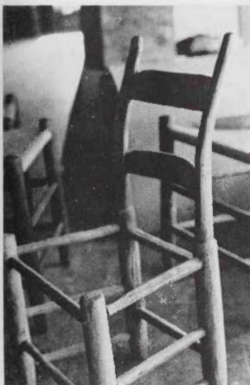
The slats and posts of this mule-ear chair were bent by boiling them. They then were placed in frames to dry.
