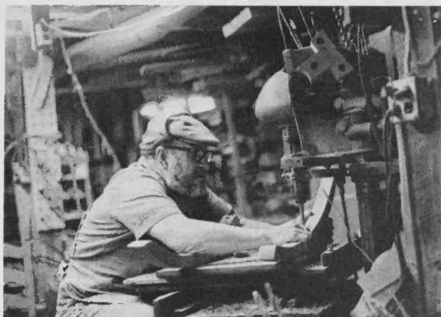
Max drills holes into the rockers for the two posts. A block on his drill press keeps him from drilling through the rockers.
