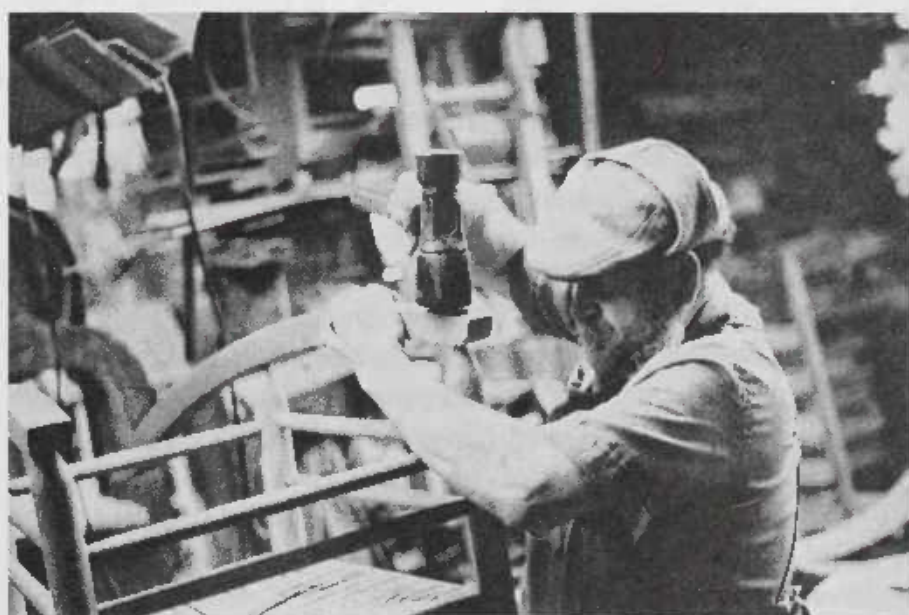
Having glued the post, he drives the rockers on with a mallet.
