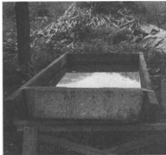
PLATE 18 The sorghum pan is made by nailing together four two-by-eights covered with a sheet of tin to form the bottom and sides.
