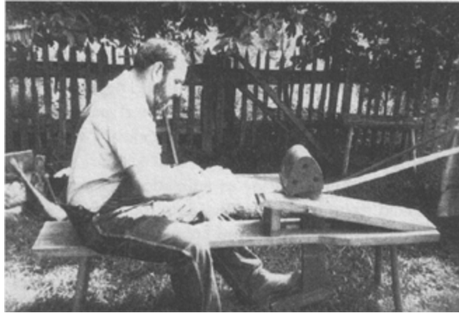
PLATE 117 Connie Carlton working on a pitchfork with his shaving horse and drawknife
