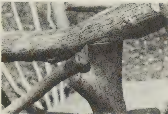
PLATE 125 As you can see from this photo, a notch is made in the arm of the chair to fit over the front post.
