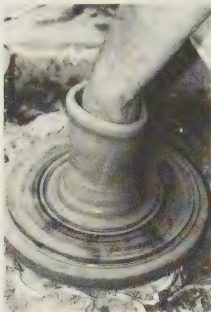
PLATE 81 Performing a knuckle draw to form the shape of the jug
