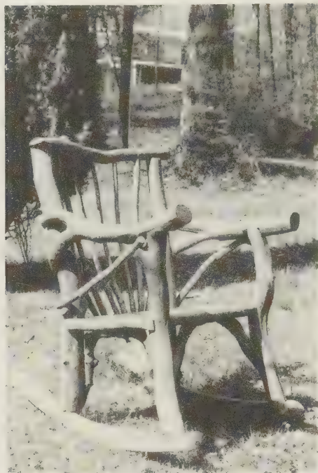
PLATE 127 Note how Kenny used crooked and forked wood for the arm to give more support to the chair.
