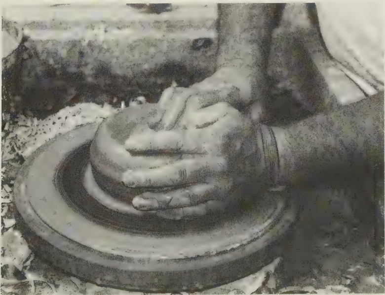
PLATE 80 Centering the clay on the head block while pushing down on the inside
