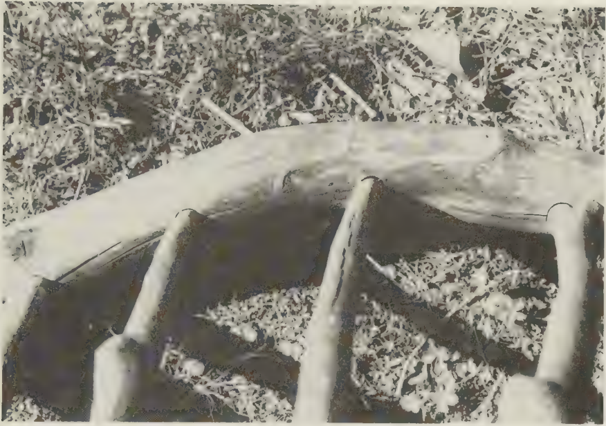
PLATE 129 Holes are drilled into the top for back slats to fit into.
