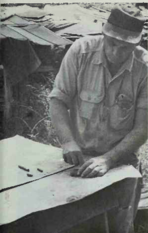
PLATE 103 Before the firing, Lanier made up a set of cones. "I make them out of the glaze and set them in the bottom of the chimney. That's to tell when it's done. They melt at about 2300° F. I roll them out after the glaze has dried out enough to roll."
