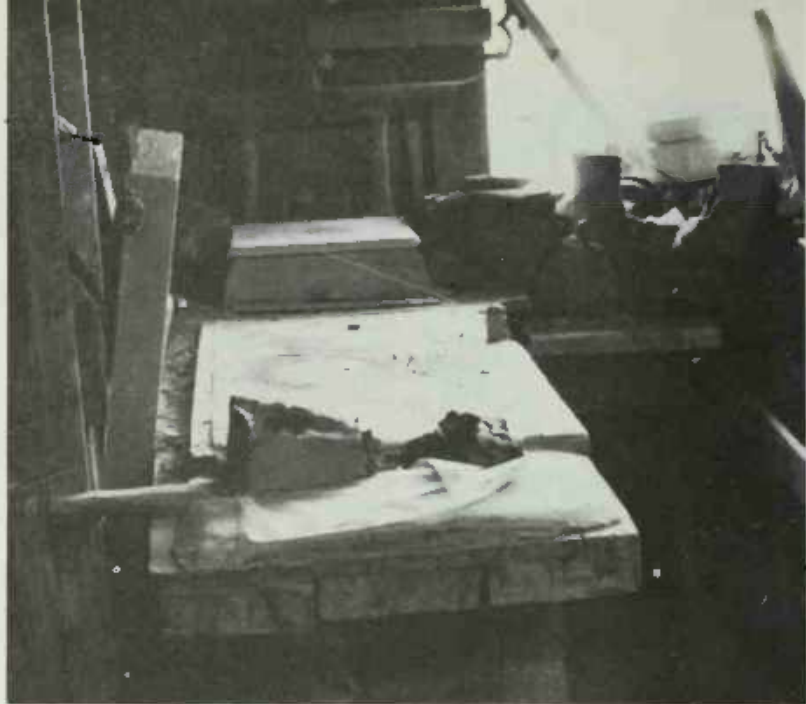
PLATE 434 The ball board, with scales for weighing balls of clay in the background. There is a piece of wire tightly strung from the wall to the front edge of the counter over the flat piece of plaster material where the clay is worked. A ball of clay is first weighed for the amount needed for the specific piece to be made. It is pounded onto the flat surface, then cut in half by the wire and pounded together again. This is done several times to ensure that all the air is out of the clay.
