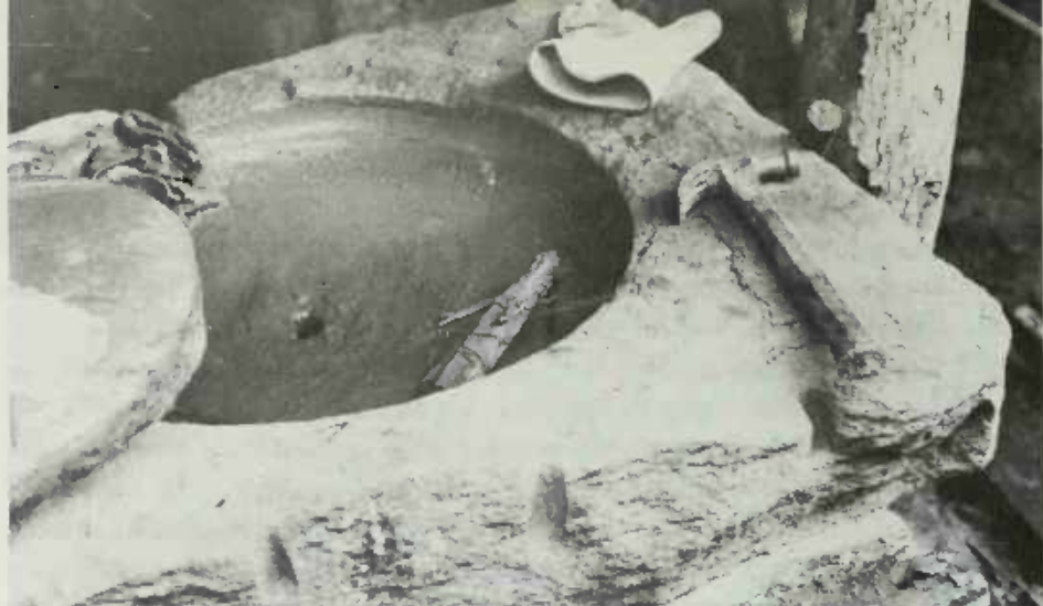
PLATE 68 The glaze mill, still in use in the late sixties when these photographs were taken, is no longer usable as the action of the top rock turning in the bed stone has now worn through the bed stone itself. When first put into use, the top surface of the bed stone was completely flat. Lanier: "That thing wore out [concave] that way. When that [glaze mill] was first started, this [top] rock was just set right flat down on the other one and clay packed around it to hold [the glaze] in. And then the top rock just wore its way through the other one."
