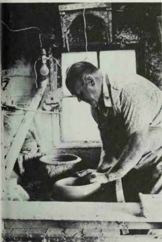
PLATE 252 Then, grasping the edges with his hands, he begins to bring up the jar's top.
