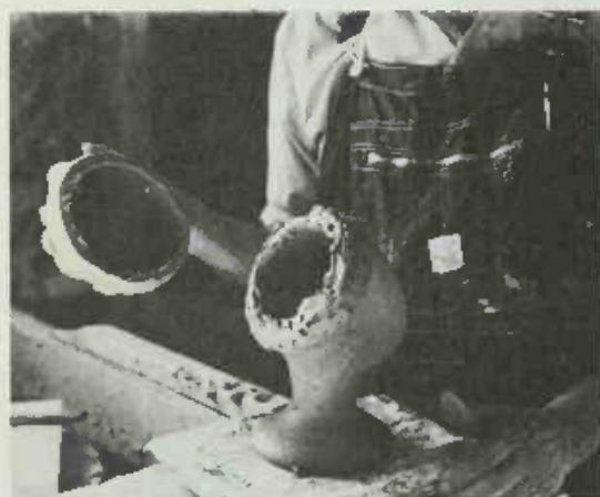
PLATE 189 . . . applies a \frac{1}{8} " to \frac{1}{4} " layer of glue to the rear body part . . .
