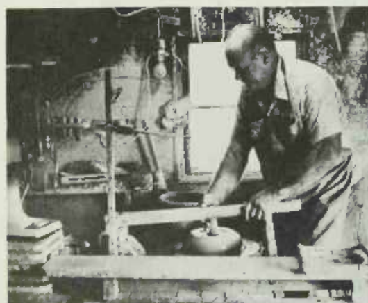
PLATE 249 Pumping with his left foot, Burlon centers the ball of clay on the wheel and lowers the ball opener to open it up for turning.
