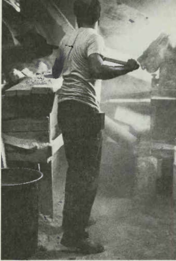
PLATE 425 Charlie Brown shoveling the dried clay into the dry pan to be crushed. There is also an old hammer mill in the shop that was once used to crush the clay. It operated like an old corn-grinding mill. Charlie told us it is no longer used because his grandfather thought it was too dangerous, and so built the dry pan.
