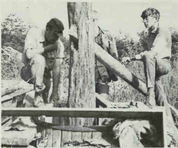
PLATE 50 The wooden beam the mule is harnessed to when the mill is in operation is visible here. Lanier's right foot rests on one of two wooden counters on which the finished clay is blocked up before being carried into the shop. As the mule turns the mill, Lanier says, "You can't imagine all the squeaky noises and everything. It sounds like old screaming doors on old haunted buildings. Just real creepy. Real ghostly-like."
