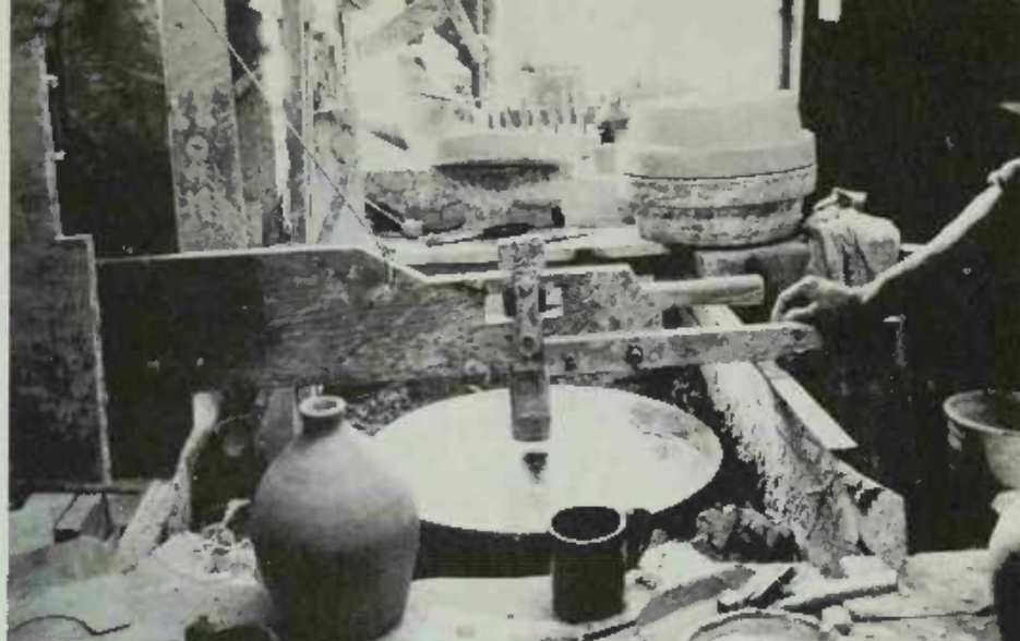
PLATE 418 Demonstration of how a ball opener works and then the pot being brought on up by hand.
