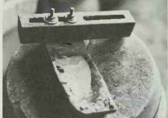
PLATE 449 A close-up view of one of the knives, fitted into the handle that is fitted into the steel structure (see Plates 444 and 445).
