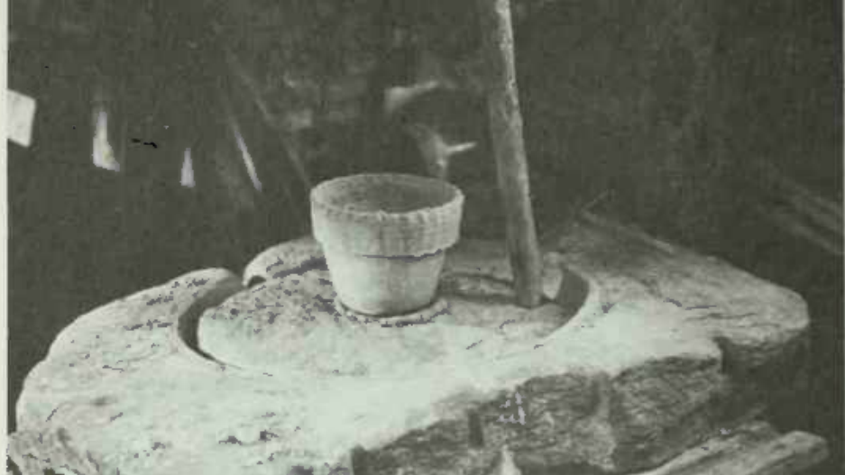
PLATE 72 To grind, the top rock was set in place and a flowerpot with the bottom knocked out of it was set over the central hole in the top rock. With clay packed around its base, the flowerpot acted as a funnel for the raw ingredients of the glaze to be poured into. Those ingredients usually included settlings, ashes, sand, and/or glass in a water base. If glass, it would have been pulverized already ("We beat the glass up with a long iron rod and mostly main strength and awkwardness"), but between the grinding surfaces of the two rocks it would be powdered even further.
