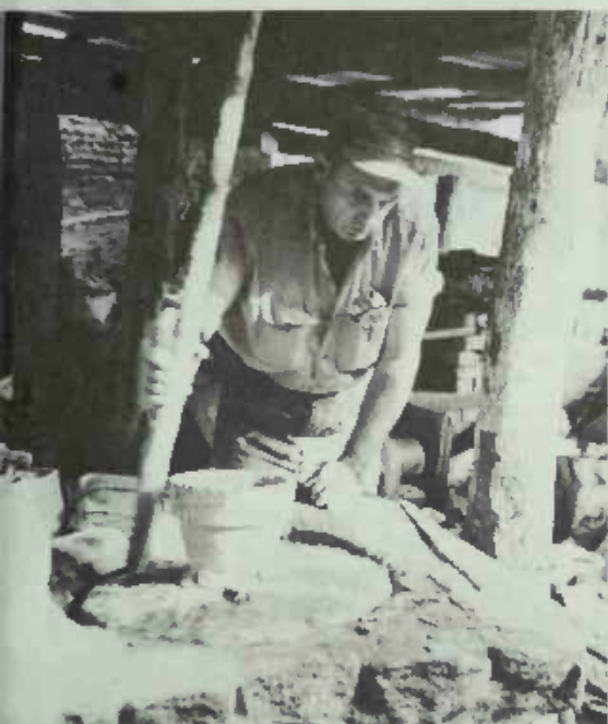
PLATE 75 . . . and grasp the wooden pole and begin to spin the top rock. The glaze would flow out the groove cut in the bottom rock "in little squirts." If the rocks were too far apart, "It wouldn't be grinding the stuff that went through it. When you feel of the glaze, you can tell whether it's ground or not. If it's coming out too coarse, why then you have to let the top rock down. Just ease the wedge out a little bit [from under the beam the iron rod rests on at the bottom] and take another iron pin or something—whatever you want—and chug down on the end of that thing in there and that would let it down a little. And a lot of times, you wouldn't have to mess with the wedge. Just [making a tapping motion] tap it down."
