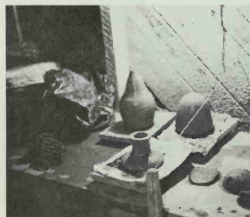
PLATE 168 The three main pieces are allowed to dry overnight to become firm enough that they can hold their shapes as they support each other's weight.
