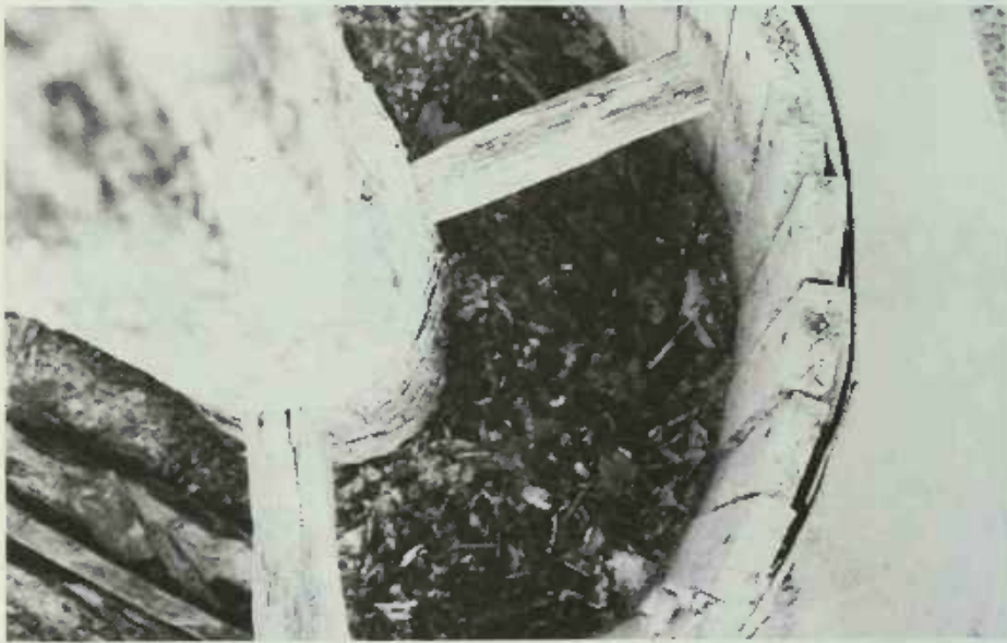
PLATE 51 Looking down into the mill, half-filled with leaves, two of the nine oak pegs are visible. There are three rows of three pegs each, staggered so that no two run the same course. "Those pegs are mostly flat on the bottom and rounded off on top and that gives the clay upward lift. When them things go around, they leave [an open] place behind them, and the clay rolls back into that open spot and then another peg comes along and cuts it again and keeps it rotating all the time. [You have to be careful because] you can get too many of them things in there. You can put so many pegs in there that it'll choke itself. It'll just pick up all the clay and just slide it around and around in one lump. Now that's what happened [in the motor-driven mill with a metal shaft and blades Lanier had built to replace the wooden mill], and me trying to get that old boy not to do it that way. I tried to explain him how to do it, but he can only do things his way. You can't tell him how you want anything done or you get him all outa sorts and he can't do it at all. But he put too many teeth in it, and I had to take a hacksaw and saw some of them out."
