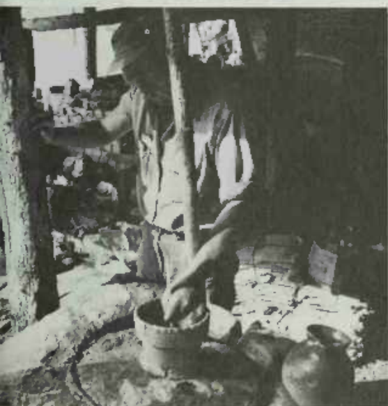
PLATE 76 From time to time the glaze would gum up in the bottom of the funnel and Lanier would have to take a stick and stir it up to keep it flowing.
