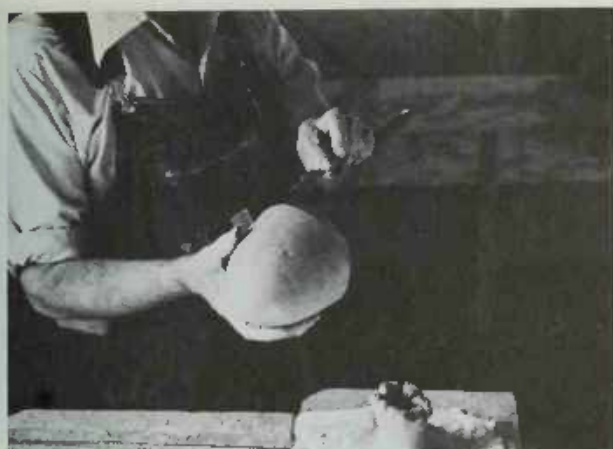
PLATE 184 Taking the rear part of the body, he tapers both the inside and outside bottom edges so there will be more surface area for the glue to adhere to . . .
