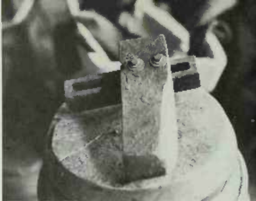
PLATE 450 The reverse side of the jigger knife.
