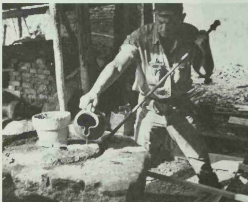
PLATE 73 "You see that iron rod I've got there? I've got that top rock prized up and I'm pouring water under it to unstick it. After it's used, there's always some glaze that's left in there, you know, and it dries out and sticks and you have to loosen it before you can grind again."
