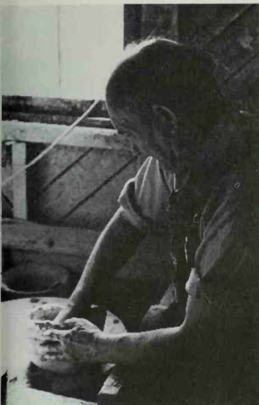
PLATE 169 The next day, Edwin mixes up a double handful of raw clay with enough water to make a sticky clay "mush"—the glue that will hold the pieces together.
