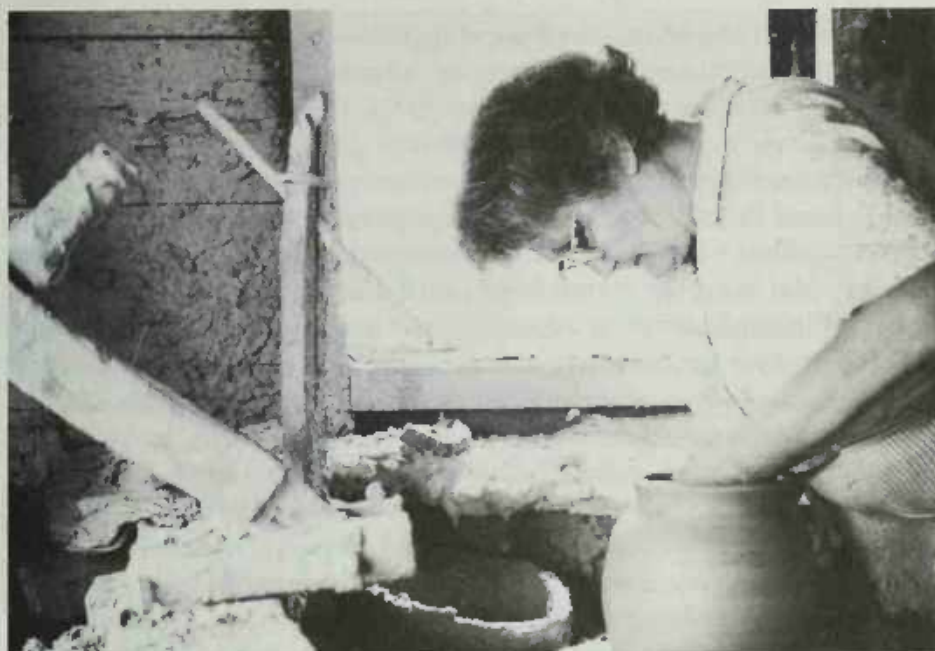
PLATE 65 A photograph of Aric taken at the same time shows the simple but efficient height gauge she and Lanier employed. When in use, to indicate the height a gallon piece should be, the pointer was set at twelve inches above the surface of the wheel, and the piece was turned to the pointer's tip.
