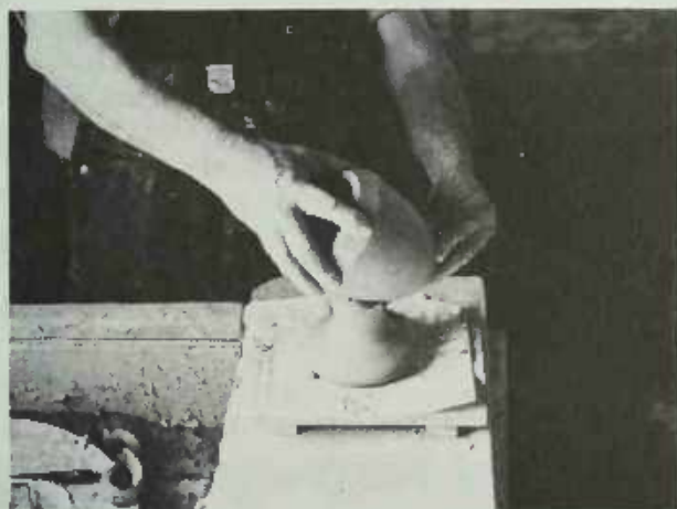
PLATE 185 . . . and presses the piece firmly down onto its base.
