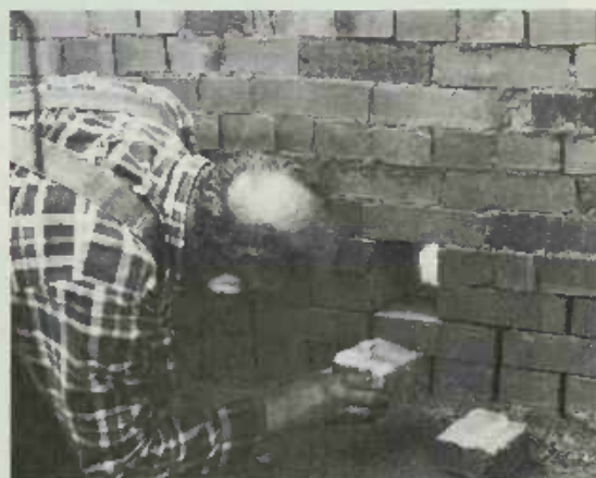
PLATE 220 During the final phase of firing, Edwin goes to the chimney end, removes two loose half bricks in the chimney wall, and checks to see whether or not the ware is completely fired.
