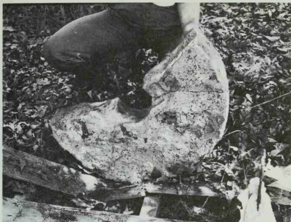
PLATE 367 Chester Hewell: "[That mill wheel] is what they used to grind the glass glaze with. They had an old thing to beat the glass up to a fine powder and then they ran it through the stone, like you were grinding cornmeal. They would run the whole mixture through there. It served as a ball mill. A ball mill is a thing that tumbles and mixes different types of clay and glazes together to make it a body of its own."
