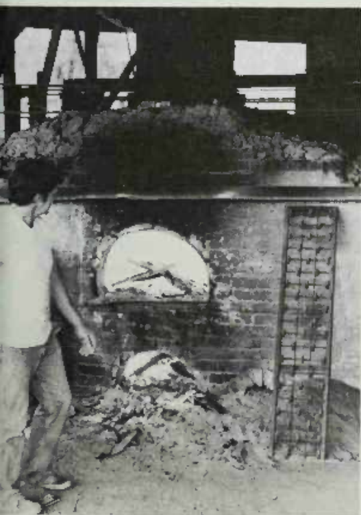
PLATE 347 The kiln being fired. This view of the wood-burning kiln shows the firebox. The twin chimneys are at the other end of the kiln, creating drafts through the kiln and over the ware. Many times ware nearest the ceiling of the kiln will be scorched because of excessive heat. For each firing, therefore, already scorched pots are stacked into the kiln in those places most vulnerable to too-high temperatures.
