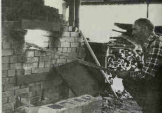
PLATE 215 Edwin fires with pine slabs. A portion of the loading door is bricked up during burning, leaving a hole through which he shoves the slabs. The metal plate resting against the kiln covers the hole when wood is not being added.
