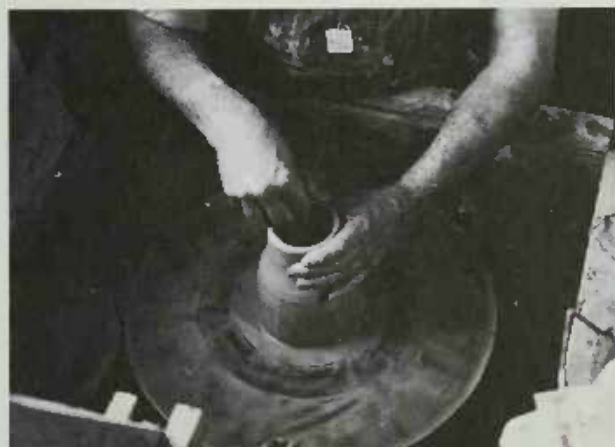
PLATE 157 He then draws the ring up into a jarlike shape . . .
