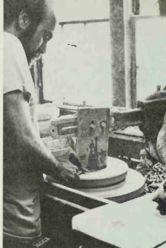
PLATE 444 Charlie at the jigger wheel, demonstrating how a jigger "knife" compresses the clay into the mold. He trims off excess clay before he removes the knife and sets the mold on a shelf to dry.
