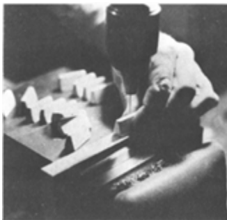
ILLUSTRATION 8 Holes are drilled through the center of each piston, and two holes are drilled 1\frac{1}{4} " apart through the handles to attach the pistons to.
