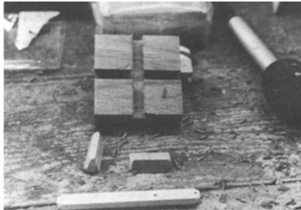
ILLUSTRATION 9 A \frac{3}{8} " dovetail router is used to cut two channels into each 3" square block.
