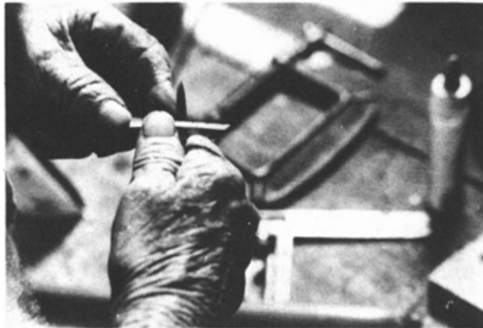
ILLUSTRATION 28 After cutting out the excess stalk between the "strings," he fashions a tiny bridge out of scrap wood.
