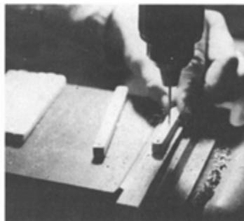
ILLUSTRATION 8 Holes are drilled through the center of each piston, and two holes are drilled 1\frac{1}{4} " apart through the handles to attach the pistons to.
