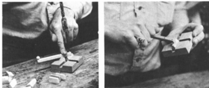
ILLUSTRATION 11 Dave puts wax on the pistons to reduce friction and keep them from binding, then he screws a bead into the handle for ease in turning. Last, he sets the two pistons into the channels cut in the block and attaches the handle. The screws are left loose so the pistons and arm turn freely (left), ILLUSTRATION 12 As the handle is turned, the pistons slide back and forth in their respective channels (right).
