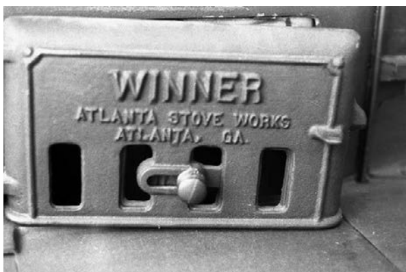
The firebox damper with its vents opened.
