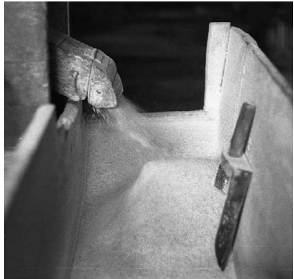
Ground meal shoots into the trough to be bagged and weighed.
