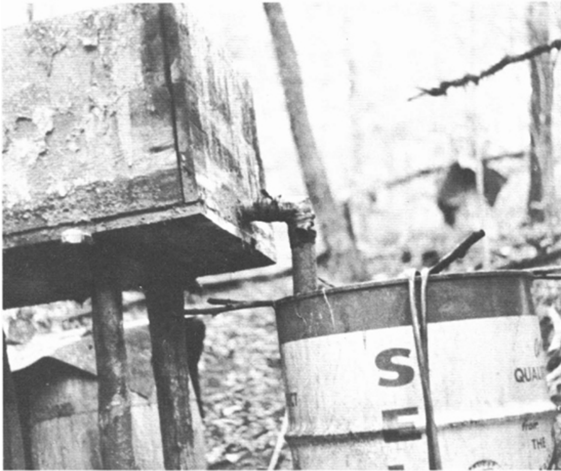
ILLUSTRATION 16 The heater box from the other side, showing the connection between the heater box and the condenser which is mounted in the metal drum.
