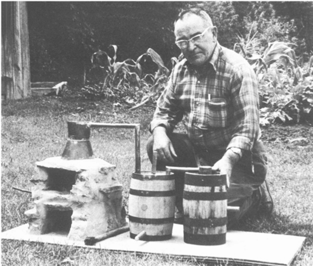
ILLUSTRATION 3 Buck Carver kneels behind a one-gallon still he made for the Foxfire museum. The still is authentic in every detail from the flue of the furnace to the tin-locked
