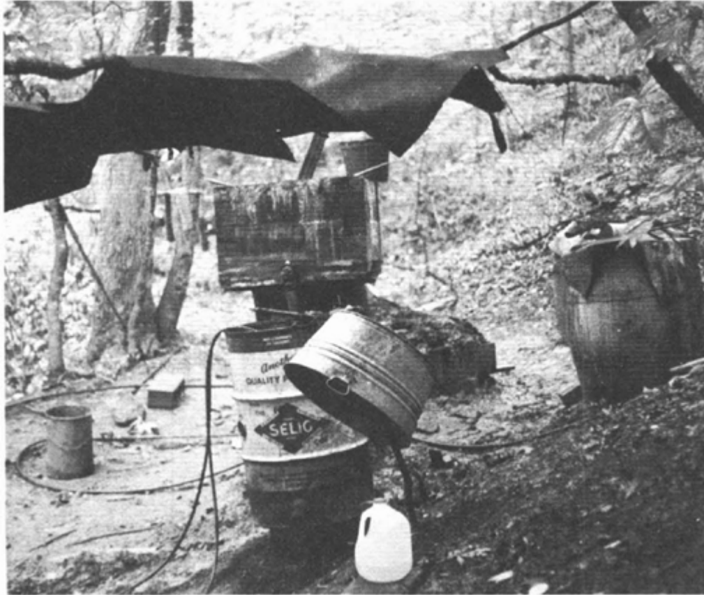
ILLUSTRATION 17 The whole operation from the heater box, condenser end. The wooden barrels on the right are rilled with fermenting mash. The furnace is hidden behind the heater box. The plastic gallon milk jar in the foreground is often used in place of glass jars for the finished product.
