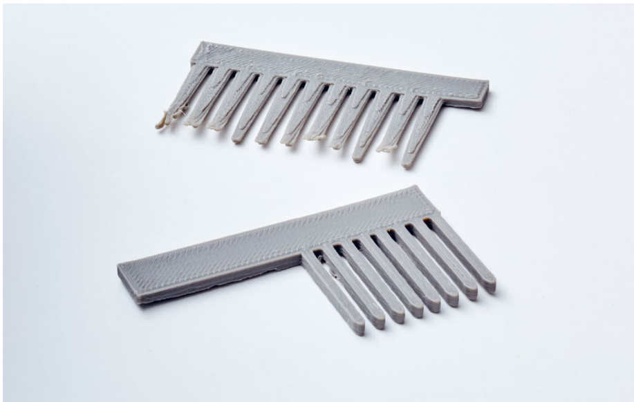
FIG. 5: Check your print to see if its teeth are warped and adjust design as needed.
