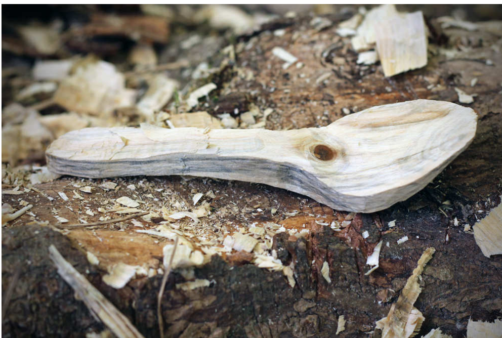
Spoon fully axed out and ready for knife work.
