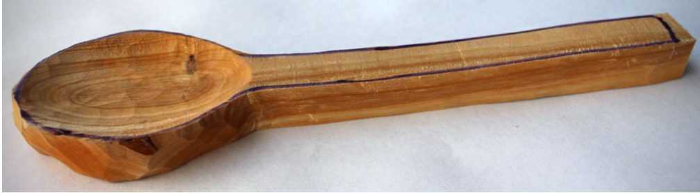
Rough cut blank ready for finishing cuts.
