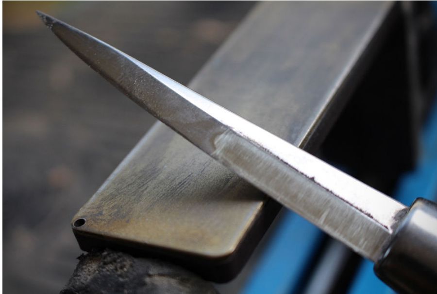
Sharpening ½ way along the length of the blade.
