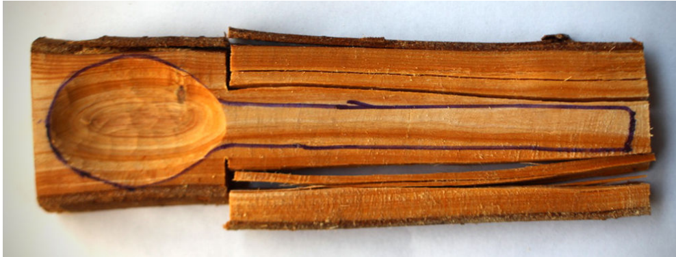
Sections split by batoning with a knife.
