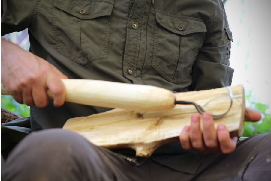
Twca Cam hollowing out the bowl of an eating spoon.
