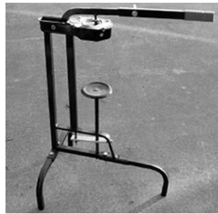
Is your hand and back tired yet from forcing corks into bottles? There is an easier way. A bench and a floor corker work the same way. One can sit on your counter and the other is tall and can be used on the floor. Many of these come from Italy and have a durable design, so you will never have to replace them. You can cork up to about
