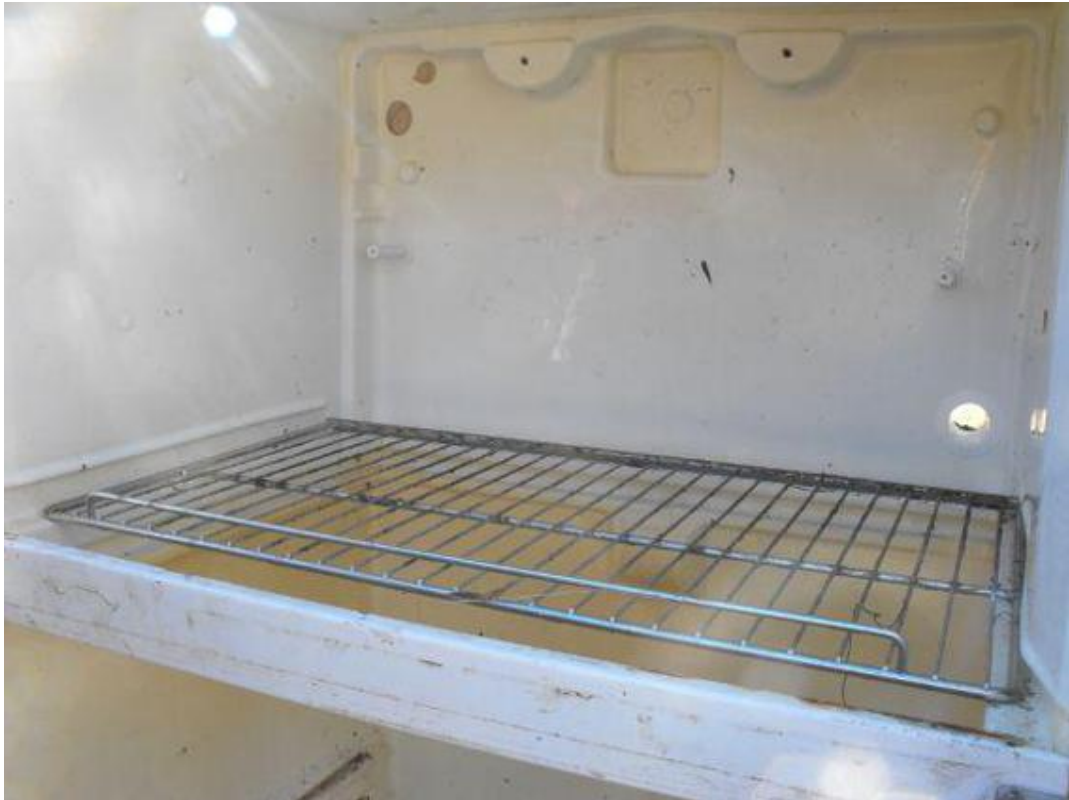
A metal rack divides the freezer and fridge compartments without restricting air flow.
