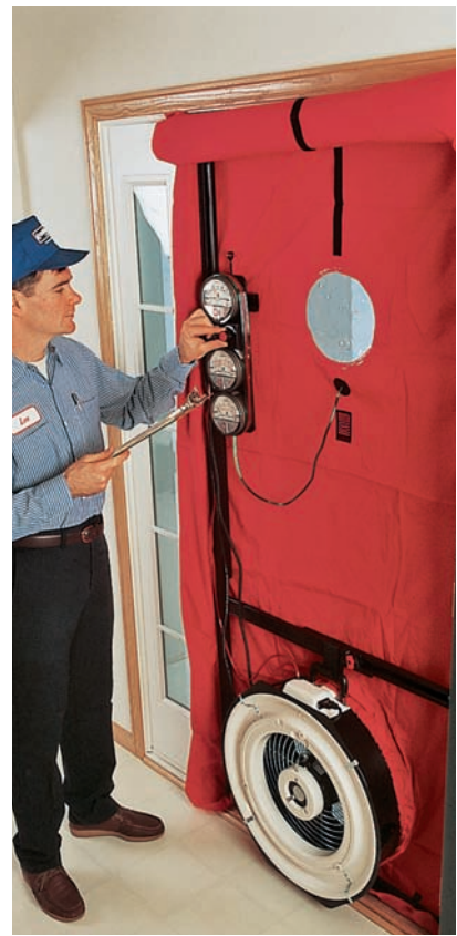
Energy audits done by power companies may use a blower door to measure airflow and detect leaks.
