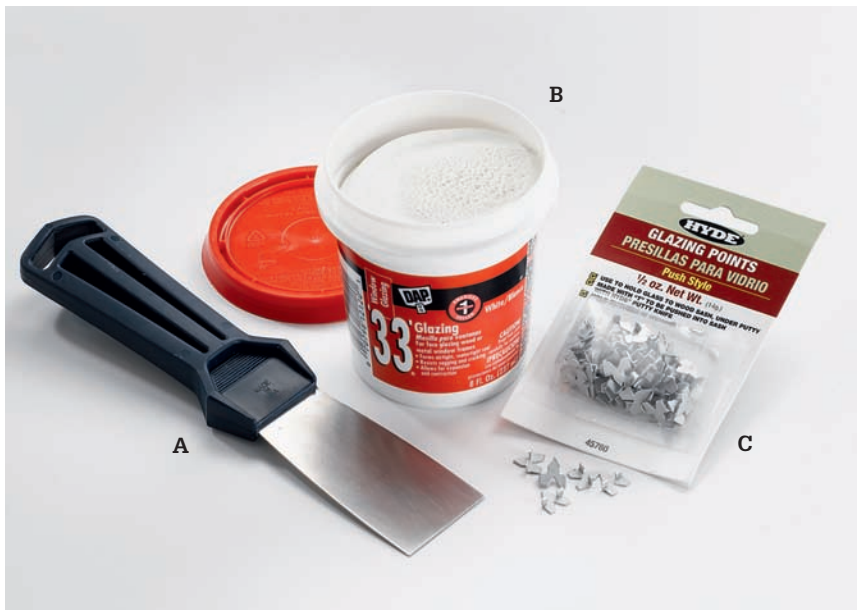
A clean putty knife (A), glazing compound (B,) and a package of glazier's points (C) are essential tools and materials for replacing window glass.
