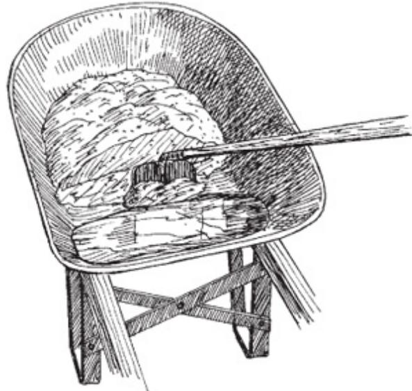
*Mix mortar by “chopping off” slices of dry mixture and working each slice with water.*
