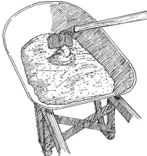
*The concrete mixture should be firm enough to hold stiff peaks.*
