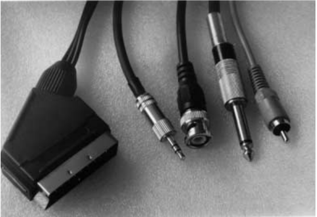
Photo 3.3 Types of cable (l-r): Scart; Mini-jack; BNC; Quarter Inch; Phono/RCA (photo: Paul O'Connor)
